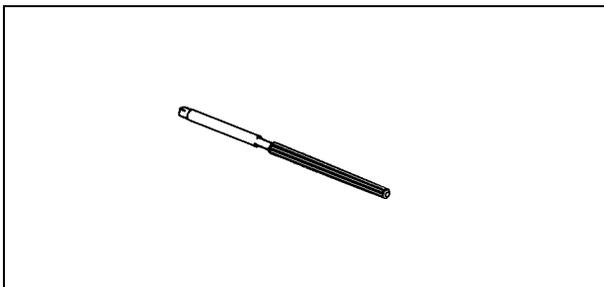
**Valve Seat Cutter,  $45^\circ - \phi 24.5$ :**
