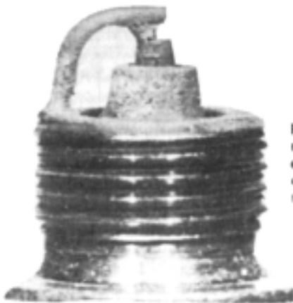
Fig. 5-16. Gap-bridged: a common malady of two-cycle engines, believed to be caused by dust. Wipe the whisker off and restart.
