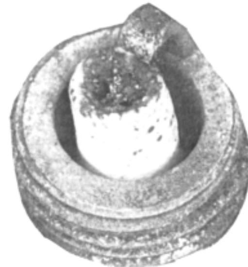
Fig. 5-19. Preignition: melted electrodes and, in most cases, a white insulator. The insulator may be discolored due to a fog of debris in the overworked cylinder. Check for correct heat range, adequate lubrication, and for overadvanced ignition timing. Correct the problem before the engine is put back into service. (Courtesy Champion Spark Plug Co.)
