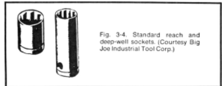
Fig. 3-4. Standard reach and deep-well sockets. (Courtesy Big Joe Industrial Tool Corp.)
