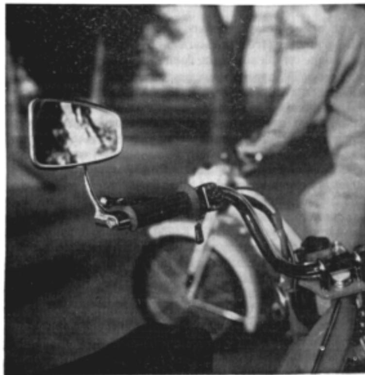
Fig. 1-1. A rearview mirror that meets the new regulations and folds for storage.
