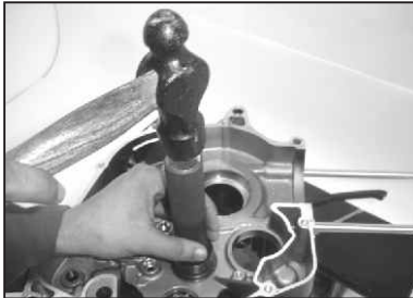
Bearing Driver Set Drawing No.: 37 1030 61 Application : Common bearing driver set for fitting and removing bearings from crankcase.
