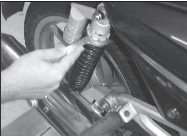
Rear Shock absorber adjuster Drawing No.: 37 00DH 14 Application : For adjusting the notch position of RSA to achieve hard or soft rear suspension
