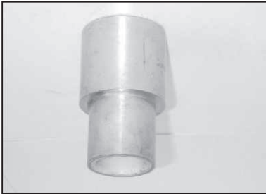
Fork oil seal fitment punch Drawing No.: 37 0040 03 Application : To fit fork oil seal on outer pipe
