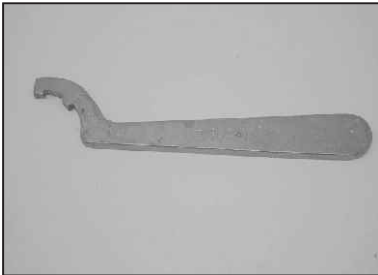
Rear Shock absorber adjuster Drawing No.: 37 00DH 14 Application : For adjusting the notch position of RSA to achieve hard or soft rear suspension
