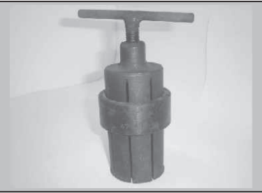
Crankshaft Bearing Extractor Drawing No.: 37 1001 14 Application : To remove bearing from crankshaft
