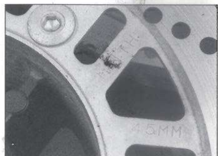
4.4b The minimum allowable thickness is stamped into the disc
