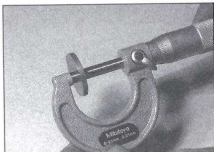
Tappet shims are measured with a micrometer
