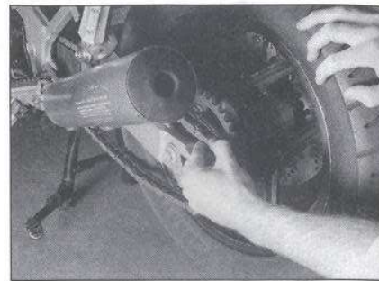
12.6 Push the wheel forward and detach the chain from the sprocket
