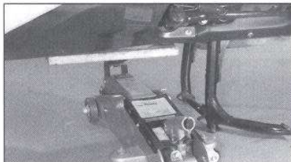
1.4 Always use a block of wood between the engine and jack head when supporting the engine in this way
