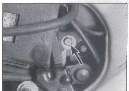
11.8 The right-side mounting bolt for the air filter housing (arrow) is located in front of the igniter unit (A and B models)
