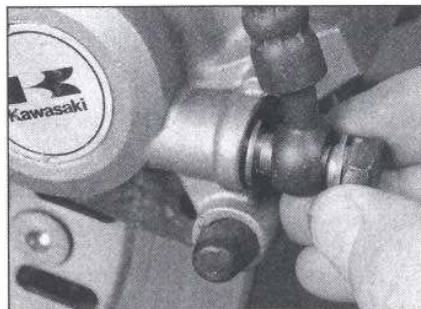
2.3a Unscrew the banjo fitting bolt, ...
