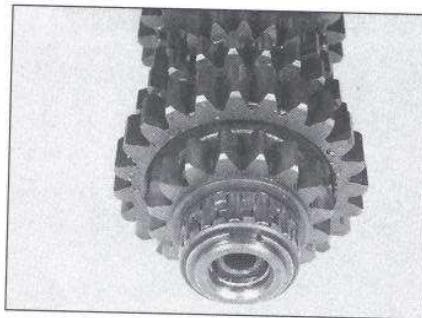
30.2b ... then remove the snap-ring and bearing
