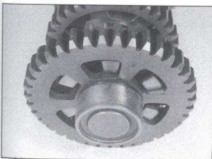
30.14a Slide off the bearing outer race ...
