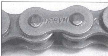
8.10 Typical chain size and type marking
