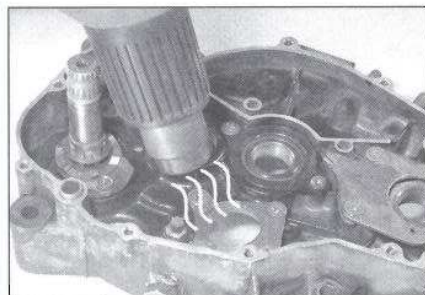
2.15 Using heat to free a seized fastener
