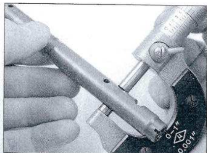
9.34a Measure the rocker arm shafts with a micrometer, in the area where the rocker arms ride
