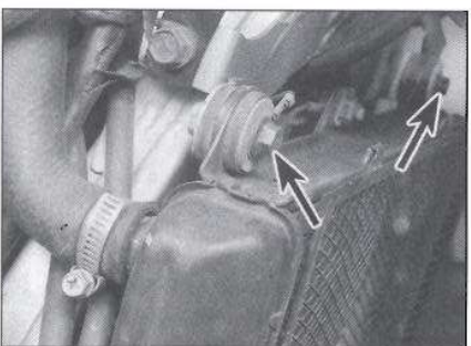
8.9 Remove the radiator mounting bolts (arrows)
