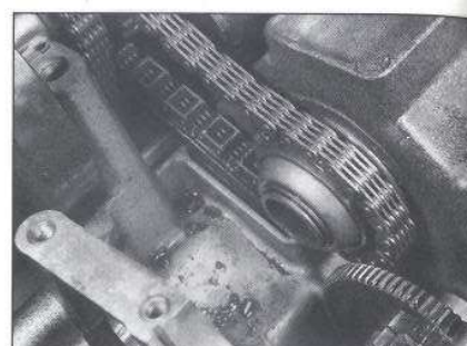
27.10b Disengage the idler shaft sprocket from the chain and remove the sprocket
