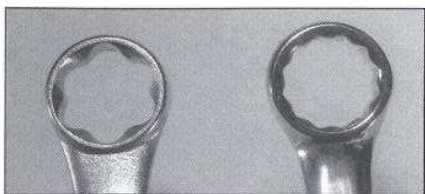
2.21 Comparison of surface drive ring spanner (left) with 12-point type (right)
