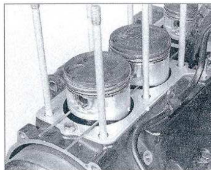
13.15 Slide rods under the pistons to support them as the cylinder block is lowered down
