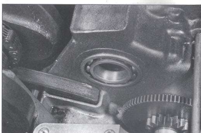
27.18 Replace the idler shaft bearing if it's worn or damaged
