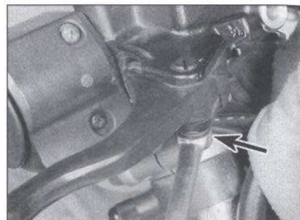
5.5 Remove the locknut then unscrew the brake lever pivot bolt
