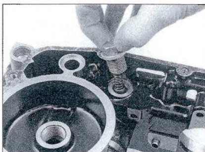
31.3 Remove the shift drum positioning bolt and lift out the spring and pin
