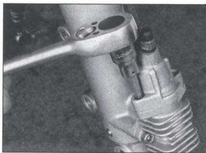
7.9 On A and B models, unbolt the brake plungers from the anti-dive units - don't disconnect the brake lines
