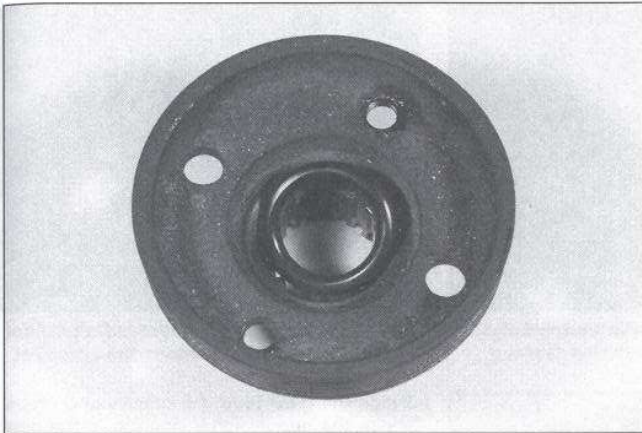
27.3 There's an O-ring behind the pulley bolt
