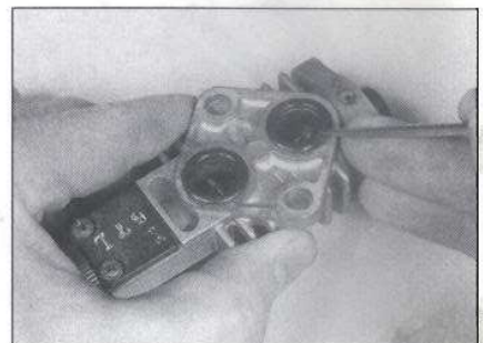
10.9 Be sure to check the O-rings on the anti-dive unit and replace them if necessary
