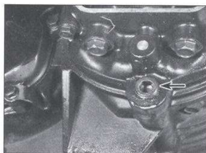
17.2 Remove the oil gallery plug (arrow) and install a pressure gauge
