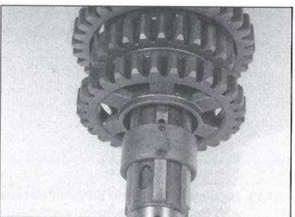
30.17d ... its bushing and fourth gear
