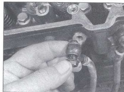
10.10c . . . there's a sealing washer on each side of the banjo fitting; replace these whenever they're removed
