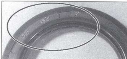
6.2 These oil seal markings indicate inside diameter, outside diameter and seal thickness
