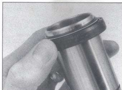
8.22 Install the oil seal
