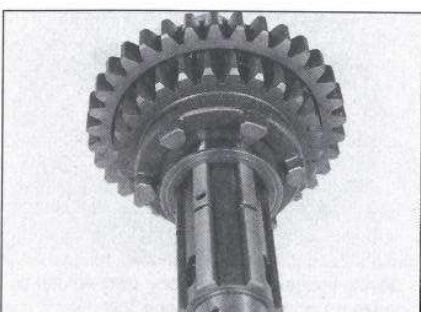
30.18a Remove the toothed washer ...
