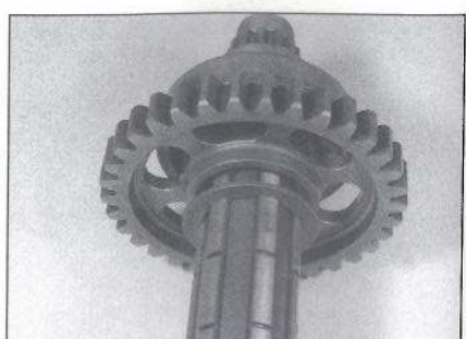
30.19b ... the toothed washer and second gear ...
