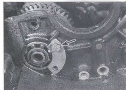
27.7c ... then unbolt the bearing retainer (arrow)
