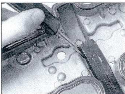
7.10 Pry the chain guide out of the cover if it's worn out
