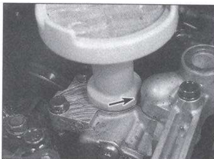
17.20 Install the pickup with its flat side (arrow) toward the oil pump
