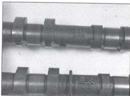
9.6b The intake and exhaust camshafts are identified by cast marks
