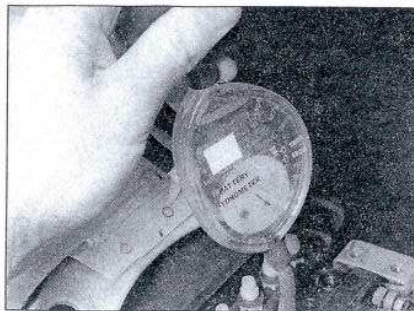
17.5 Check the specific gravity with an hydrometer
