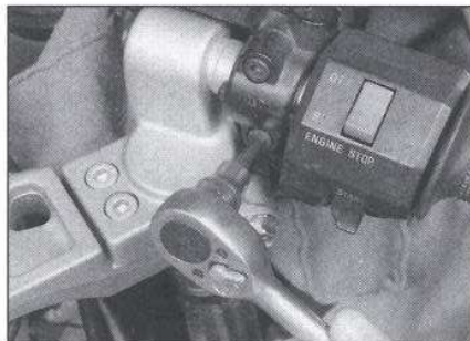
5.6 Remove the master cylinder mounting bolts
