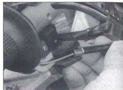
9.6 Pull the decelerator cable from the housing
