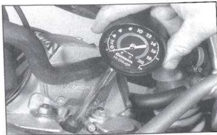
3.20 Using a rubber-cone type cylinder compression gauge
