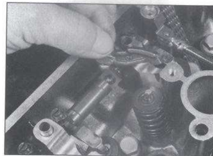
9.18a Lift the rocker arms out of the shafts ...
