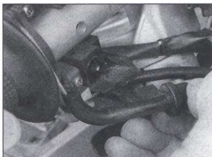
9.5 Detach the accelerator cable and guide from the rear half of the housing
