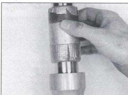
8.20b If you don't have the proper tool, a section of pipe can be used the same way the special tool would be used - as a slide hammer (be sure to tape the ends of the pipe so it doesn't scratch the fork tube)
