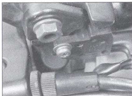
14.6 The brake light switch mounted on the brake lever is retained by a screw
