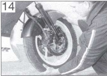
14 Check for wheel bearing play by trying to move the wheel about the axle (spindle)
