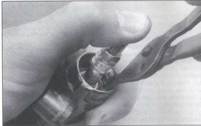
6.10a Depress the pushrod and remove the snap-ring from the cylinder bore
