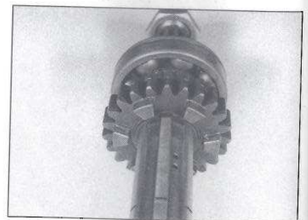
30.7a Remove the snap-ring ...
