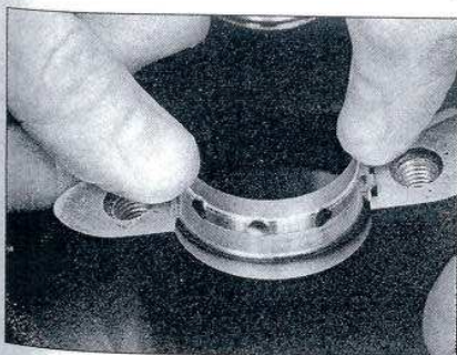
25.18 Make sure the tabs on the bearing inserts fit into the notches in the web
