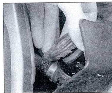
26.6 Remove the screw at the rear of the fairing inner panel to gain access to radiator cap
