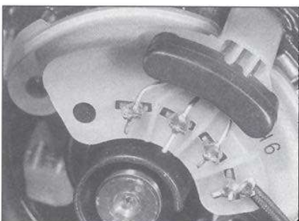
34.13 Unsolder terminal wires quickly to avoid damaging the rectifier
