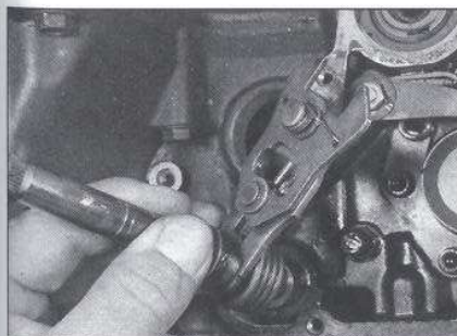
21.8b ... then take the shift mechanism out
