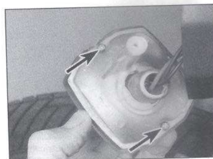
11.3 Remove these screws (arrows) to detach the lens from the reflector
