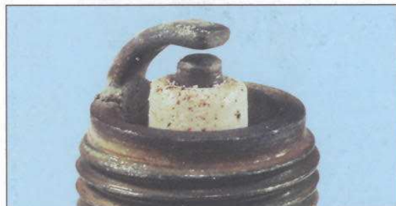
Overheating – A blistered white insulator and glazed electrodes. Caused by ignition system fault, incorrect fuel, or cooling system fault.
