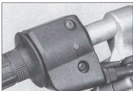
9.4 Remove the screws from the cable/switch housing and detach the front half of the housing
