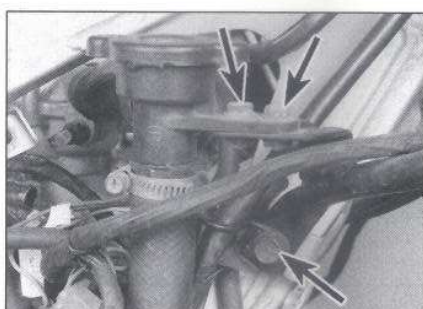
3.14 Unbolt the radiator filler neck from the fairing mount, then remove the right mounting bolt (arrows)
