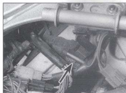
13.3 Location of the turn signal flasher (arrow)
