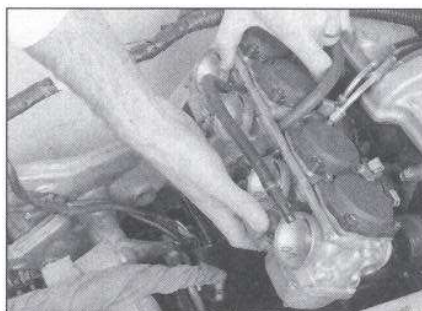
6.8a Gently pull the assembly to the rear, detaching the carburettors from the intake manifold tubes
