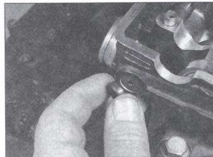
9.20b ... remove the shaft seal as the rocker shaft pushes it out ...
