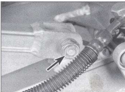
16.3 Remove the torque arm-to-swingarm nut and bolt, then support the brake caliper and torque arm with wire or rope
