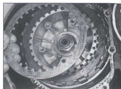
19.5c Take out the first steel plate, then continue removing friction and steel plates
