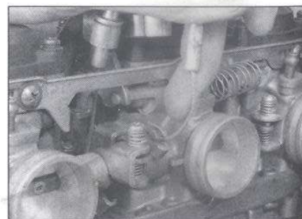
6.8b Raise the carburettors up, then align the throttle cables with the slots in the throttle pulley and pass the cables through
