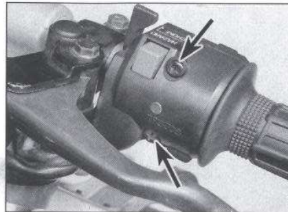
10.3 Remove the screws from the choke cable/switch housing, then pull the front half of the housing off the handlebar
