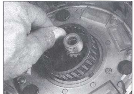
19.8b ... and lift out the bearing ...
