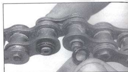
8.5 ... install the O-rings over the pin ends ...
