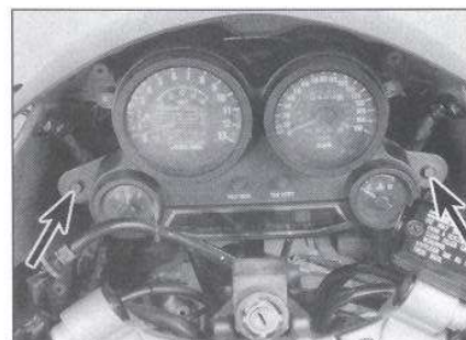
15.3 The instrument cluster is retained by two bolts (arrows)
