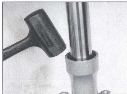
8.9 If you don't have the special tool, use a plastic dead-blow hammer to tap the outer tube from the inner tube
