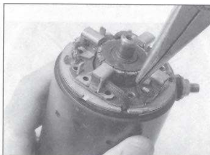
28.17b ... then pull the end of the spring 1/2 turn clockwise and seat the end of it in the groove in the end of the brush
