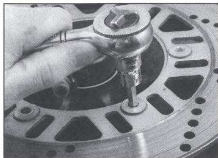
4.6 Loosen the disc retaining bolts a little at a time to prevent distortion
