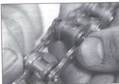
8.3 ... and separate the chain link
