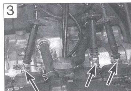
... and ensure that the metal bodies of the plugs (arrows) are earthed against the cylinder head
