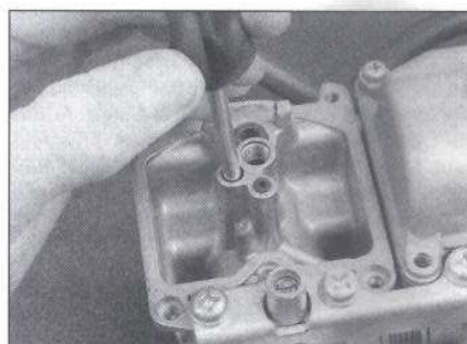
7.11 Unscrew the pilot jet
