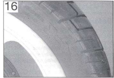
16 Tyre direction of rotation arrow can be found on tyre sidewall
