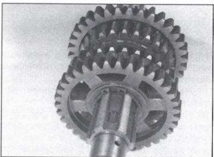
30.17a Remove the snap-ring ...
