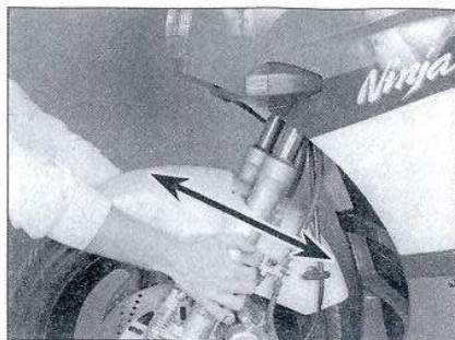
15.4 If play is felt when attempting to move the forks back-and-forth, adjust the steering head bearings
