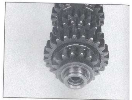
30.3 Remove the thrust washer and second gear
