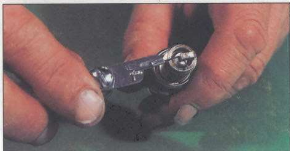
Electrode gap check – use a wire type gauge for best results.
