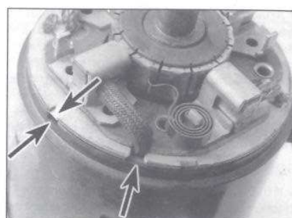
28.16 When installing the brush plate, make sure the brush leads fit into the notches in the plate (arrow) - also, make sure the tongue on the plate fits into the notch in the housing (arrows)
