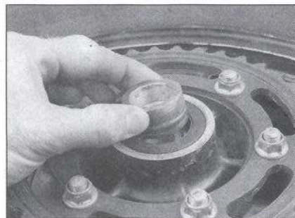
13.4a If you're removing the rear wheel bearings, lift out the coupling sleeve, ...
