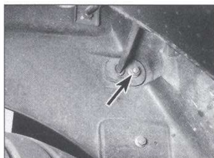
12.3b Rear turn signal nut (arrow)
