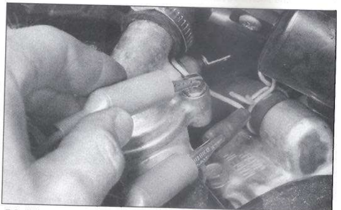
5.3 When the wire to the sending unit is grounded, the needle on the gauge should move all the way past the Hot mark
