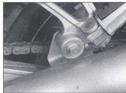
12.6 Remove the muffler mounting bolts from the passenger footpeg bracket on each side
