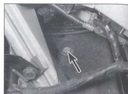
8.6 Remove the bolts that attach the baffle plate to the fan bracket (left side shown)
