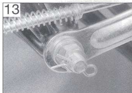
Brake torque arm must be properly secured at both ends
