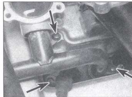
10.5 Location of the coolant pipe-to-cylinder head bolts (arrows) – the bolt on the left branch of the pipe isn't visible in this photo
