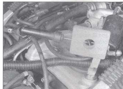
2.14 Connect the tester to a good ground (earth) and attach one of the spark plug wires - when the engine is cranked, sparks should jump the gap between the nails
