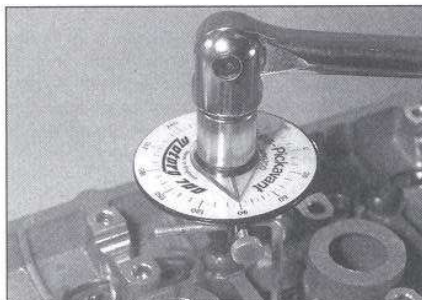
Angle-tightening cylinder head bolts
