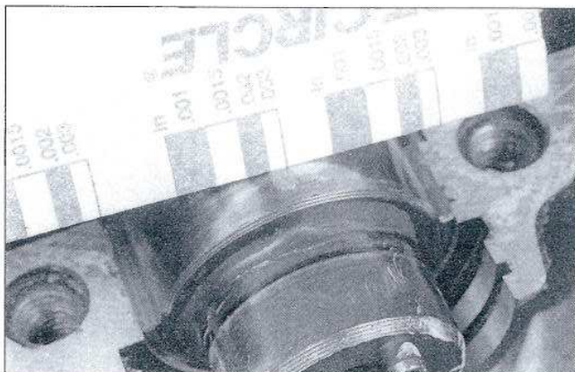
25.10 Measuring the width of the crushed Plastigauge (be sure to use the correct scale – standard and metric are included)
