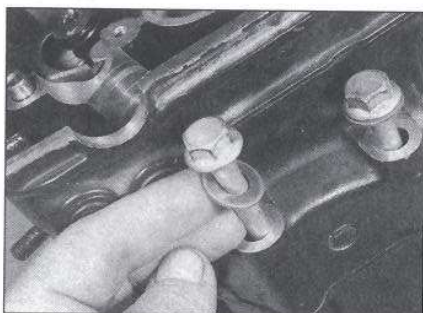
10.12a Lift out the cylinder head bolts and washers . . .
