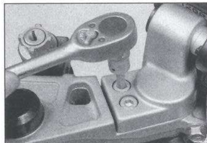
6.1 To detach a handlebar, remove the two bolts and slide the assembly off the fork tube - if it's stuck, wiggle it back and forth while pulling up
