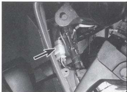
7.2 Unplug the headlight electrical connector and apply battery voltage to the red/yellow wire and ground (earth) the black/yellow wire - the light should come on
