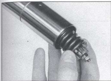
8.4 Remove the TCV from the inner tube
