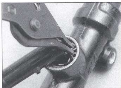
6.8a Remove the snap-ring that secures the fluid inlet fitting
