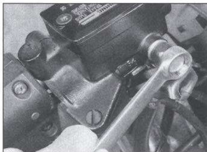
5.4 Use a six-point box-end wrench to remove the banjo bolt from the master cylinder - be prepared for spillage
