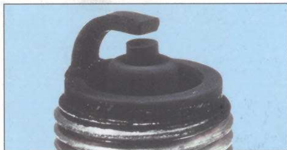
Carbon fouling – Dry, black sooty deposits leading to misfire and weak spark. Caused by an over-rich fuel/air mixture, faulty choke operation or blocked air filter.
