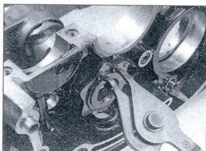
31.6 Remove the snap-ring and slide the operating plate off the shift drum
