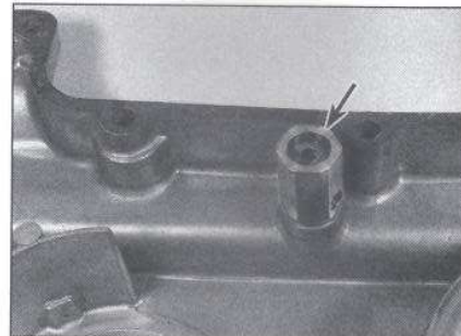
18.2 The oil pressure relief valve is mounted in the oil pan (arrow)
