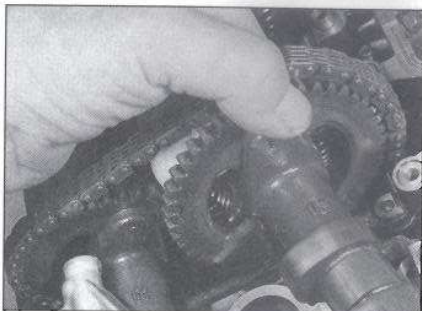
9.6a Lift the camshaft chain, disengage it from the sprocket and guide the camshaft out
