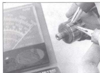
28.11a Continuity should exist between the commutator bars
