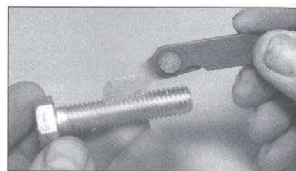
2.12 Using a thread gauge to measure pitch
