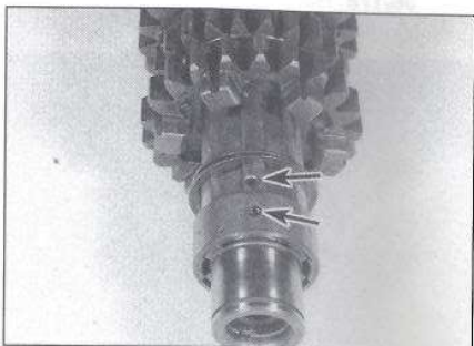
30.13 Be sure to align the bushing oil hole with the shaft oil hole (arrows)
