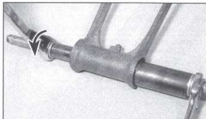
5.10 Drawing the bearing out of the suspension arm
