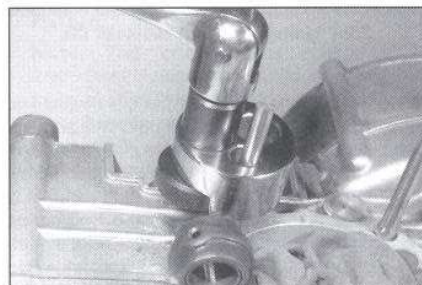
2.17 Using a stud extractor tool to remove a broken crankcase stud
