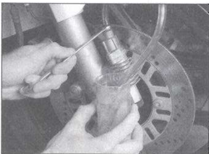
8.9a After bleeding the front calipers on 600 A and B models, bleed the anti-dive units...
