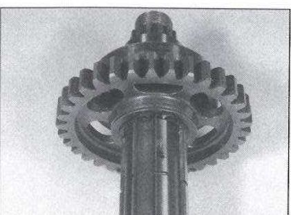
30.19a Remove the snap-ring ...
