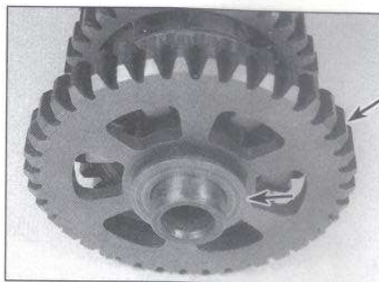
30.15 Remove the thrust washer (arrow) and first gear
