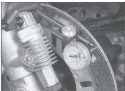
4.3 Use a dial indicator to check disc runout - if the reading exceeds the specified limit, the disc will have to be replaced
