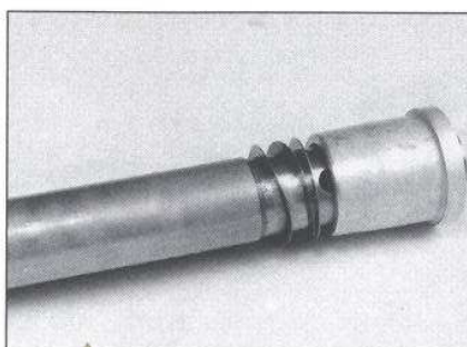
8.18 Install the damper rod washers and base on the end of the damper rod - the flat washer should be between the two spring washers
