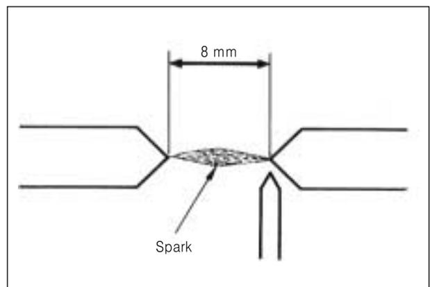
**IGNITION COIL (Checking with Pocket Tester)**
