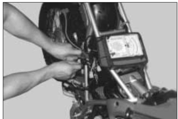
Check the coil for "open", "ground" and ohmic resistance. The coil is in good condition of the resistance is as follows.
