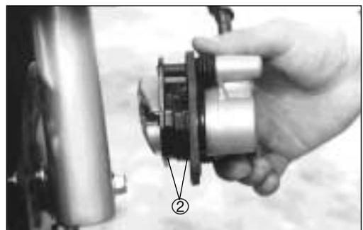
**CALIPER REMOVAL AND DISASSEMBLY**
