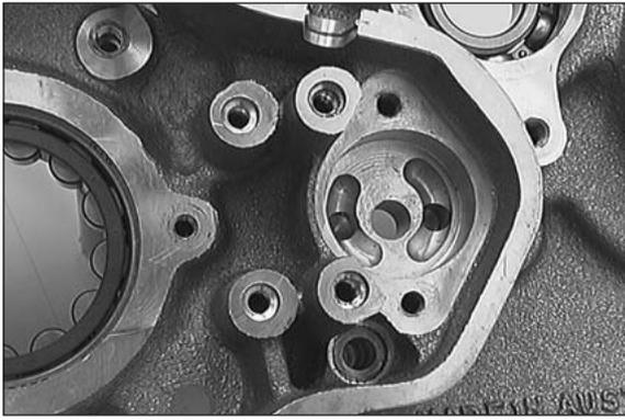
The oil pump housing must not have any score marks or seizing marks.
