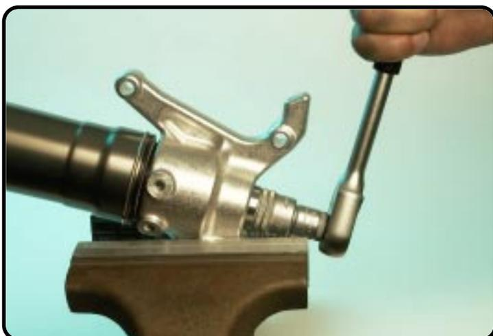
Unscrew the compression holder out of the axle-clamp. (size 19)
