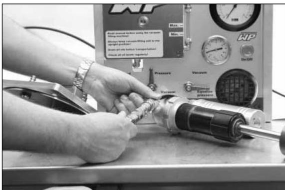
Filling procedure using the external tank
