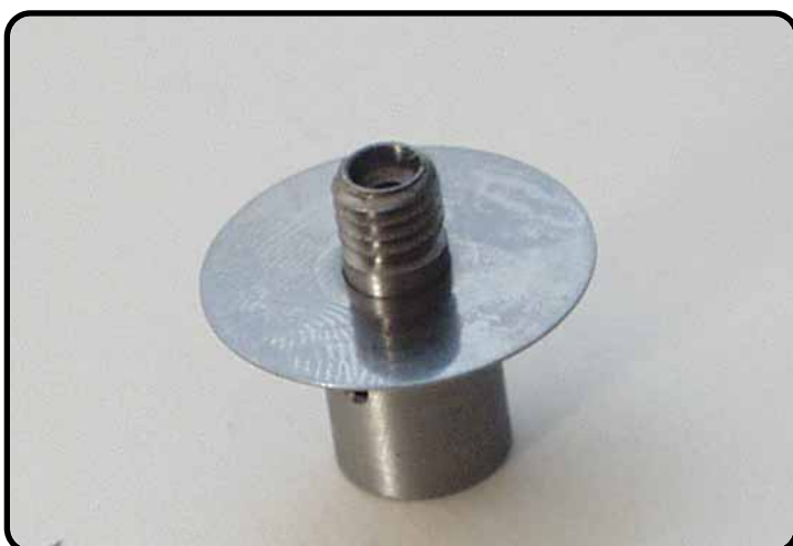
Damping holder with shims (setting).
