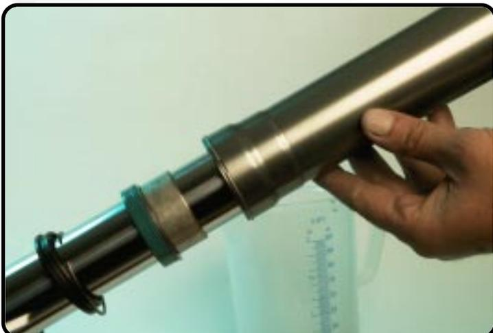
Slide carefully the outer-tube over the inner-tube.
