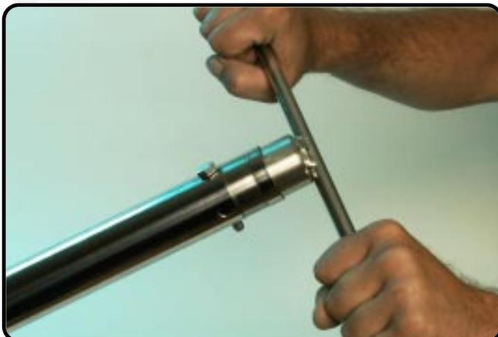
...and unscrew the inner-tube from the axle-clamp.
