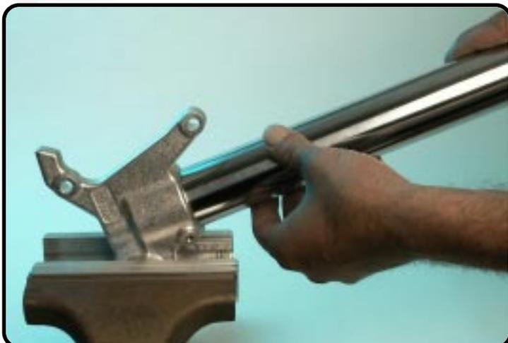
Assemble the inner-tube in the axle-clamp.
