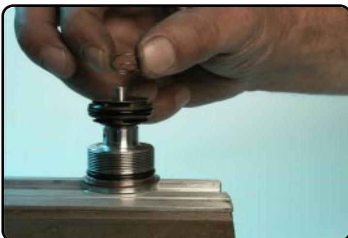
Remove the check-valve spring. Pay attention to the assembling direction!!!
