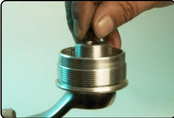
Assemble the O-ring into the innerside of the holder.
