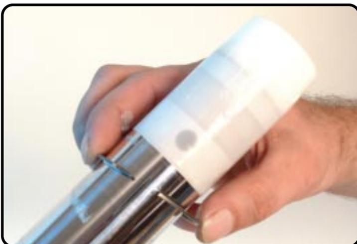
Replace the circlip.
