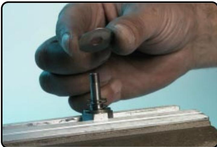
Remove check-valve shims.
