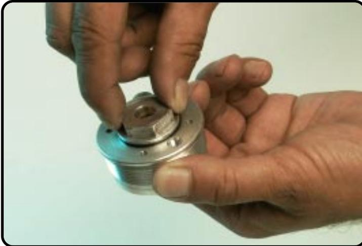
Assemble the holder in the screw-cap.
