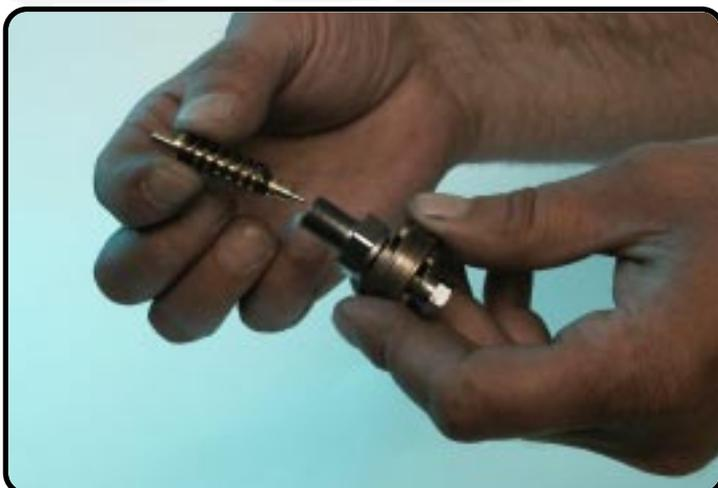
Pull the rebound needle with spring out of the tap rebound.
