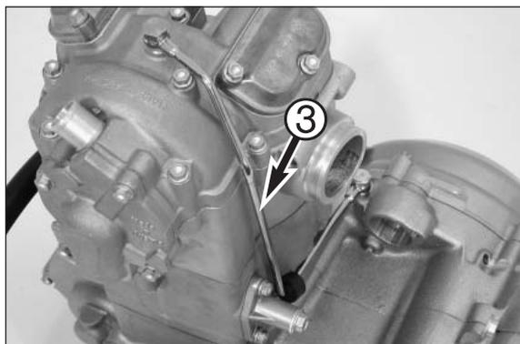
NOTE: Place the oil line such that it does not touch the engine. The oil line must not be twisted during tightening.
