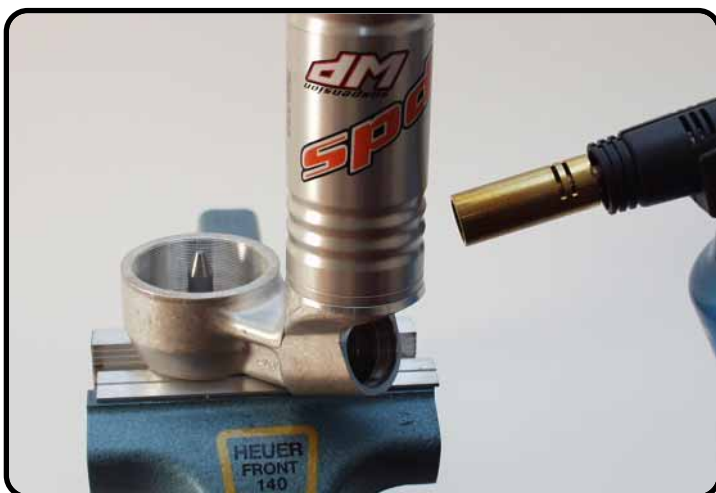
Heat the reservoir near the bottom.
