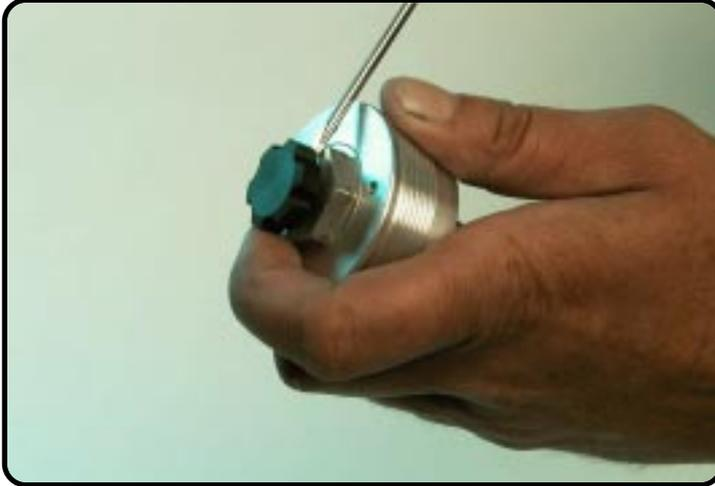
Disassemble the adjusting knob from the screw-cap.
