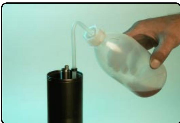
Push the piston-rod and outer-tube fully down and adjust the oil level (airchamber) with T137S.
