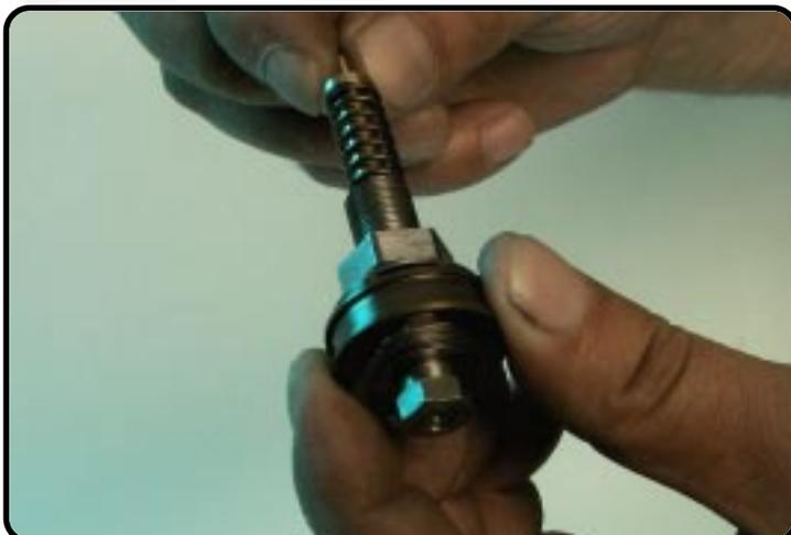
Mount the needle with spring into the tap rebound.
