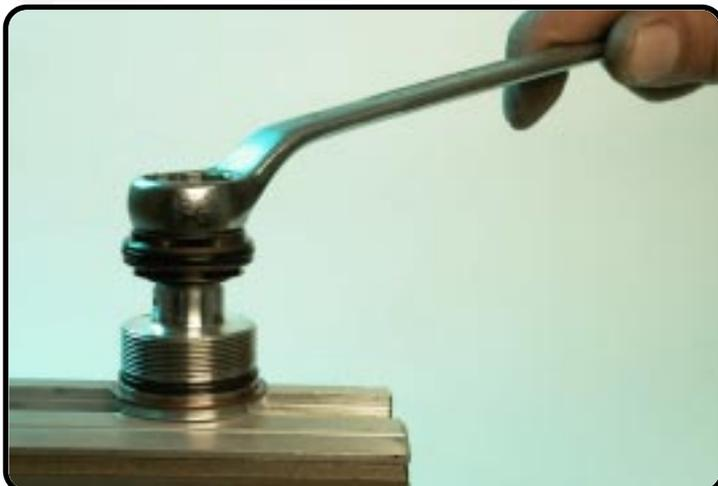
Clamp the compression holder in the vice and unscrew the check-valve nut. (size 17)
