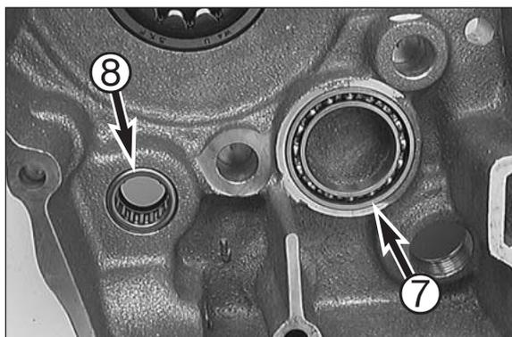
**Grooved ball bearing of the shift roller ⑦**
