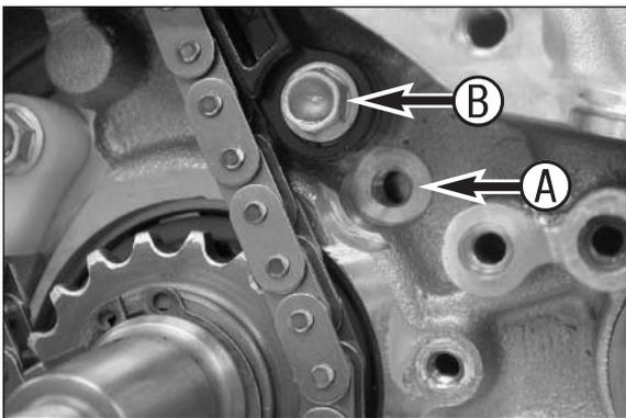
NOTE: 2 mounting points for the tensioning rail are provided for models from 2003. The tensioning rail is attached to point A on the 450 SX model.
