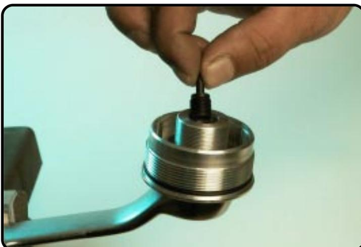
Turn the plastic adjustment tube holder out of the screw-cap.
