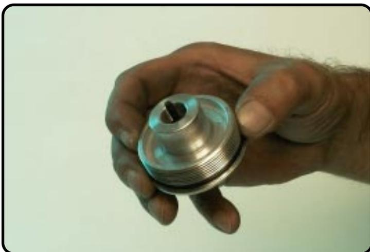
Screw the holder adjustment tube in the screw-cap.
