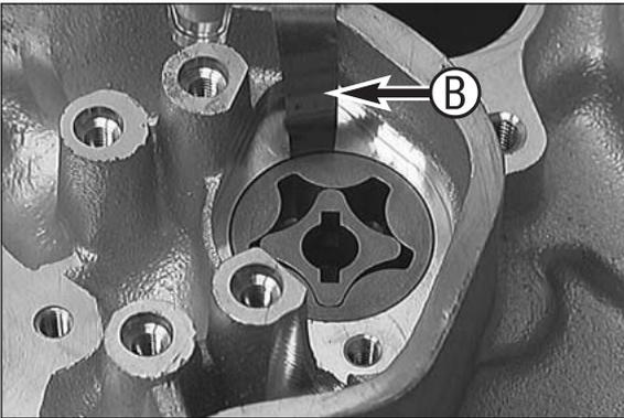
outer rotor - inner rotor: max. 0.20 mm
