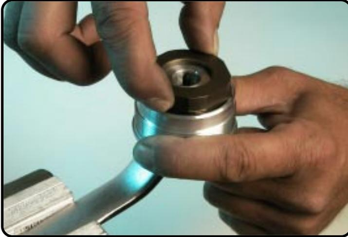
Turn the washer so that its fitting into the screw-cap.
