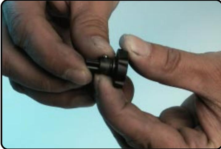
Grease the steel balls with spring (T159) and assemble those in the adjustment knob.
