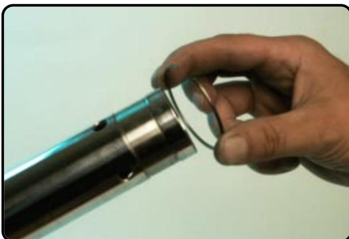
Remove the circlip.
