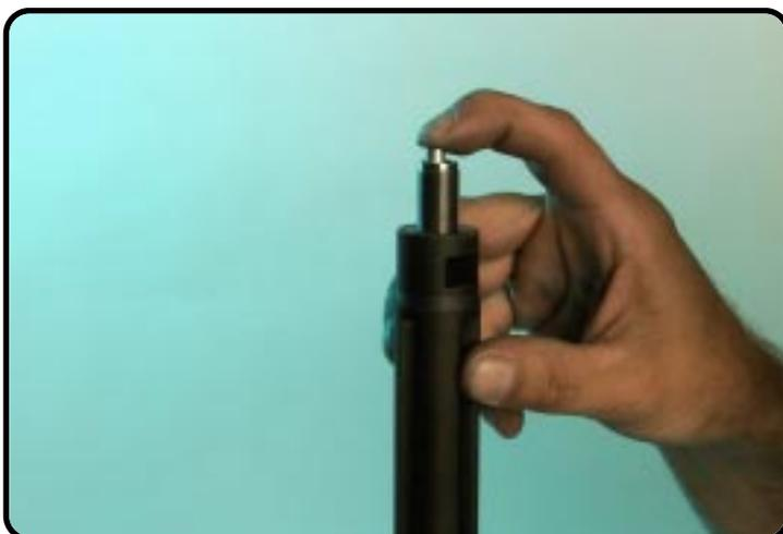
Move the piston-rod (keep the adjustment tube on his place) several times up and down till you feel that the cartridge is full with oil, (the damping is smooth over the entire stroke) mostly it is necessary to fill some (not too much) extra oil in the forkleg.
