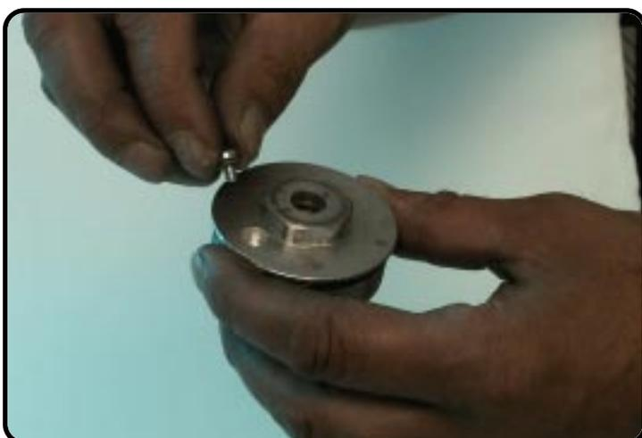
Remove air release screw with O-ring.
