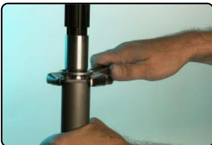
Tighten the screw sleeve.
