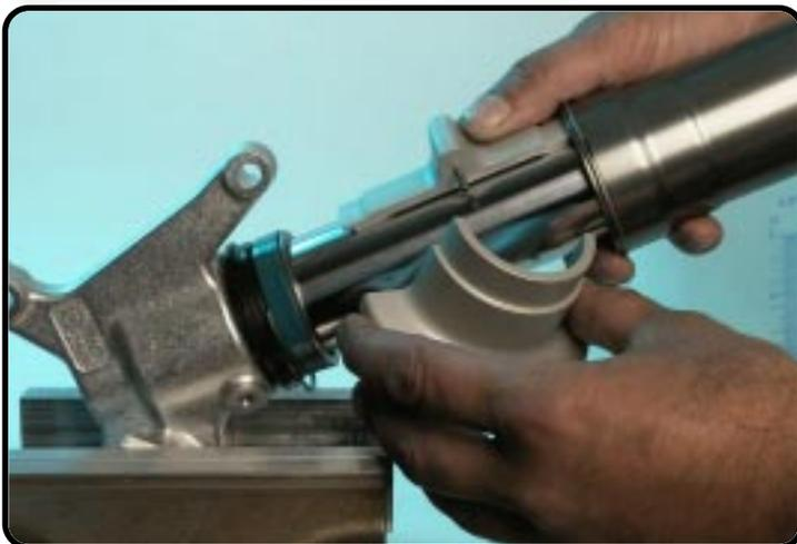
Assemble with T1402S the DU-bush - with the flat side- and...
