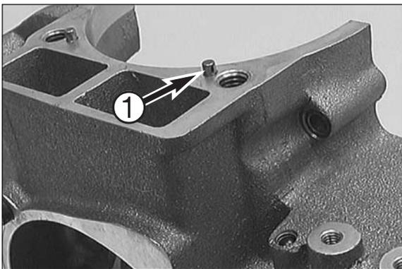
Check the 2 dowels **1** for tight fit and if necessary, adhere them using Loctite 243.
