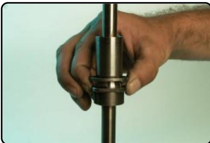
Clamp the piston-rod “not too tight” in at the other side and replace the screw sleeve with spring retainer.
