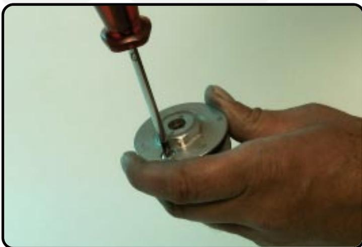
Assemble the air release screw
