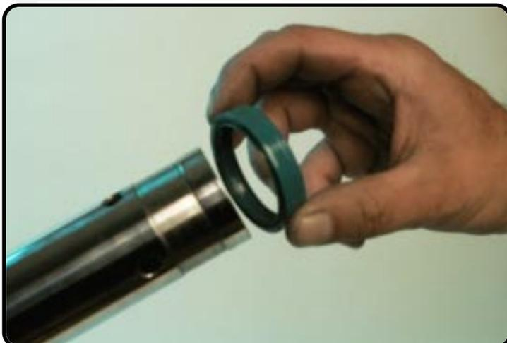
Disassemble the oilseal.
