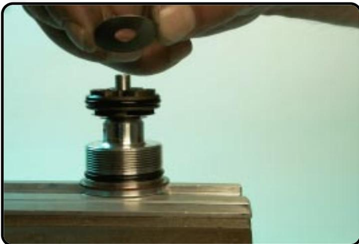
Remove the check-valve shim.
