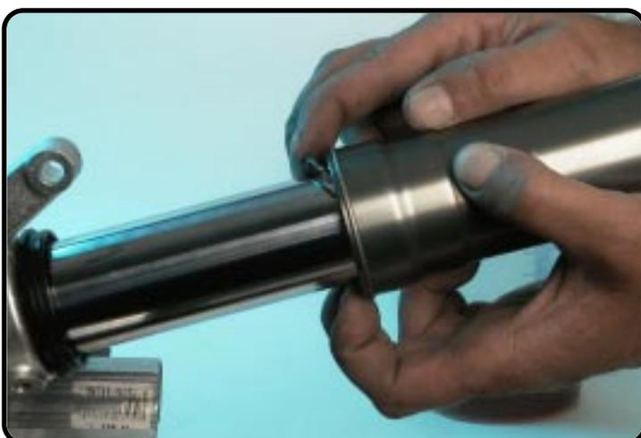
Assemble the circlip into the groove of the outer-tube.
