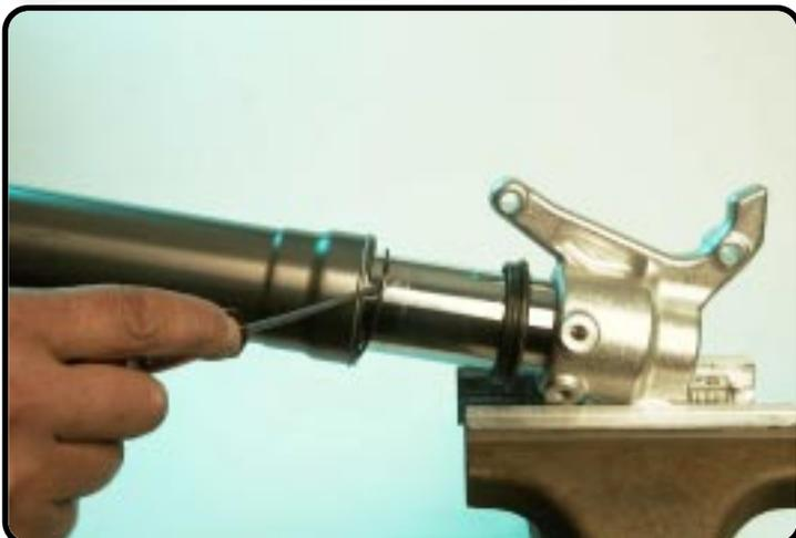
Disassemble the circlip.
