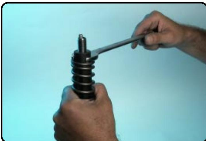
Pull the spring downwards and place open-end spanner 22 on the hydraulic stop.
