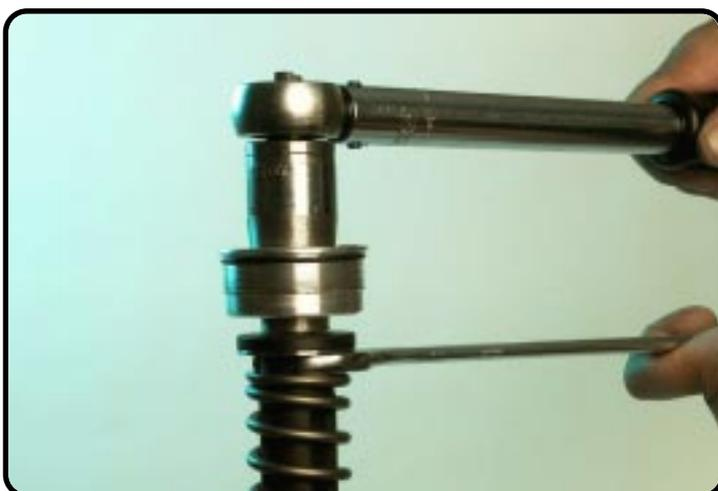
Screw down the screw-cap, till the hydr. stop is against the screw-cap and tighten it to a torque of 25Nm.
