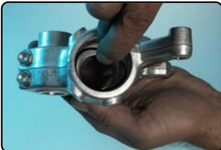
Replace a new O-ring in the groove of the axle-clamp.
