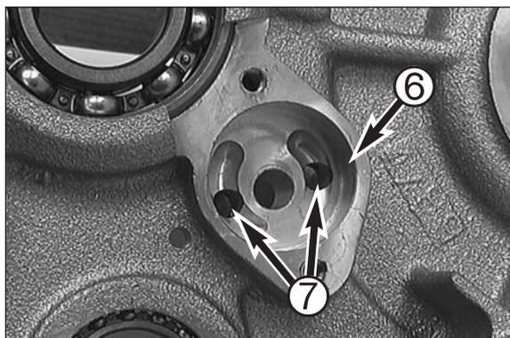
The oil pump casing **6** must not have any score marks or seizing marks.
