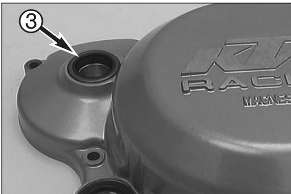
**Clutch cover****Shaft seal ring of kickstarter shaft ⑥**
