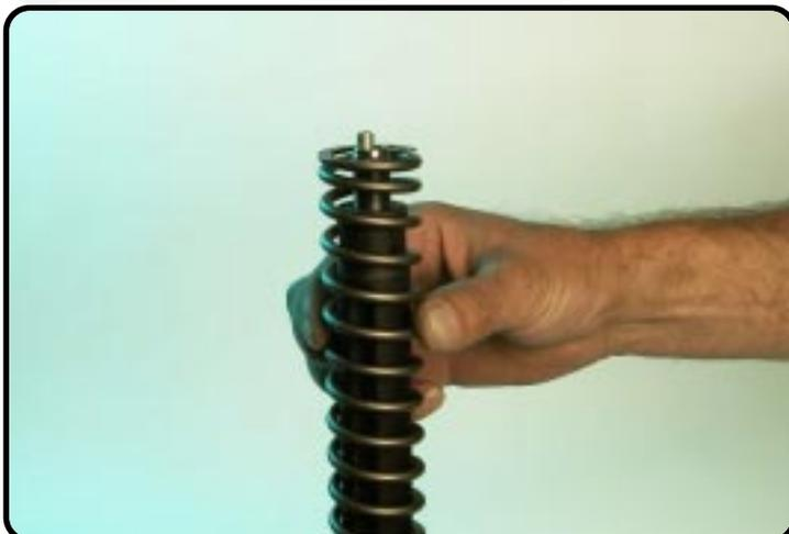
Pull the piston-rod out and assemble the spring.
