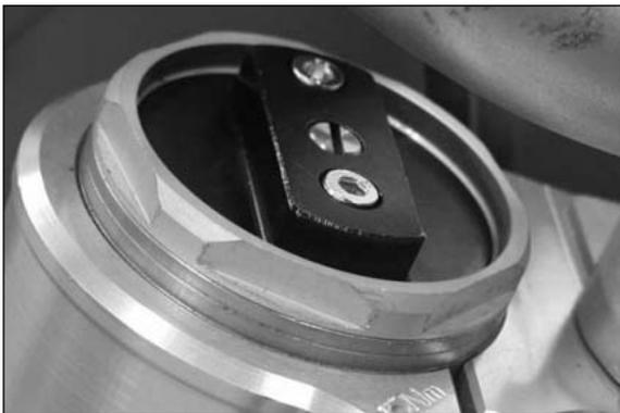
NOTE: The maximum riding height is the level of the second groove!
