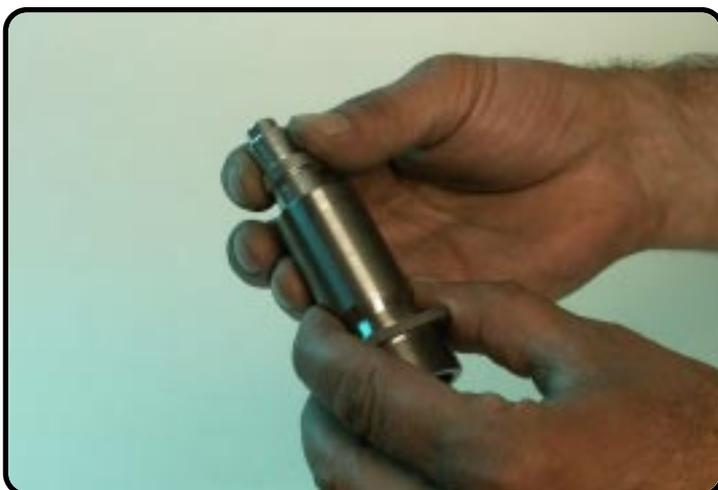
Disassemble the DU-bush with T507 and press it out the screw sleeve with support of the vice.
