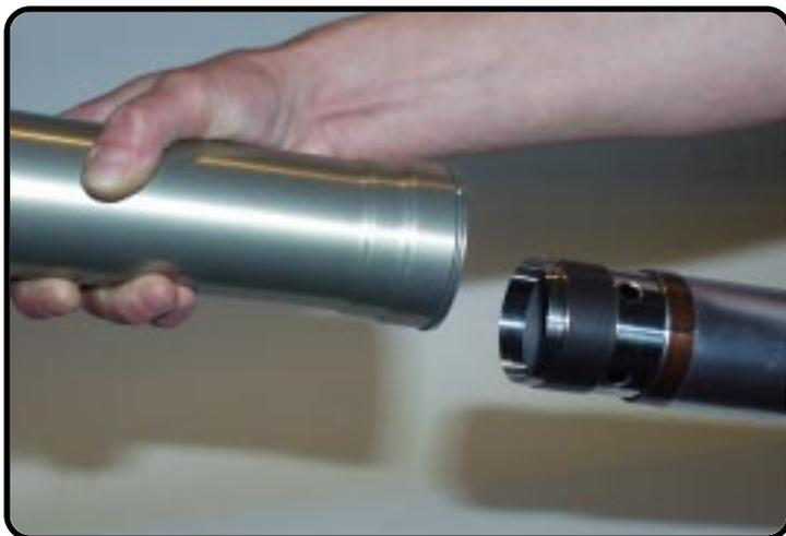
Slide carefully the outer-tube over the inner-tube.
