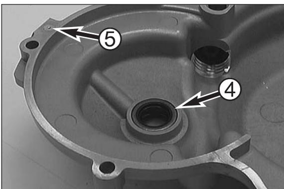
**Shaft seal ring of crankshaft ④**
