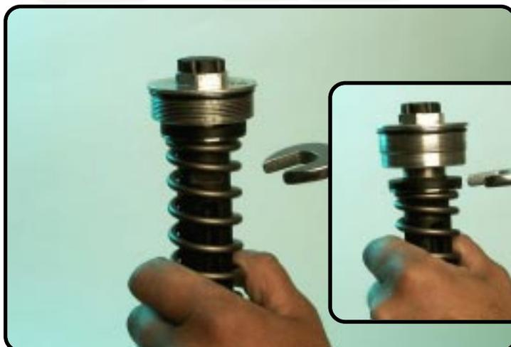
Pull the spring downwards and remove the spanner.
