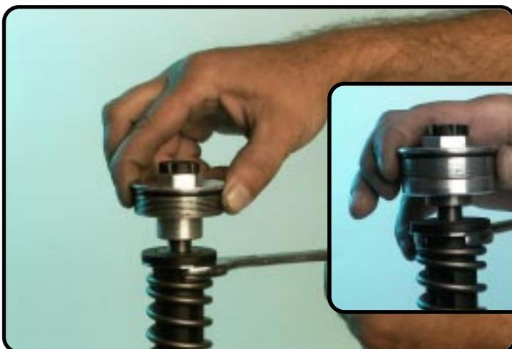
Screw handtight the screw-cap on the piston-rod.
