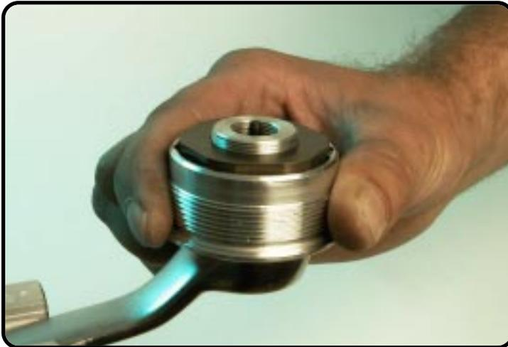
Turn the spring washer past the springing groove.
