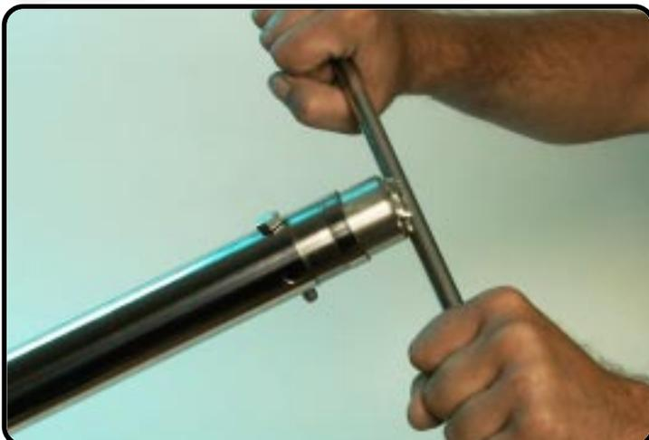
...and unscrew the inner-tube from the axle-clamp.
