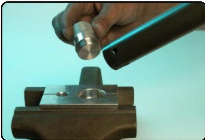
1. Clamp the tube with plug in the clamping-block (Tool T508S + T509).
