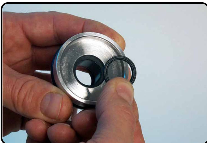
Assemble the quad ring.
