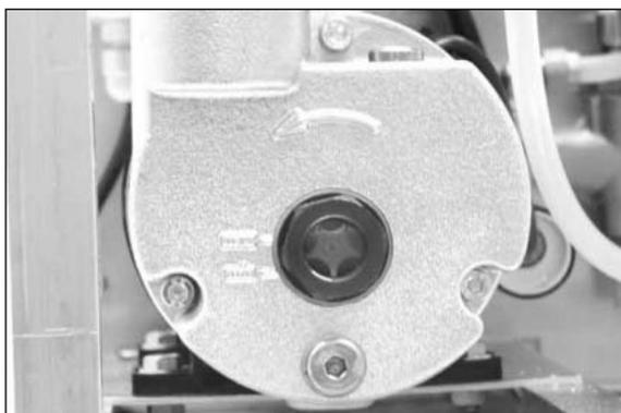
Checking / adjusting oil level vacuum pump
