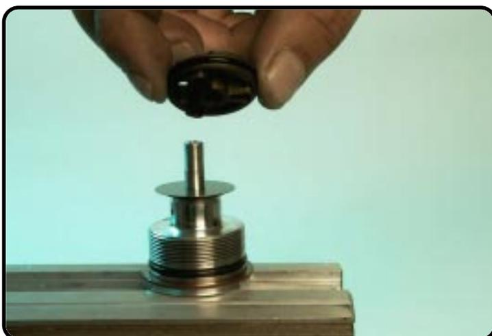
Disassemble the compression piston with O-ring.
