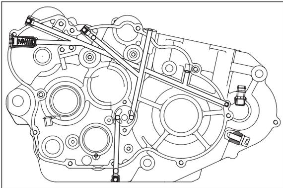
Clean all oil ducts with compressed air and check them for unobstructed passage.
