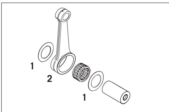
NOTE: From Model 2001 onwards the conrod **2** is mounted without thrust washers **1**, but the conrod overhaul set (see drawing below) is the same for both Model 2000 and 2001. The trust washers included in the set are not used for Model 2001 engines.
