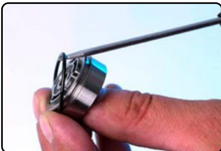
Disassemble the O-ring.
