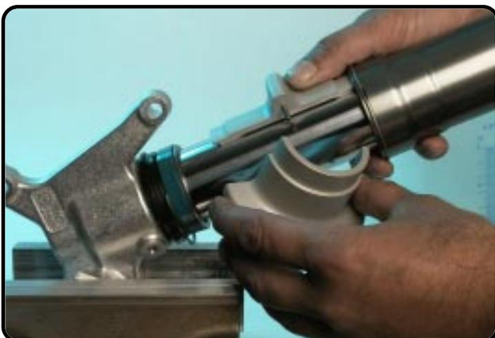
Assemble with (4357) T502S / (4860) T1402S the DU-bush -with the flat side- and...
