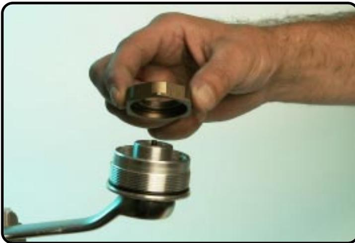
Remove the spring washer. Pay attention to the assembling direction!!!
