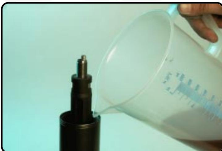
Keep the outer-tube down and the piston-rod a little bit extended (like picture), fill the forkleg with oil till the edge of the outer-tube, wait a few moments, you will see air bubbles rising up.
