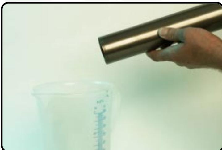
Drain the oil out the forkleg.
