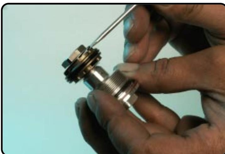
Check if the spring is correctly placed in the chamber of the nut.
