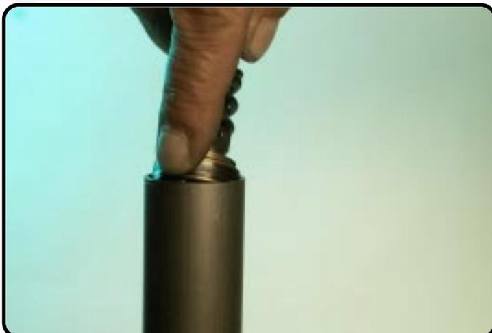
Clamp the tube with plug in the clamping block (T508S and T509) and assemble the piston-rod "cpl." into the tube.
