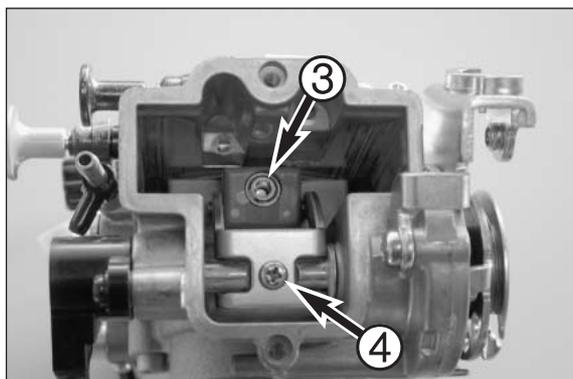
– Remove screw ③ and pull the jet needle out of the throttle slide.
