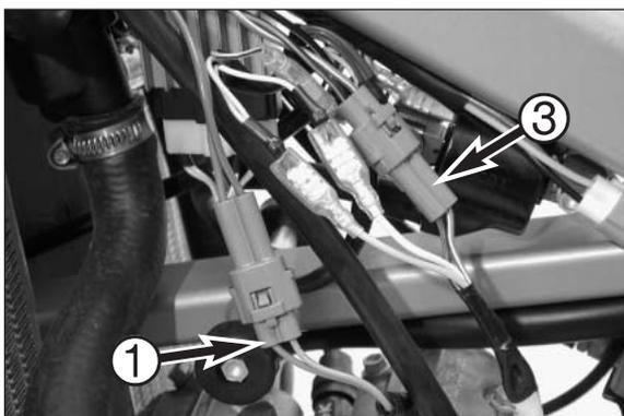
Check the **pulse generator** for an output signal – two-pin connector **1** with green and red cable colors (also see circuit diagram on next page):
