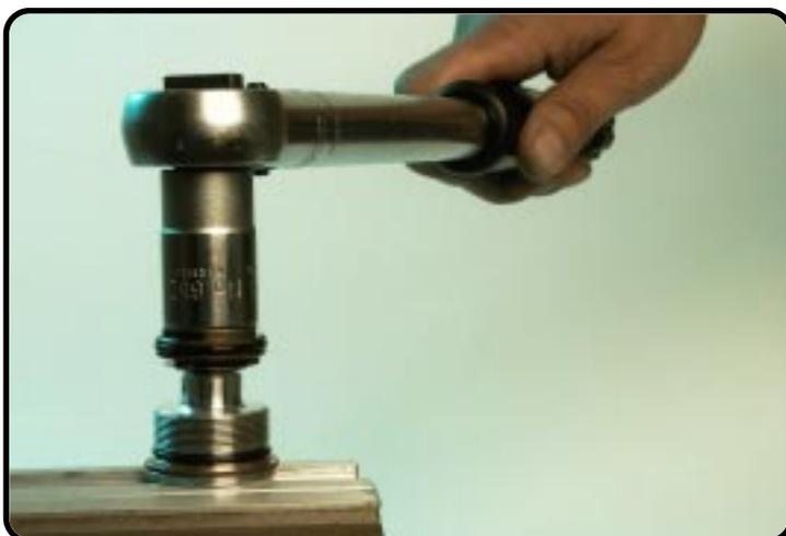
...to a torque of 5Nm.
