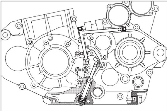
Blow compressed air through all oil ducts and check them for unobstructed passage.
