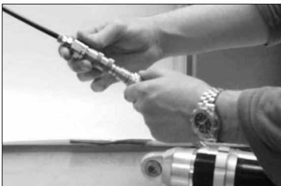
Filling procedure without external tank
