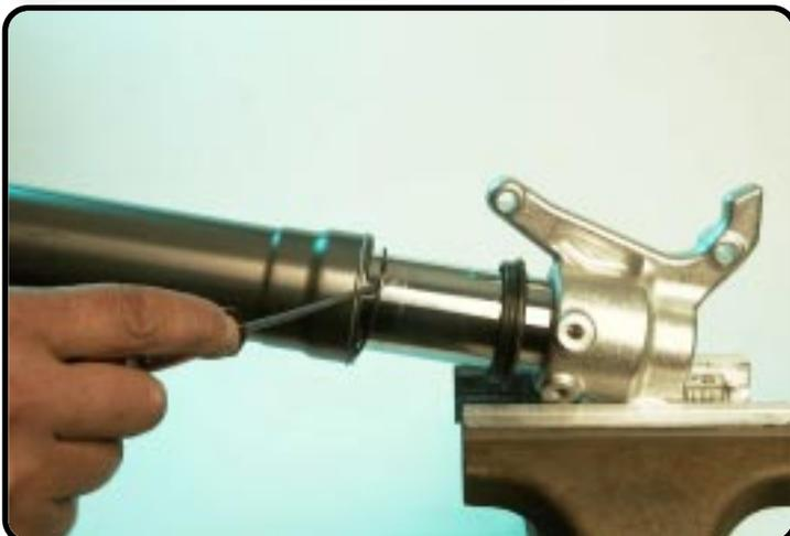
Disassemble the circlip.
