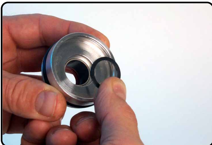
Assemble the back-up ring.
