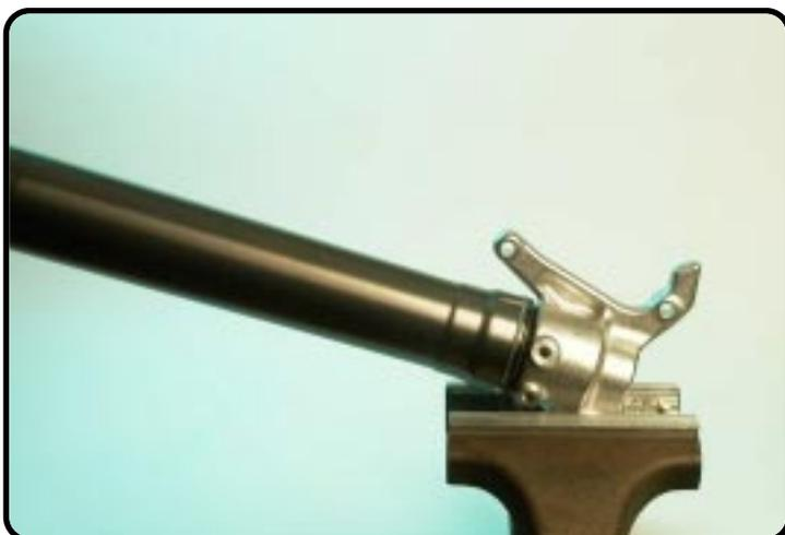
Clamp the axle-clamp in the vice so that the forkleg is at an angle of  $\pm 45$  degrees.
