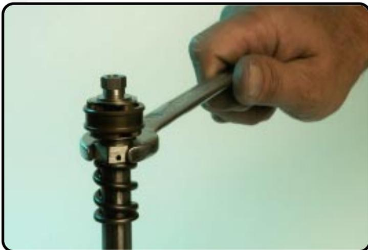
Clamp the piston-rod (at the level where the hydraulic stop is mounted) in T508S and unscrew the rebound tap. (Size 17)
