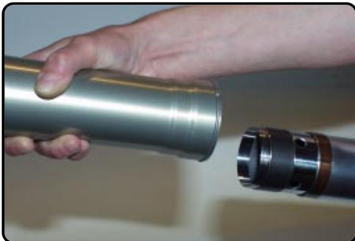
Pull with both hands the outer-tube from the inner-tube.
