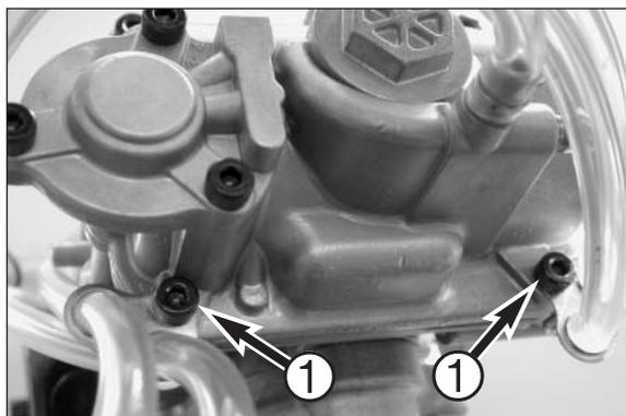
– Dismount the carburetor and remove any coarse dirt.
