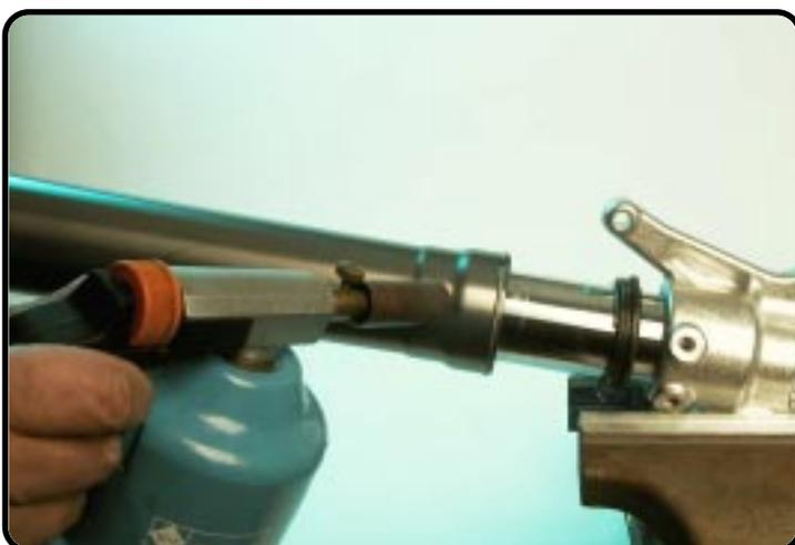
Heat the outer-tube near the oilseal.
