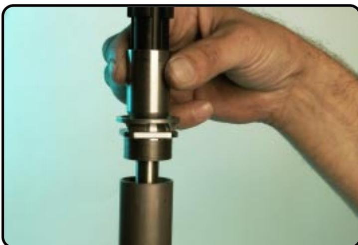
Turn the screw sleeve out of the tube.
