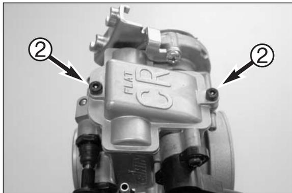
– Remove both screws ② and remove the slide cover and gasket from the carburetor.
