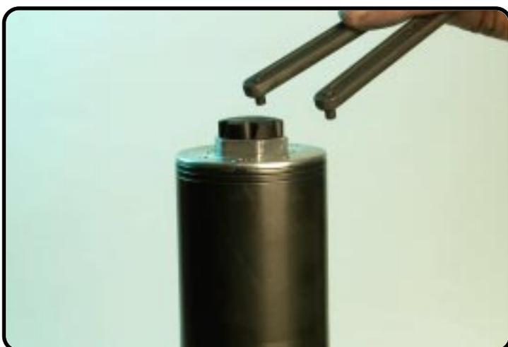
Clamp the outer-tube in T1403S and
