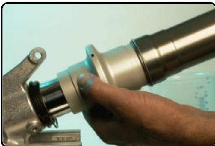
...and tap the oilseal into the outer-tube.
