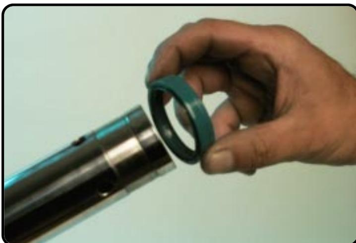
Disassemble the oilseal.
