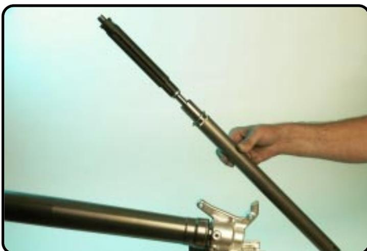
Disassemble the cartridge out the
