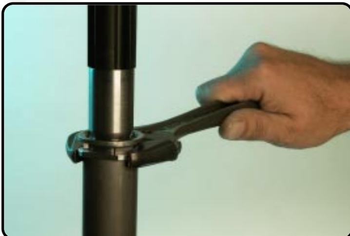
Unscrew the screw sleeve (size 22).
