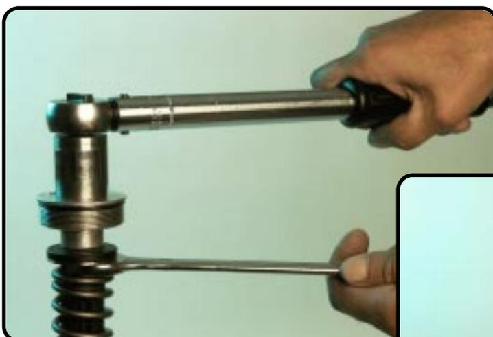
Screw down the screw-cap, till the hydr. stop is against the screw-cap and tighten it to a torque of 20Nm.
