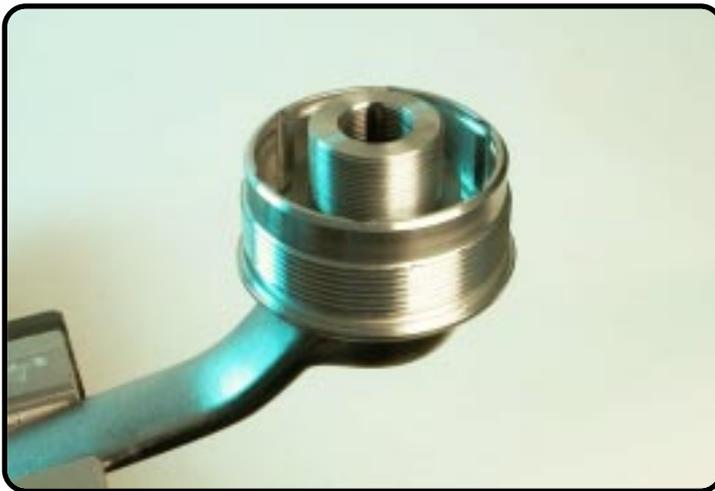
Screw plastic holder adjustment tube into the holder.
