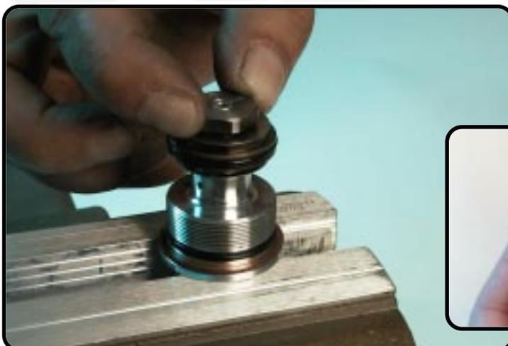
Wetting the thread of the nut with T132 and tighten it...
