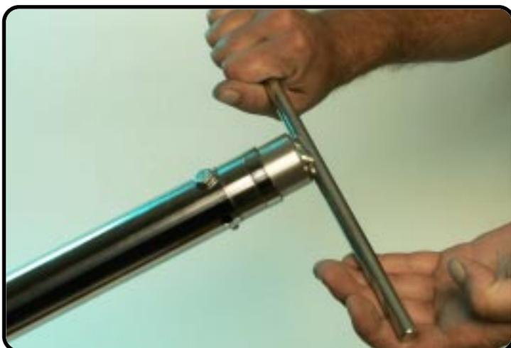
Screw very tight the inner-tube with T503S / T1404S.
