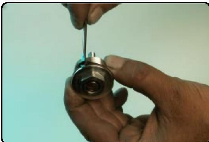
Disassemble the O-ring.
