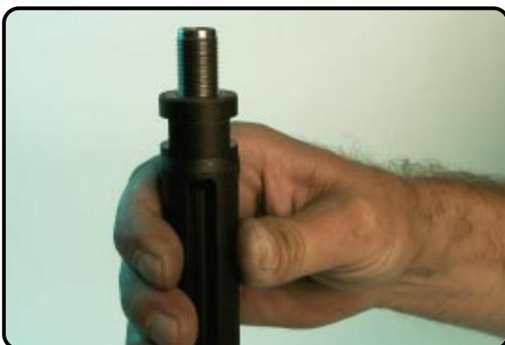
Screw the hydraulic stop "hand tight" to the end of the thread of the piston-rod.
