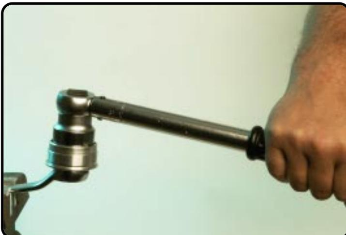
Tighten the nut to a torque of 100Nm.
