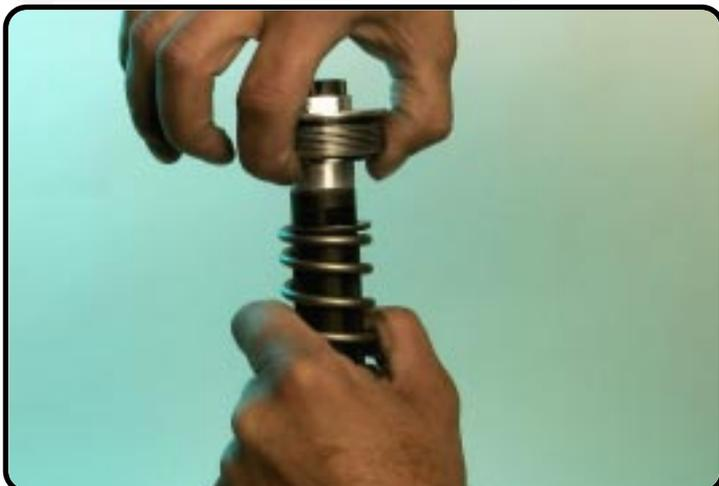
Clamp the forkleg (axle-clamp) in the vice and let the outer-tube down. Pull the spring downwards...
