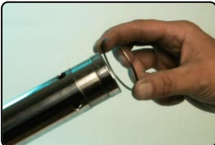
Remove the circlip.
