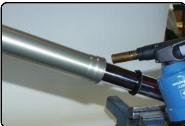
Heat the outer-tube near the oilseal.
