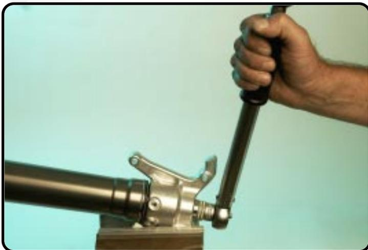
Assemble the cartridge in the center of the axle-clamp and tighten the holder compression to a torque of 25Nm.
