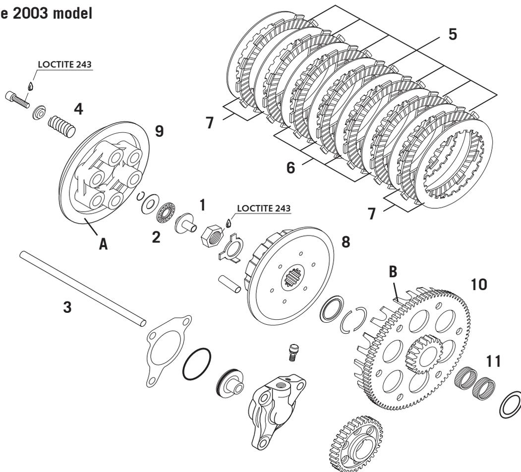
**Checking the clutch for wear - from the 2003 model****Pressure piece ①**
