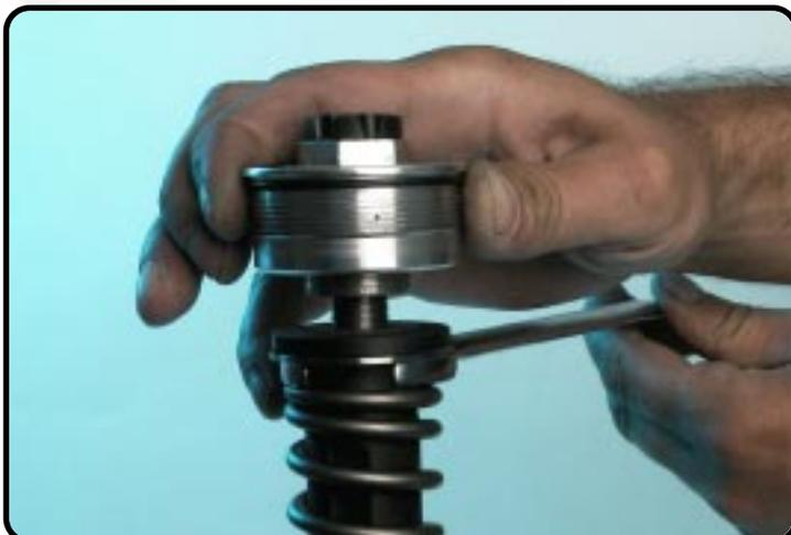
Screw handtight the screw-cap on the piston-rod.
