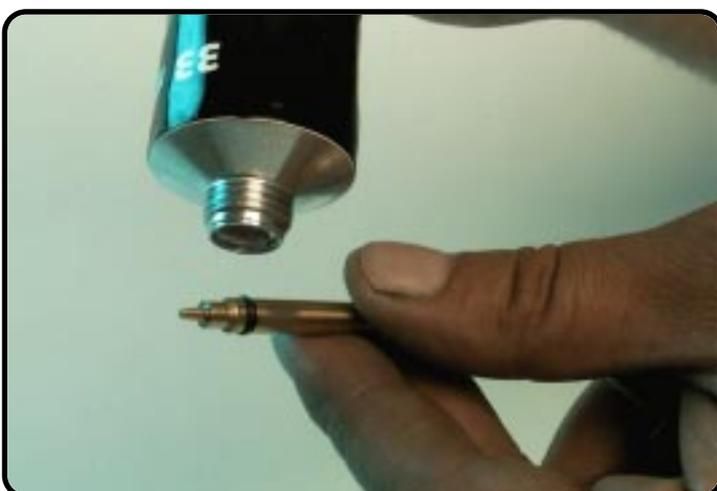
Grease the O-ring of the adjustment
