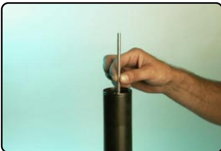
Remove the adjustment tube with the O-ring.
