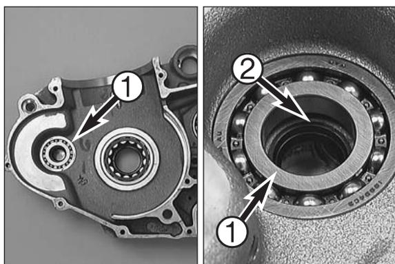
Grooved ball bearing **1** and seal ring **2** of balancer shaft.
