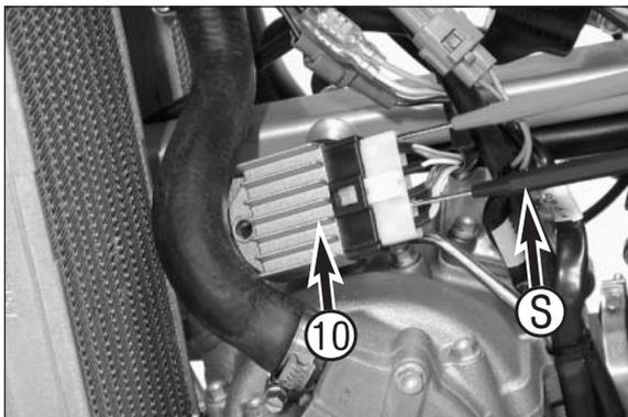
Check **regulator rectifier output voltage ⑨** (also see circuit diagram on opposite page) cable colors yellow/red, regulator rectifier ⑩ connected, capacitor disconnected (if installed) and fuse ⑫ removed:
