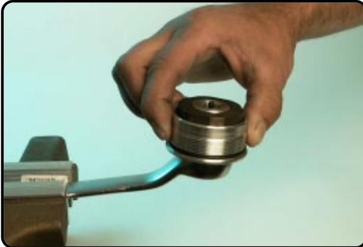
Screw the screw-cap to the right so that the spring washer is turning out of the screw-cap PA.
