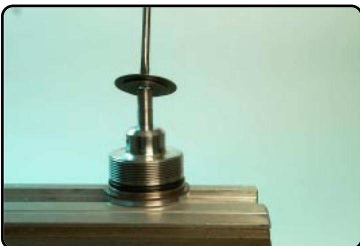
Place a screwdriver on top of the holder and remove the entire shim packet.
