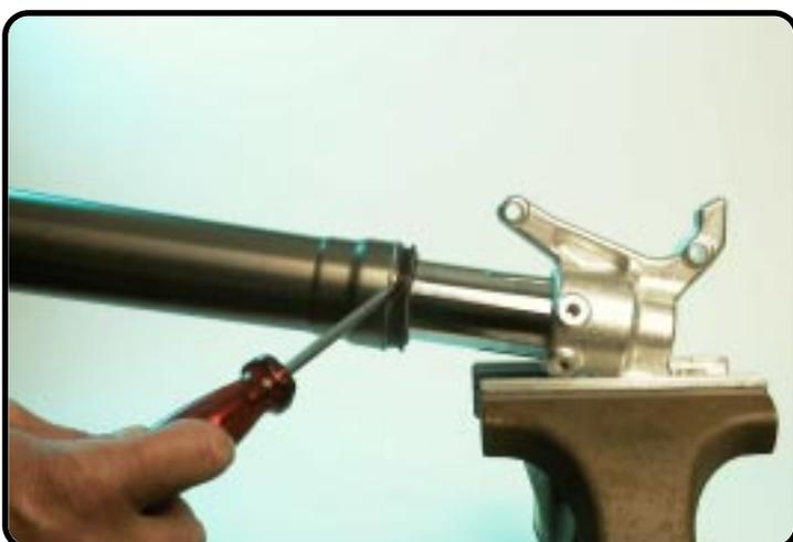
Disassemble the dust-wiper.
