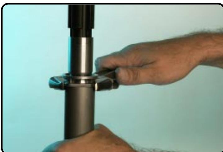
Tighten the screw sleeve.
