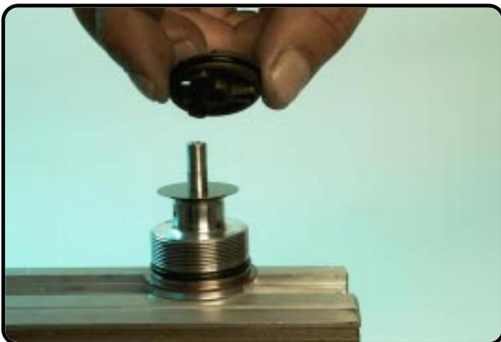
Disassemble the compression piston with O-ring.
