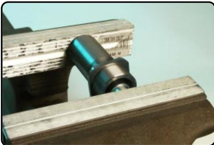
Press with T507 the DU-bush into the screw sleeve.
