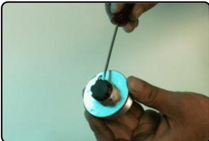
Disassemble the adjustment knob.
