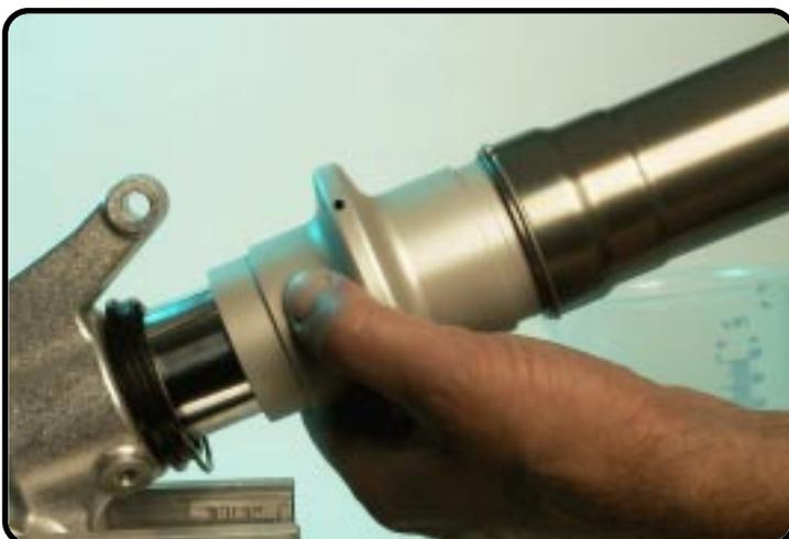
...and tap the oilseal into the outer-tube.
