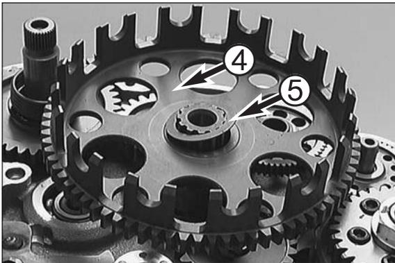
NOTE: In the 2001/2002 models, disc ⑤ is replaced by a stepped disc and the bushing by 2 needle bearings ⑥ (see illustration).
