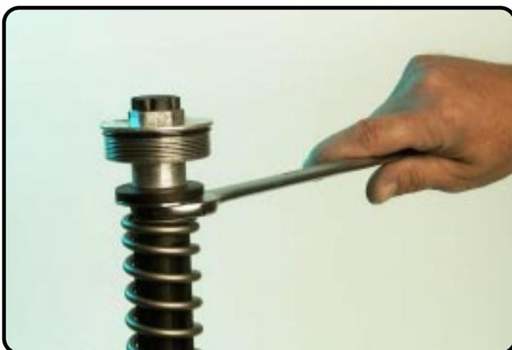
...and place open-end spanner (size 22) on the hydraulic stop.
