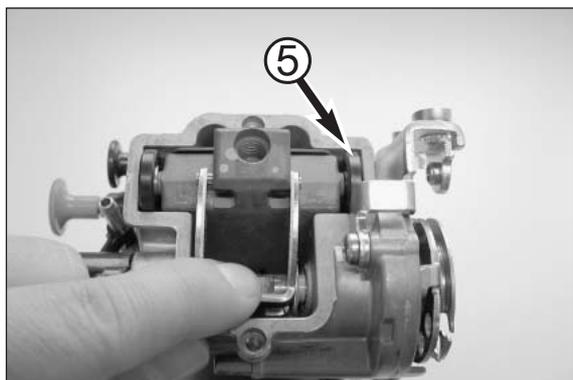
– Pull the throttle slide arm up and take the throttle slide roller ⑤ and the slide shim out of the carburetor.
