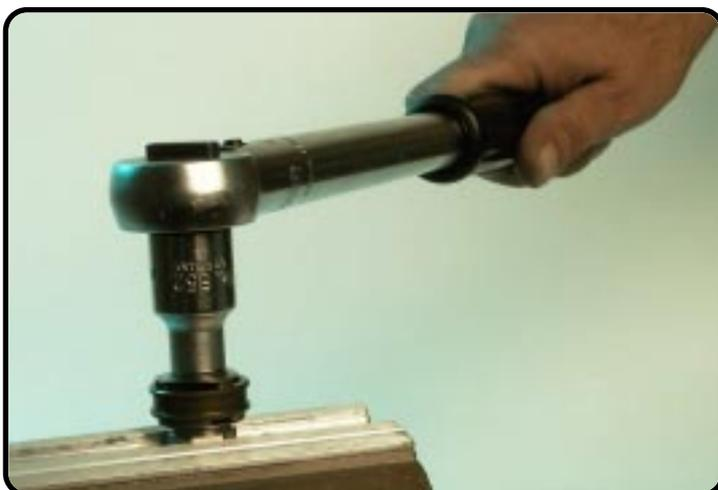
...tighten the nut to a torque of 5 Nm.
