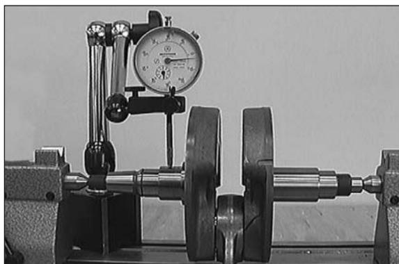
If the crankshaft will continue to be used, check the crankshaft journals for run out. Place the crankshaft on a roller block or a similar device and check the outer end of the journals for run out with a dial gauge.
