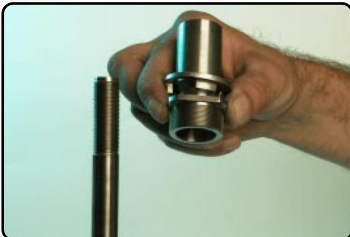
Remove the screw sleeve with spring retainer.
