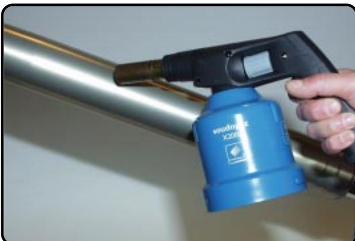
Heat the outer-tube at this level..
