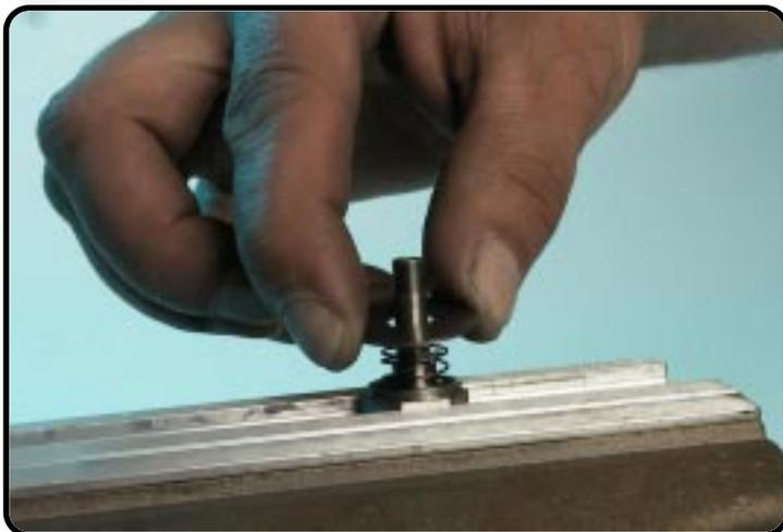
Assemble the spring and shims check-valve.
