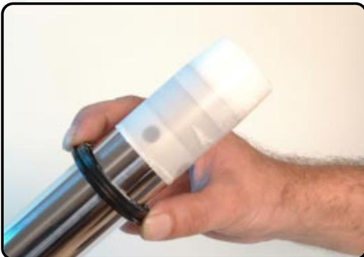
Place T1401 over the inner-tube and assemble the dust wiper.
