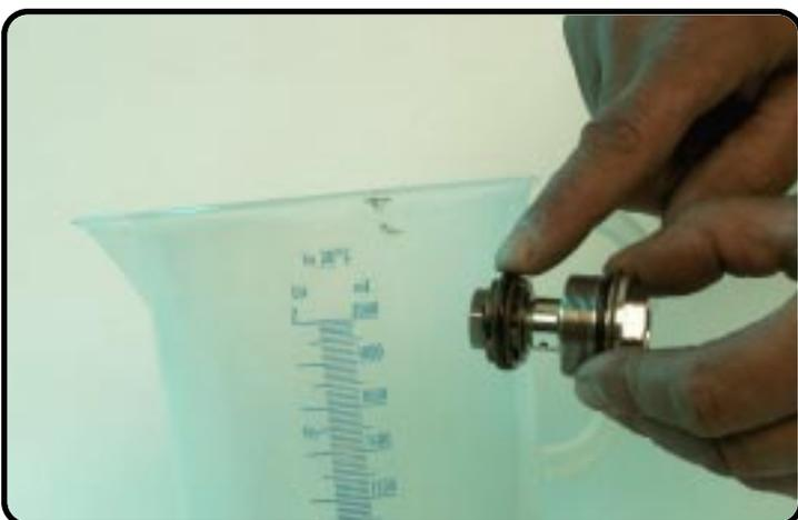
Apply the O-ring of the compression piston with frontfork oil.
