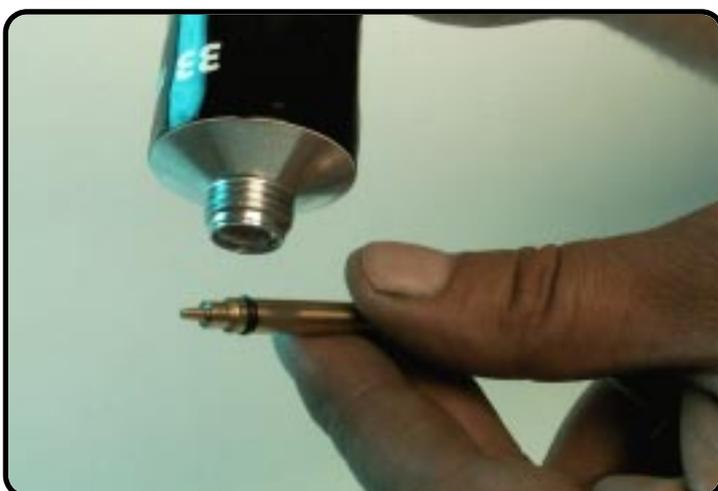
Grease the O-ring of the adjustment
