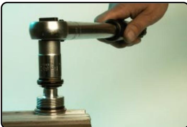
...to a torque of 5Nm.
