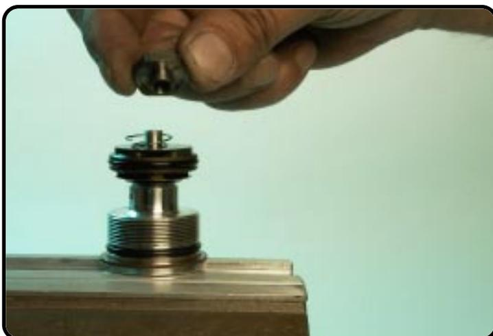
Remove the check-valve nut.
