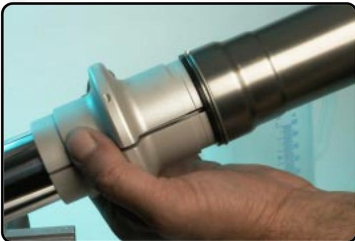
Assemble the dust wiper with T502S / T1402S.
