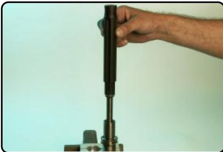
Clamp the piston rod in T508S “**not too tight**” and unscrew the hydraulic stop from the piston-rod.
