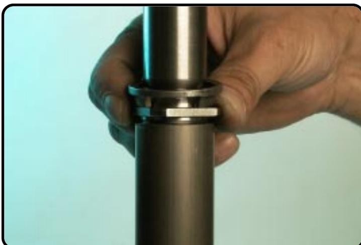
**Before assembling wet the thread of the screw sleeve with T131.**
