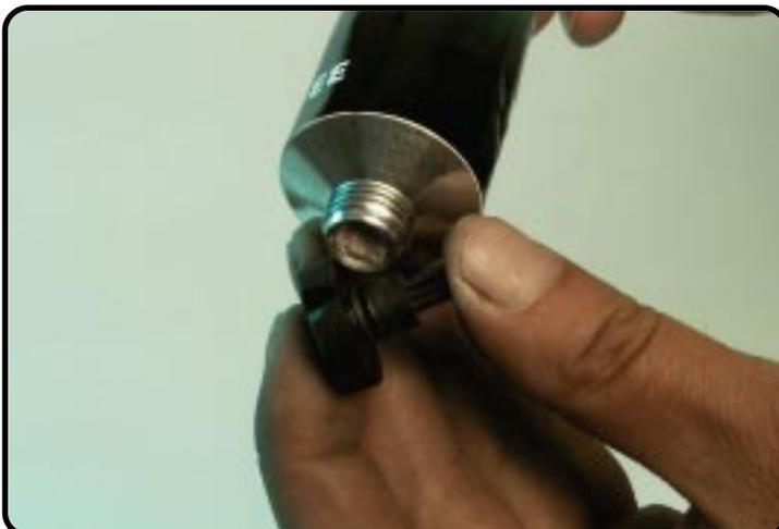
Grease the O-ring adjustment tube with T159.
