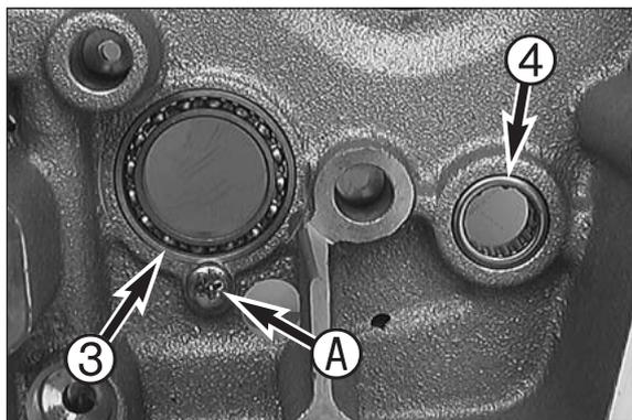
Grooved ball bearing of shift roller **3**
