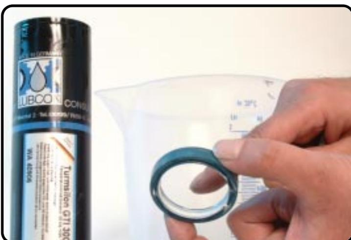
Apply the innerside of the oilseal with T511 and the outside with frontfork oil.
