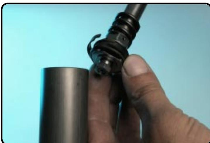
Disassemble the piston-rod "complete".
