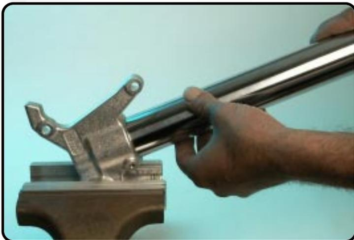
Assemble the inner-tube in the axle-clamp.
