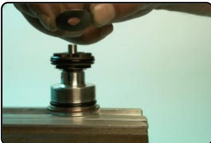
Remove the check-valve shim.
