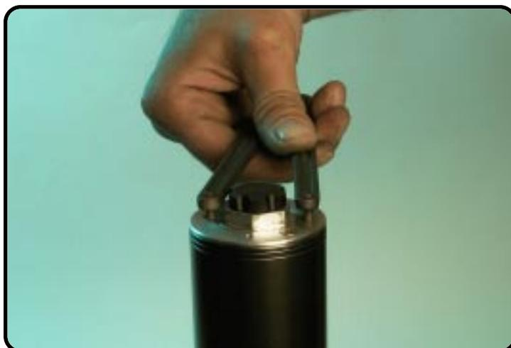
Tighten the screw-cap with T103.
