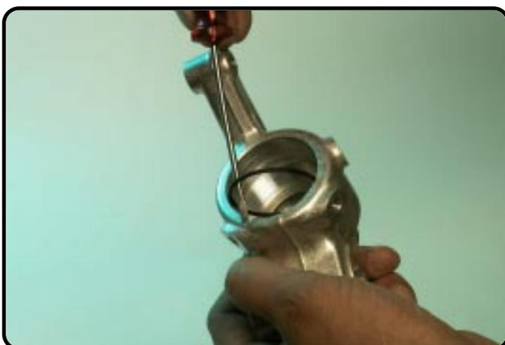
Remove the O-ring out the groove of the axle-clamp.
