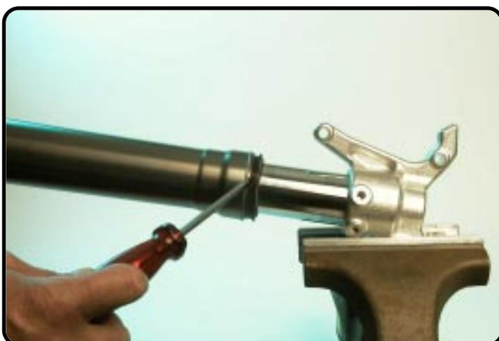
Disassemble the dust-wiper.
