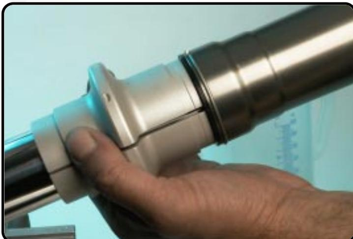
Assemble the dust wiper with T1402S.
