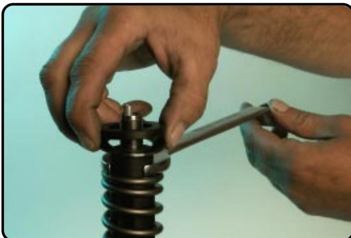
Replace first the steel washer on the spring, then the preload spacer(s).
