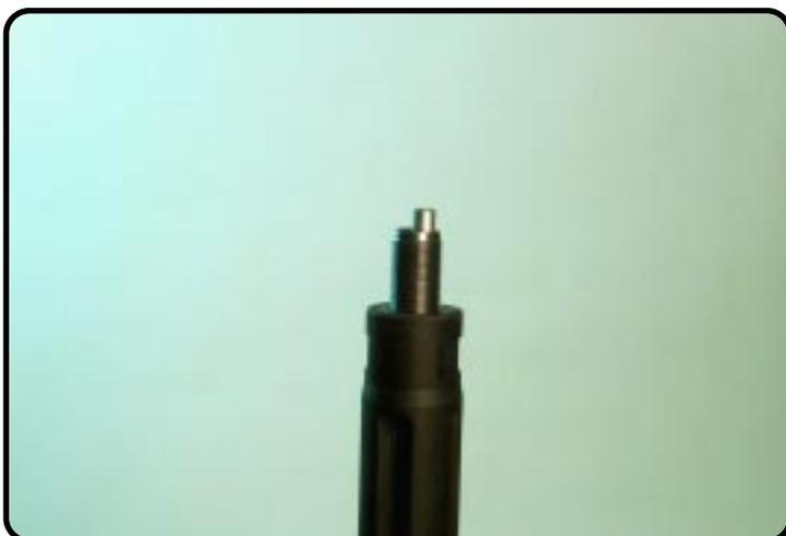
Assemble the adjustment tube with the O-ring into the piston-rod.
