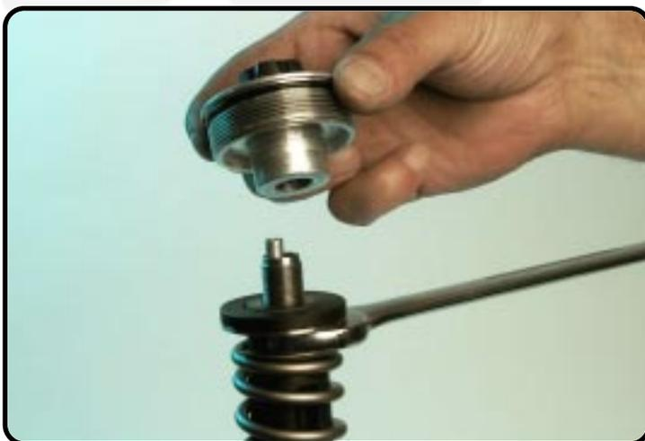
Remove the screw-cap from the piston-rod.
