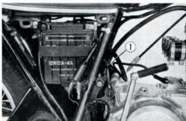
Fig. 53 ① Battery ground cable
