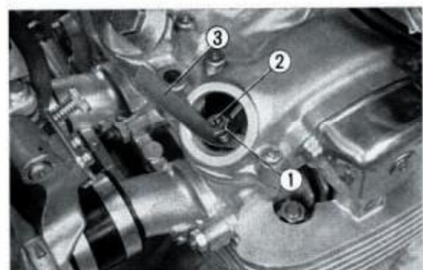
Fig. 3 ① Lock nut ③ Feeler gauge ② Adjusting screw
