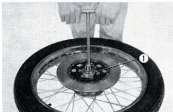
Fig. 197 ① Front wheel bearing retainer
