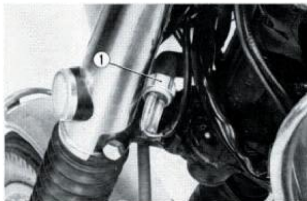
Fig. 309 Front stop switch inspection ① Front stop switch
