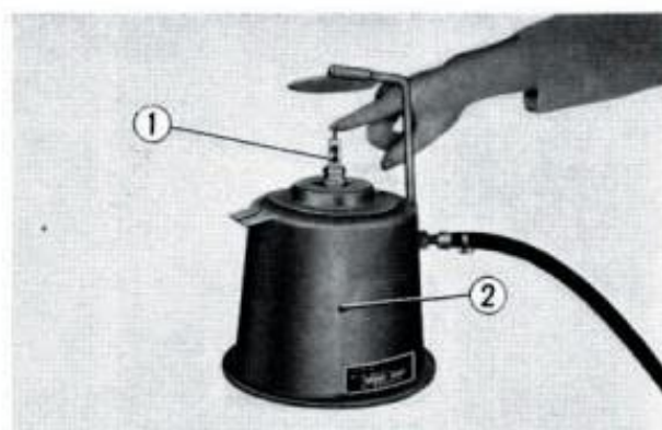
Fig. 275 ① Spark plug ② Spark plug cleaner
