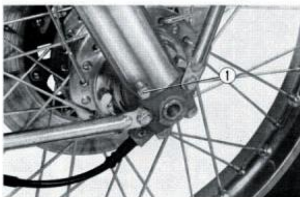
Fig. 41 ① Drain bolt
