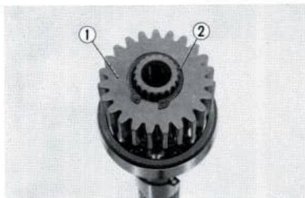
Fig. 159 ① Primary drive gear ② 20 mm snap ring
