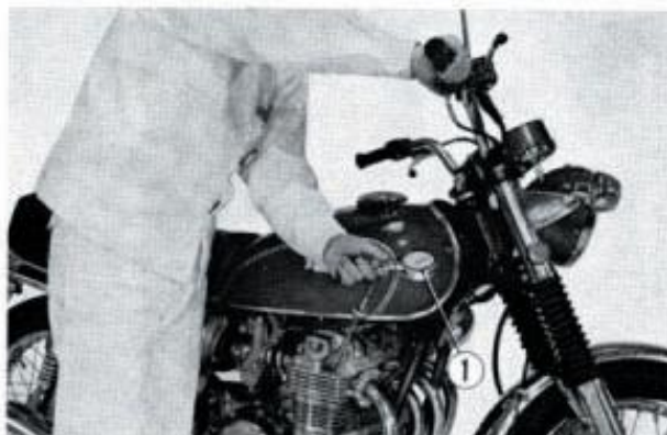
Fig. 42 ① Compression gauge
