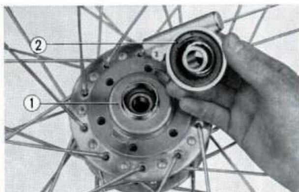
Fig. 205 ① Gear box retainer ② Speedometer gear box
