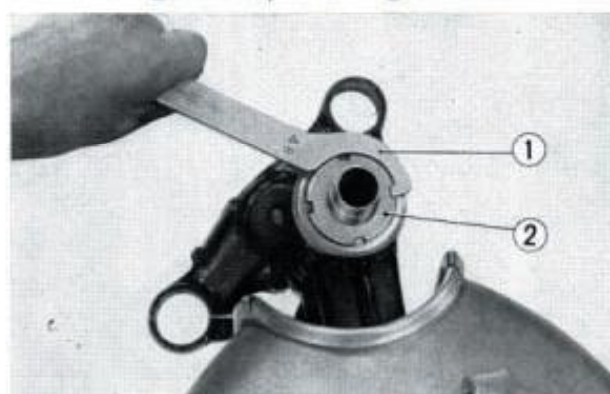
Fig. 240 ① Steering stem wrench ② Steering stem head nut
