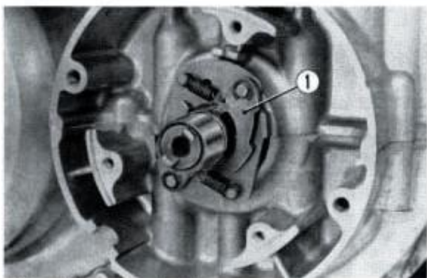
Fig. 279 ① Spark advancer
