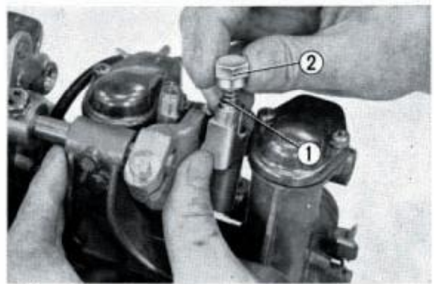
Fig. 191 ① Coil spring B ② Cap nut
