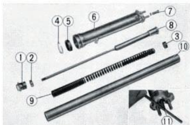
Fig. 249 ① Front fork bolt ② Lock nut ③ Cushion spring seat ④ Snap ring ⑤ Oil seal ⑥ Bottom case ⑦ 8mm bolt ⑧ Damper unit ⑨ Fork spring ⑩ Fork pipe ⑪ Special tool
