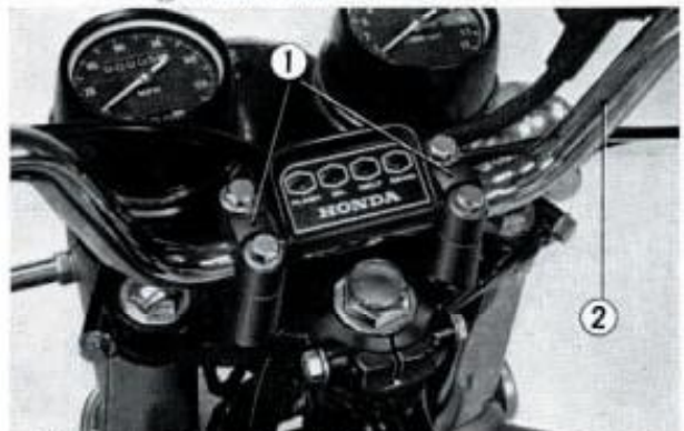
Fig. 238 ① Upper handle bar holders ② Handle bar
