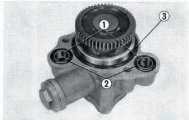
Fig. 108 ① O-ring collar ② 14 mm O-ring ③ 47 mm O-ring
