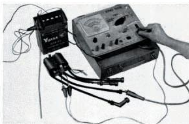
Fig. 273 Ignition coil performance test
