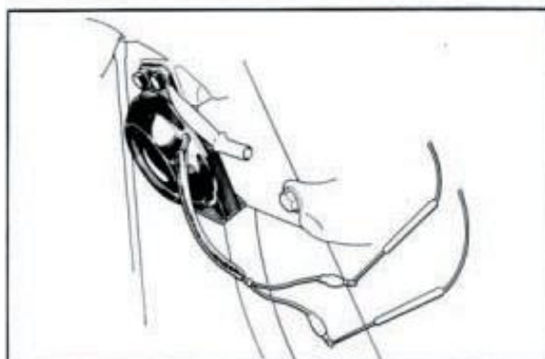
Fig. 311 Horn continuity test
