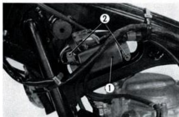
Fig. 271 ① Ignition coil ② Bolts
