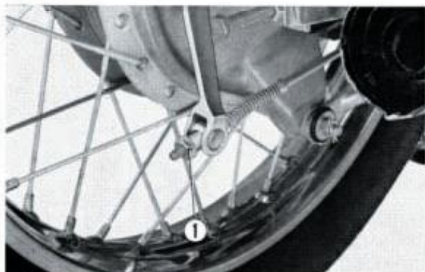
Fig. 235 ① Adjusting nut
