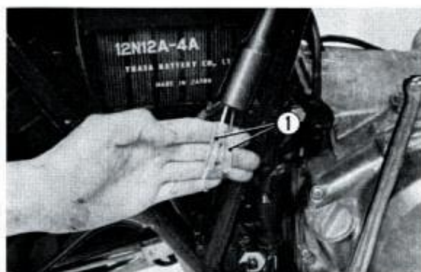
Fig. 50 ① Contact breaker point leads
