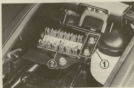
(1) ACC terminal (2) Fuse box
