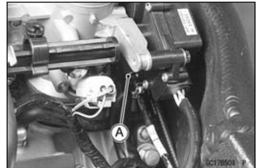
Main Throttle Sensor Connector [A]
