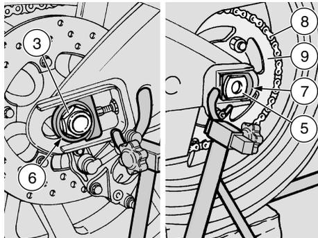
holder (15), do not overturn or rotate the rear wheel in horizontal position on the rear sprocket side (A), since the final drive unit would come off and fall down, with the risk of damaging the rear sprocket (9).
