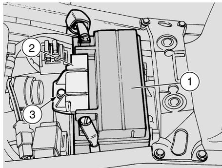
**NOTE** The battery (1) must be positioned in its compartment with the terminals directed towards the rear part of the vehicle.
