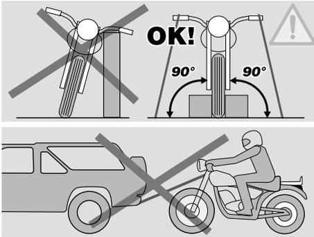
**NOTE** During transport, the vehicle must be kept in vertical position, it must be firmly anchored and the 1st gear must be engaged, in order to avoid any leak of fuel, oil, coolant.
