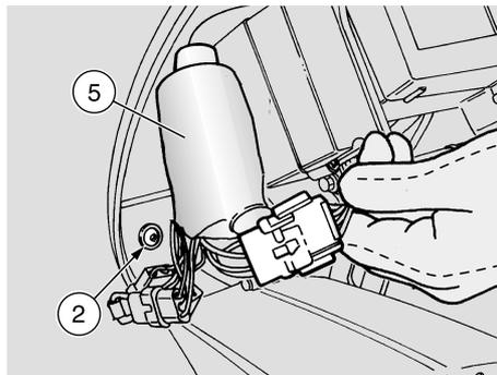
The whole unit must be correctly positioned on the support.
