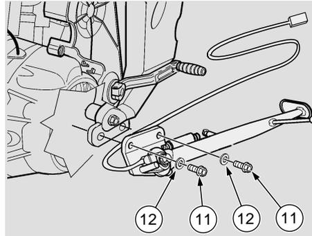
**NOTE** Store the following components together: complete stand, screws (11) and washers (12), in order to be able to install them correctly when the vehicle must be used on roads.
