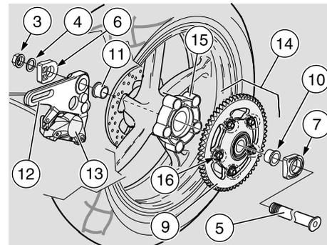
Wheel nut (3) driving torque: 120 Nm (12 kgm).
