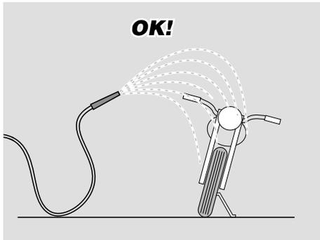
To remove dirt and mud from the painted surfaces use a low- pressure water jet, carefully wet the dirty parts, remove mud and filth with a soft car sponge impregnated with a lot of water and shampoo (2 – 4% parts of shampoo in water). Then rinse with plenty of water and dry with chamois leather.
