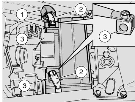
**NOTE** This vehicle is provided with a maintenance-free battery and no operation is necessary, excepting occasional checks and the recharge when required.
