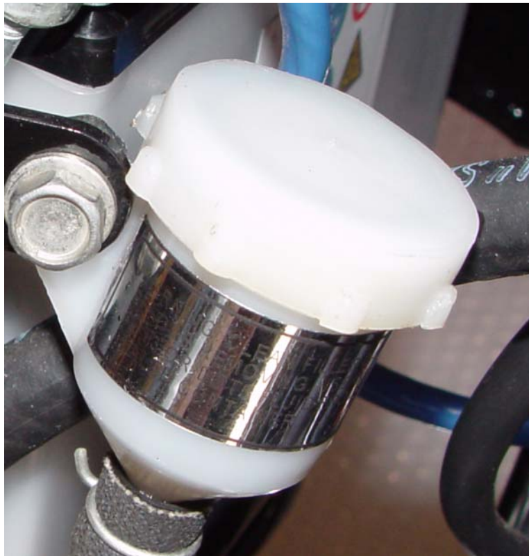
Rear Brake Hydraulic Reservoir
