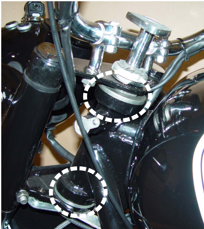
Steering Head Bearing Location
