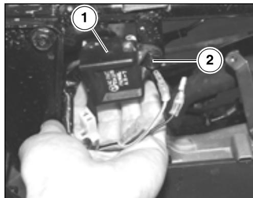
**6.1.14 REMOVING THE CONTROL UNIT**
