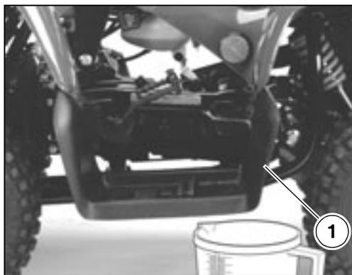
**2.12 CHECKING THE TRANSMISSION OIL LEVEL****DO NOT RELEASE OIL INTO THE ENVIRONMENT**
