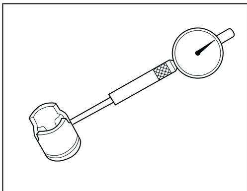
Check the diameter of the roller cage seat on the connecting link.
