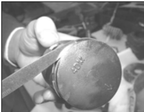
Measure the side clearance of the piston rings using a thickness gauge.
