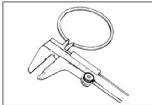
**PISTON RING-TO-GROOVE CLEARANCE INSPECTION**
