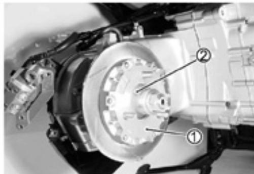
**T** Caliper mounting bolt: 25 N·m (2.5 kgf·m, 18.0 lb·ft)
