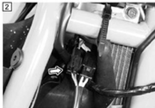
2) Crank the engine a few seconds with the starter motor, and measure the CKP sensor peak voltage at the coupler.
