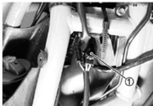
Measure the resistance between the three lead wires.
