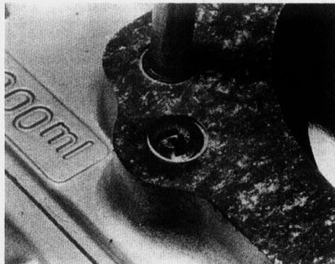
7.5 ...and the oil supply jets located on the edge of each crankcase mouth
