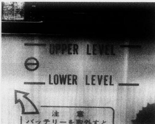
7.1 The battery electrolyte should be kept between the two level marks
