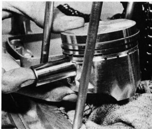
41.5b Lubricate the gudgeon pin before fitting
