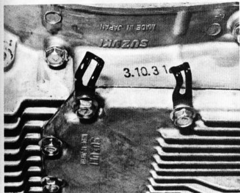
36.8b Correctly position the two electrical cable retaining clips beneath the bolt heads
