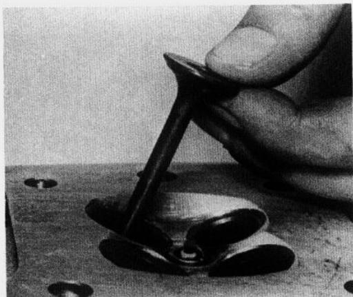
22.19b ...before lubricating and inserting the valve
