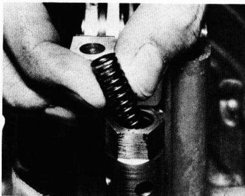
27.1c ...withdrawing the spring...
