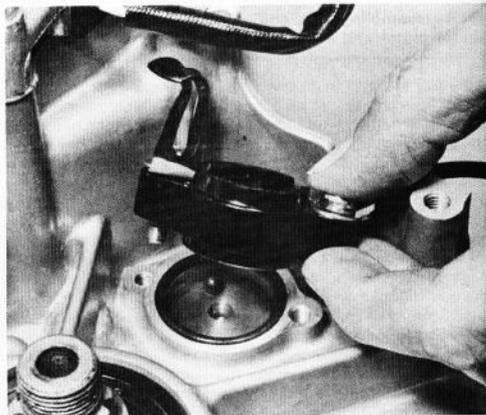
40.6 Do not omit to fit the neutral indicator (or gear position) switch contact pin and spring and a new O-ring
