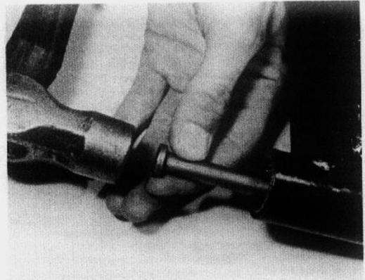
9.8b Use a length of steel rod to drift worn or damaged bearings from position...
