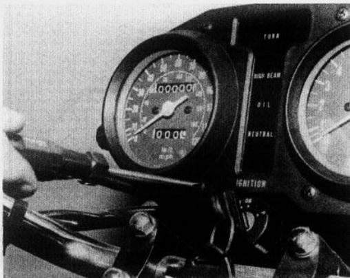
27.1a Remove the four securing screws...
