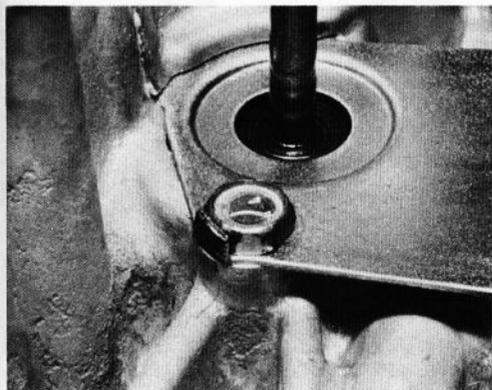
40.7 Lock the oil seal retaining plate bolts by bending up the plate tabs as shown
