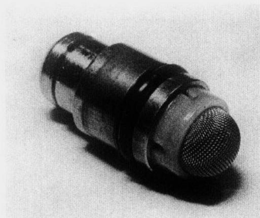
6.12b ...whilst checking that the filter attached to the seating is clean
