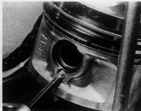
7.7 Prise each gudgeon pin circlip from position
