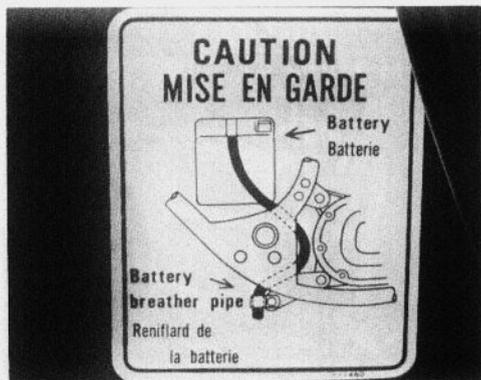
Note the instructions for routing the battery vent pipe
