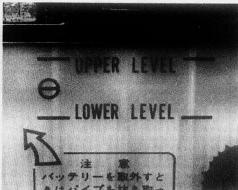
Keep the battery electrolyte level between the level marks
