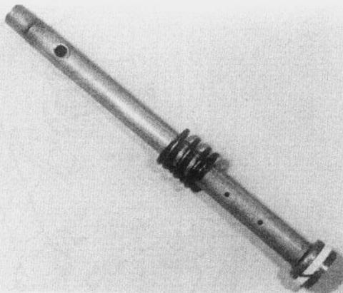
4.8 Inspect the damper rod assembly for ring and spring wear
