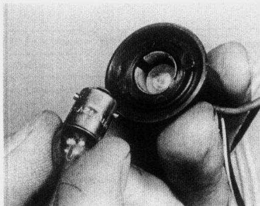
31.2d The pilot bulb is a bayonet fitting in its holder
