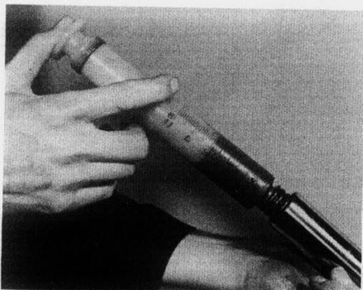
4.14b Remove the cap bolt to allow replenishment of the fork leg oil
