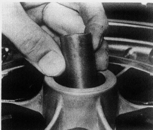
12.5b ...grease and insert the bearing spacer...
