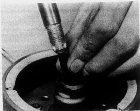
8.6b ...before inserting a dowel spacer...
