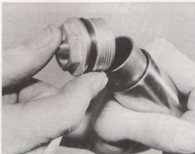
5.1a Remove fork top bolt ...
