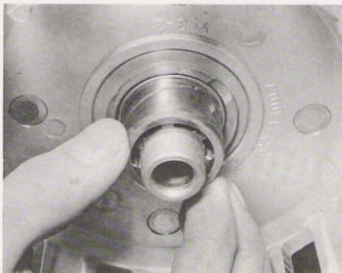
32.3e ... and the inner bush fitted
