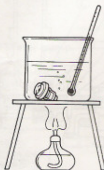
Fig. 2.5 Thermostat operation
