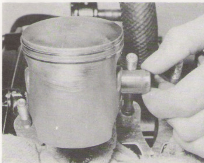
6.7b Gudgeon pins can now be displaced to allow the pistons to be lifted away
