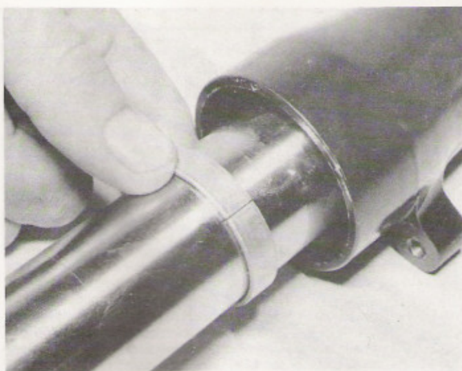
5.8a Lubricate top bush and slide into place
