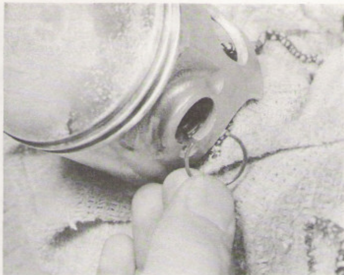
34.4a Use new circlips to secure the gudgeon pins ...
