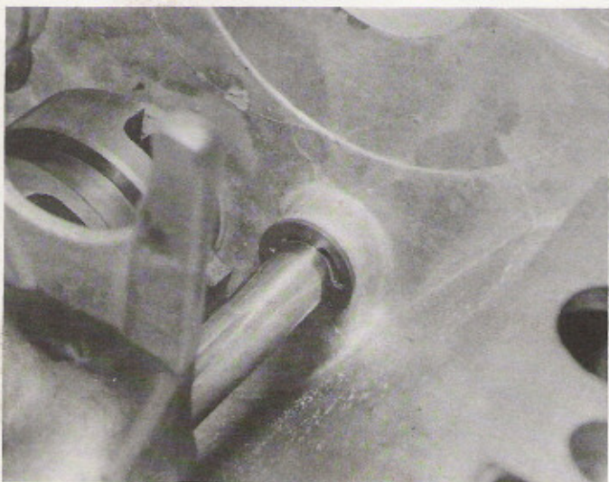
12.4a Release the circlips which retain the selector fork shafts ...
