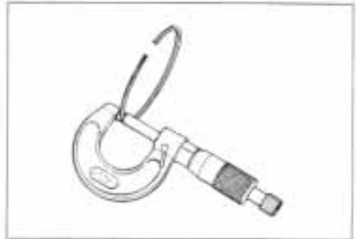
**PISTON RING FREE END GAP AND PISTON RING END GAP**
