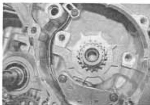
**CAMSHAFT POSITION SENSOR (CMP SENSOR)**
