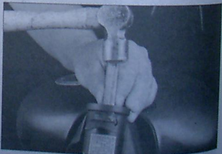
7.16 Drive the lower bearing top race out from above; drive the upper bearing bottom race out from below
