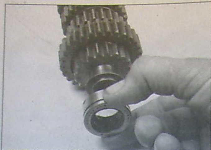
29.3b Remove the bearing and snap-ring from the end of the shaft
