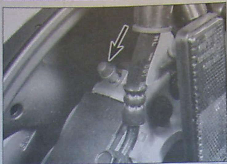
8.6a Each front caliper has a single bleed valve (arrow) ...
