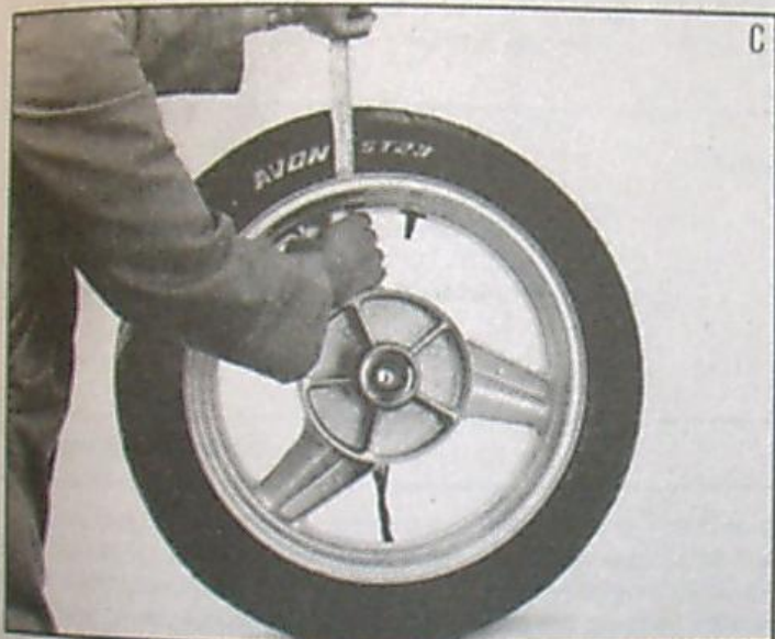
When first bead is clear, remove tire as shown.
