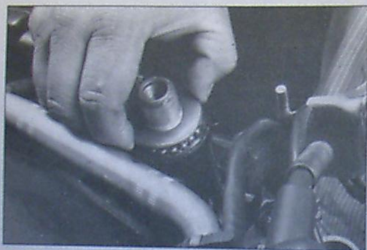
7.12b ... and the upper bearing top race, taking care not to let the bearing balls drop out...
