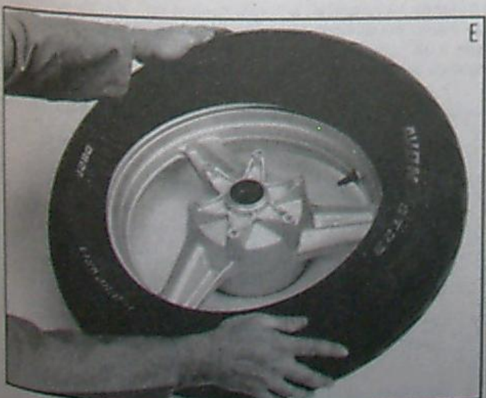
Work first bead over the rim flange.
