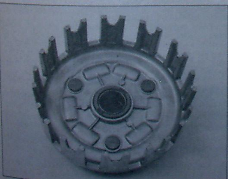
19.10 Slide the clutch boss off and remove the thrust washer
