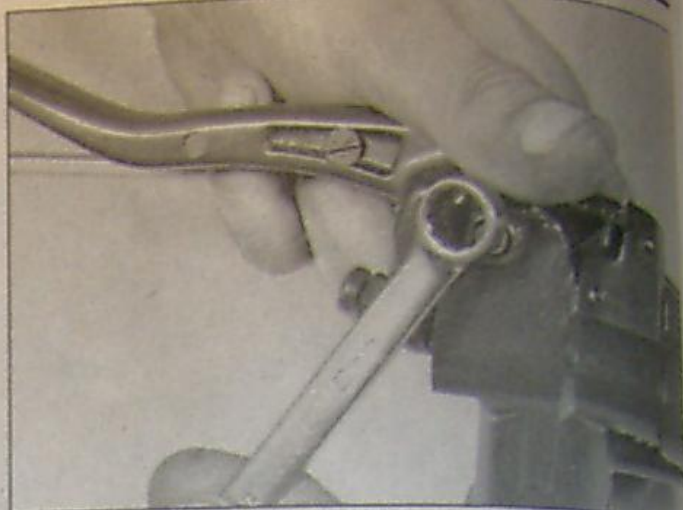
5.6 Remove the locknut and pivot bolt (master cylinder removed for clarity)
