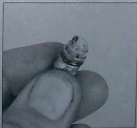
7.6c This is the typical type of debris found on the needle and seat filter screen
