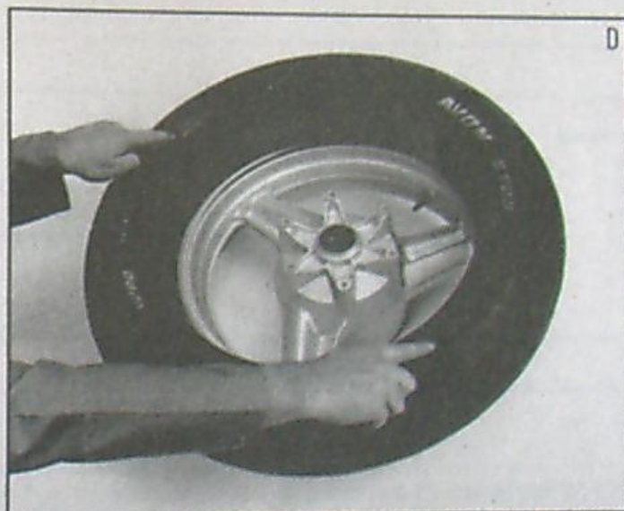
Before installing, ensure that tire is suitable for wheel. Take note of any sidewall markings such as direction of rotation arrows.
