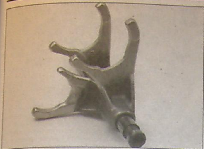
30.3 Reassemble the forks onto the guide bar so they don't get mixed up; the number on each fork faces the right side of the engine when the forks are installed
