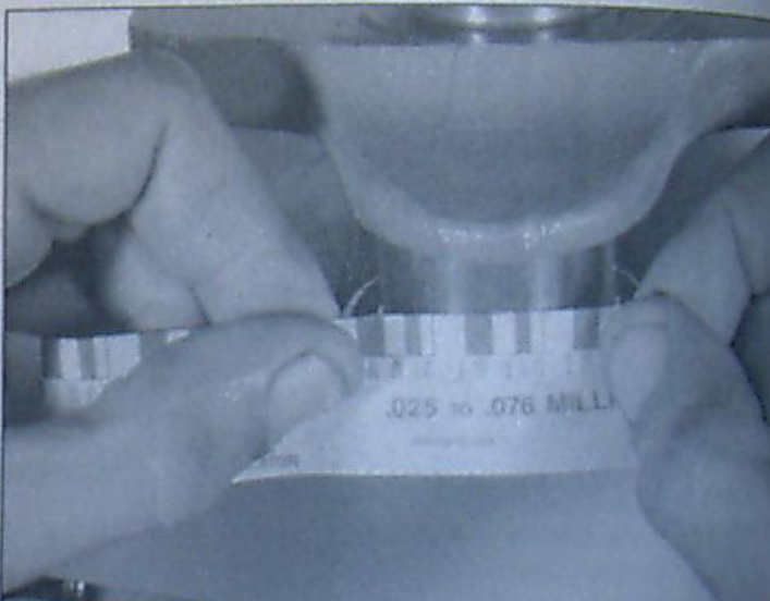
26.13 Place the Plastigage scale next to the flattened Plastigage to measure the bearing clearance
