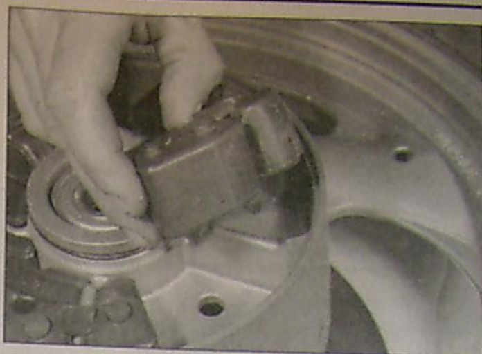
15.3 Lift out the rubber damper segments
