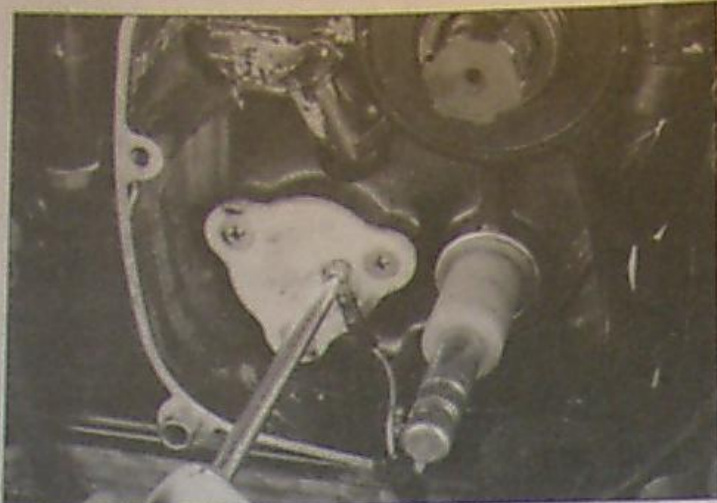
19.6 Remove the small screw and disconnect the wires, then remove three larger screws and remove the switch
