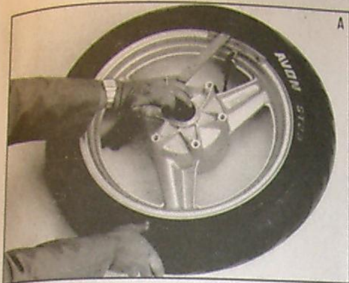
Deflate tire. After releasing beads, push tire bead into well of rim at point opposite valve. Insert lever next to valve and work bead over edge of rim.
