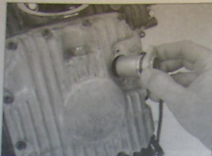
15.3 Remove the bolts and pull the oil level sender out of the oil pan; use a new O-ring for installation
