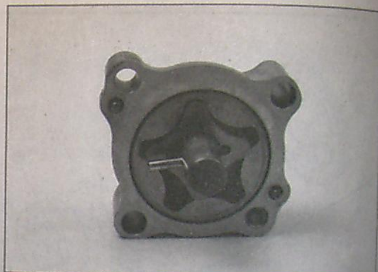
17.16 Insert the pin in the shaft and make sure it's centered
