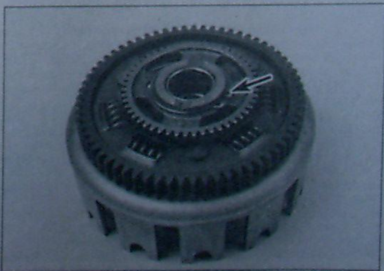
19.11 Remove the snap-ring (arrow) and take off the oil pump drive gear
