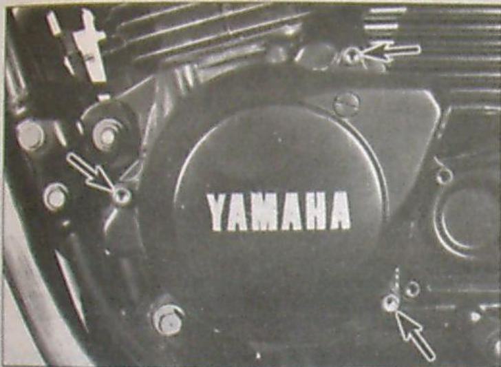
18.10 On later models, remove the Allen bolts (arrows) and remove the alternator cover...
