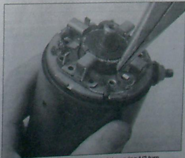
25.14b . . . then pull the end of the spring 1/2 turn counterclockwise (anti-clockwise) and seat the end of it in the groove in the end of the brush
