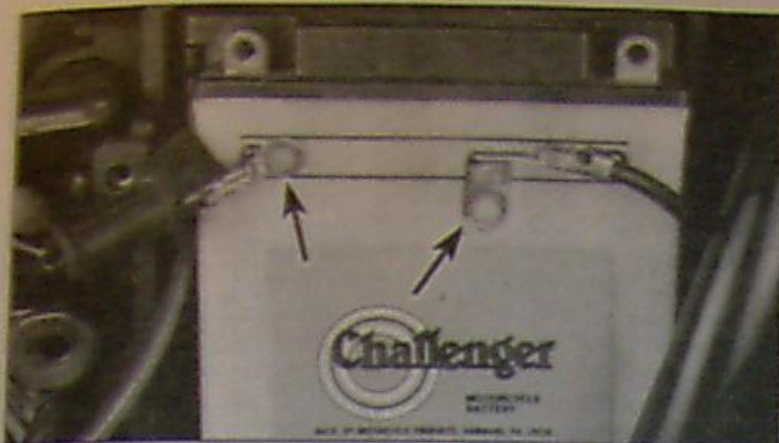
4.4 Detach the negative cable (right arrow) from the battery first, then detach the positive cable (left arrow); the plastic cap protects the positive terminal from accidental contact with metal
