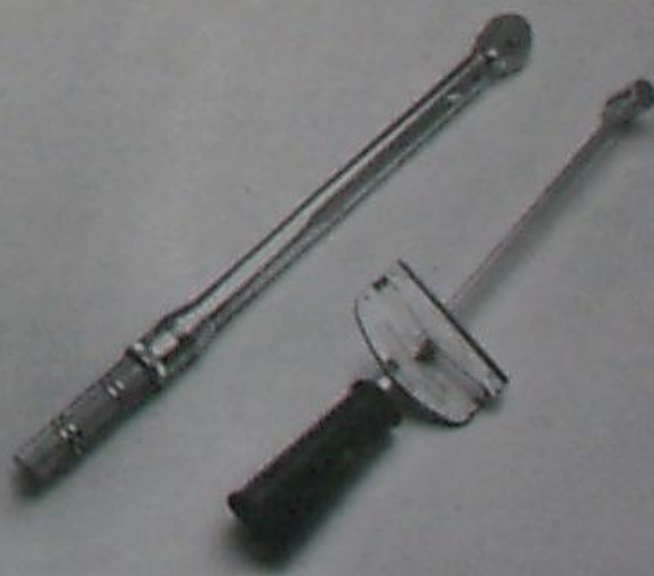
Torque wrenches (left - click type; right - beam type)
