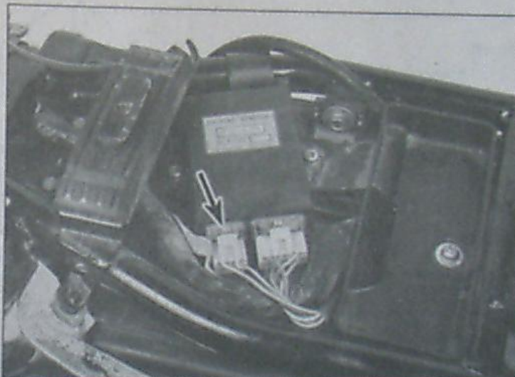
4.2 Disconnect the four-terminal connector from the igniter (YX600 Radian shown)
