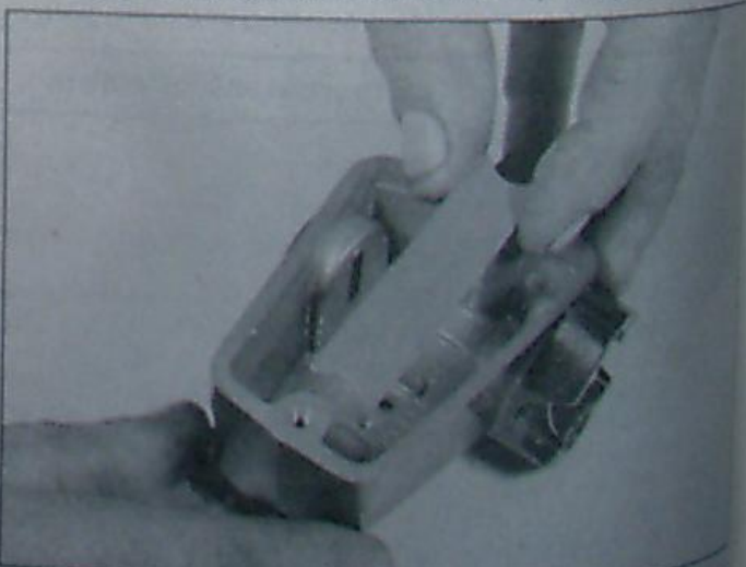
5.8 Lift the splash plate (if equipped) out of the cylinder body so you can clean the fluid ports in the bottom
