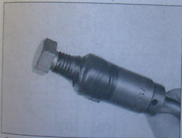
6.4e ... then install the nut-end into a socket (connected to a long extension) and tape it into place
