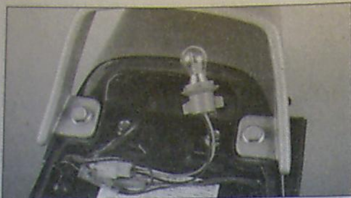
9.8a To replace taillight bulbs on YX600 Radian models, reach inside the tail cowl, turn the bulb socket counterclockwise (anti-clockwise) and pull it out . . .
