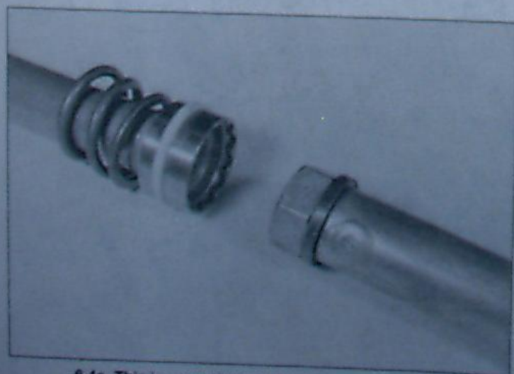
6.4a This is a special tool that's used to hold the damper rod from turning
