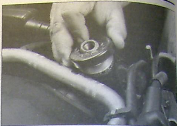
7.12a Lift off the bearing cover...
