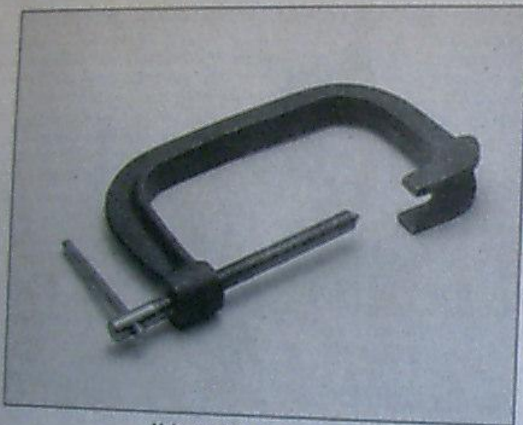
Valve spring compressor
