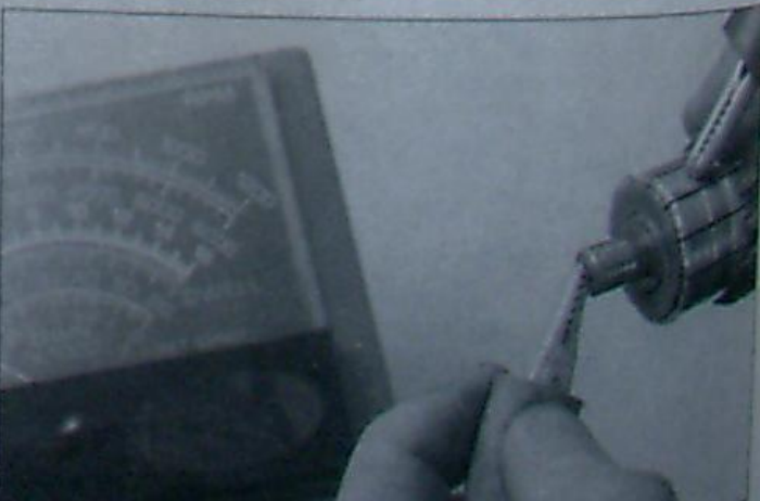
25.8b There should be no continuity between the commutator bars and the armature shaft
