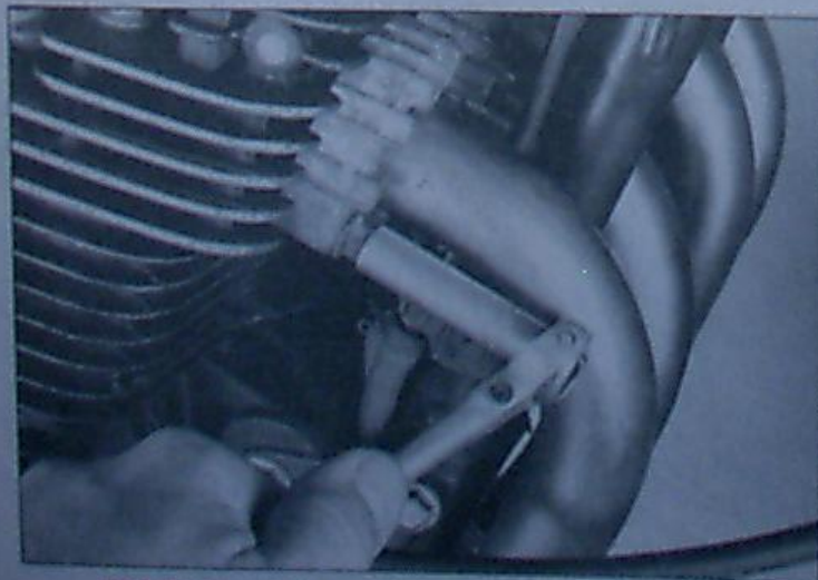
12.8 Remove the mounting nuts at the cylinder head
