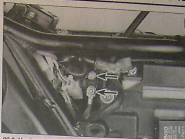
23.3 Unplug the wiring connector, then remove the nuts (arrows) and disconnect the cables ...
