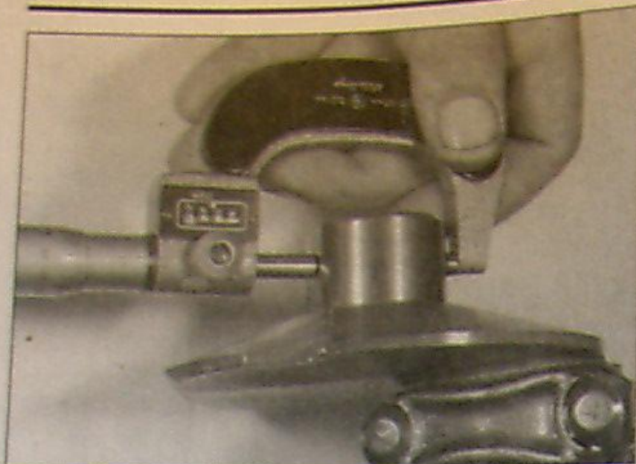
25.14 Measure the diameter of each crankshaft journal at several points to detect taper and out-of-round conditions
