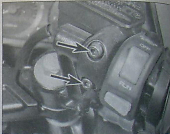
5.7 Remove the master cylinder mounting bolts
