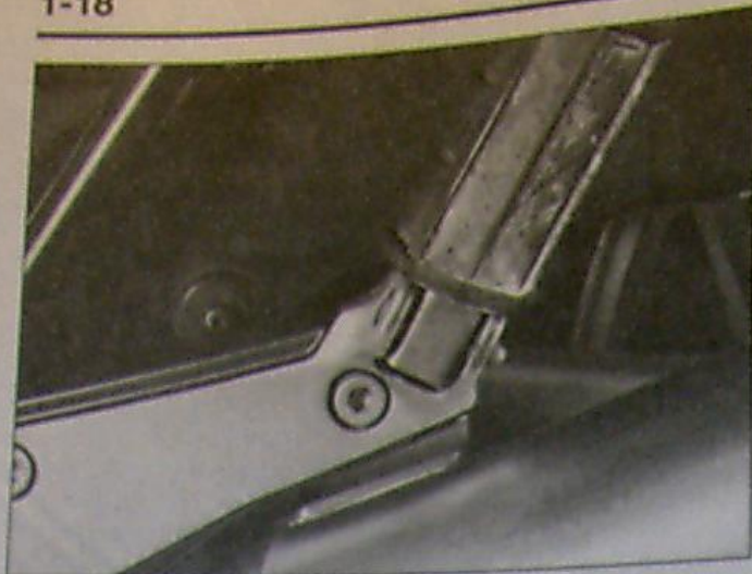
17.2b Lubricate the rear footpegs at their pivot points
