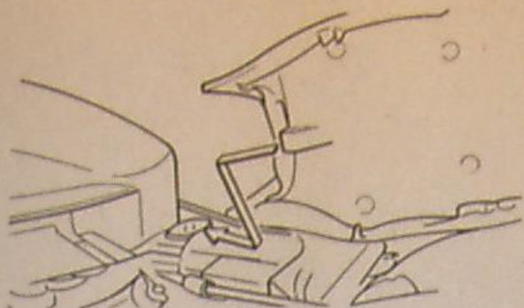
2.5 Disengage the tab at the front of the seat
