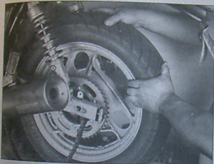
13.8 Pull the rear wheel out, taking care not to lose the collar on each side of the wheel
