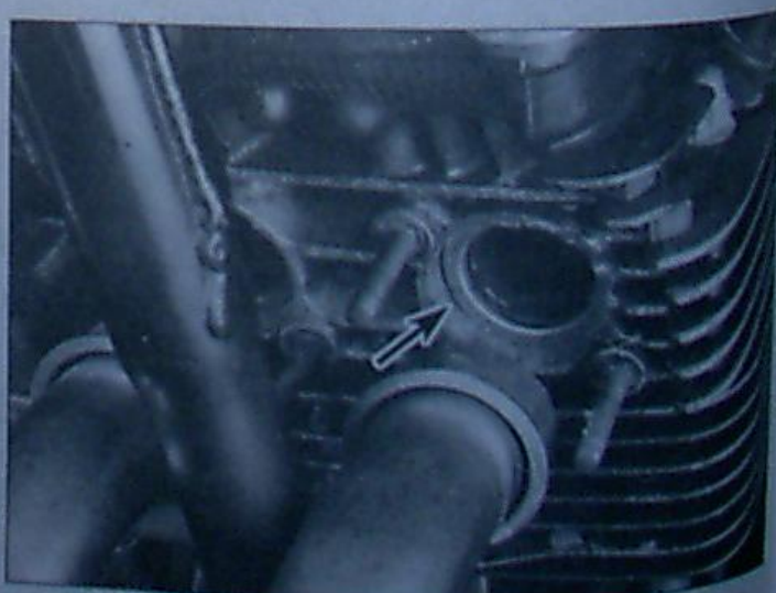
12.9 Always replace the copper gaskets when reconnecting the exhaust pipes to the cylinder head
