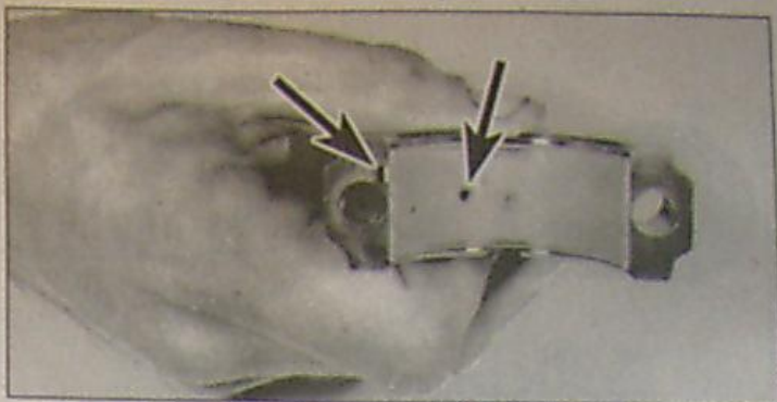
26.20 Be sure the tab fits in the notch and the oil hole in the upper bearing aligns with the hole in the connecting rod (arrows)
