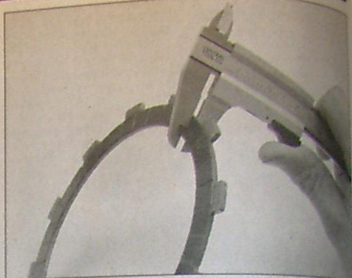
19.14 Measure the thickness of the friction plates
