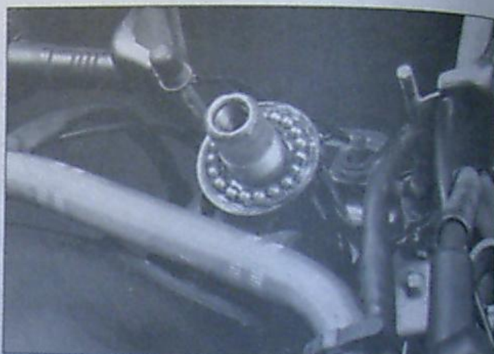
7.12c ... and remove the bearing balls
