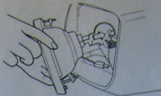
7.1b ... and pull the assembly out
