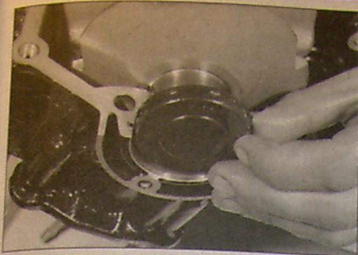
22.15 Make sure the blind plug is in place before assembling the crankcase
