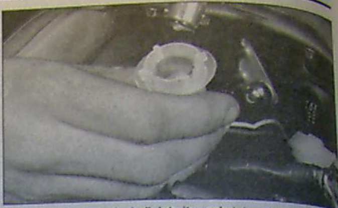
9.8b . . . then push the bulb into its socket, turn counterclockwise (anti-clockwise) and pull it out
