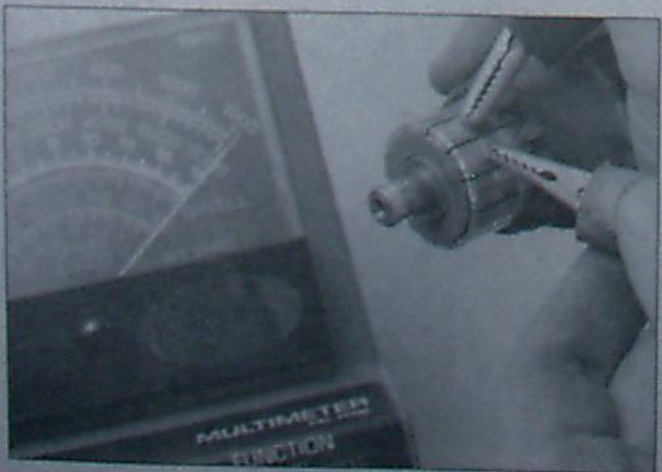
25.8a Continuity should exist between the commutator bars
