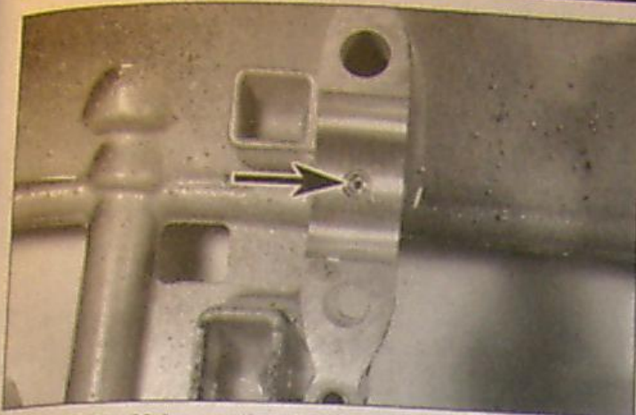
25.17a Make sure the oil holes are clear (arrow) ...
