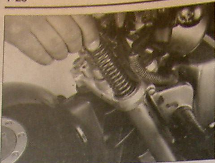
27.13 Remove the spring; it will retain a little left-over oil when it's pulled out, so have a rag handy to catch the drips
