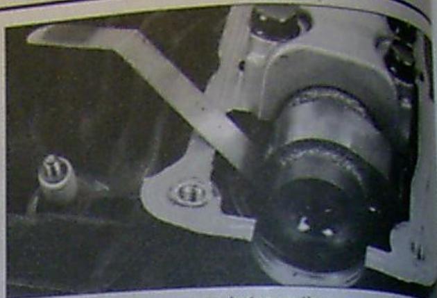
18.13 Slip a feeler gauge between the cam lobe and valve adjusting shim - it should pull out with a very light drag
