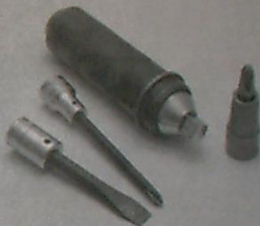
Hand impact screwdriver and bits
