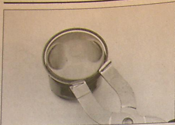
14.6 Remove the piston rings with a ring removal and installation tool
