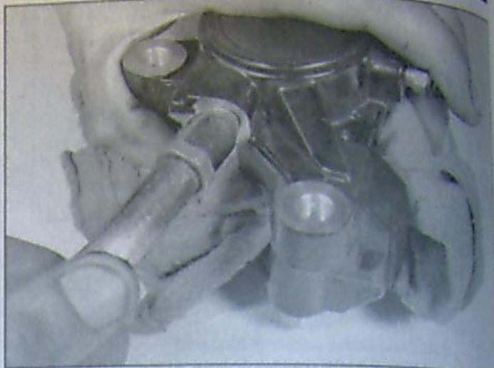
3.6 Blow air into the bleed valve hole to force the pistons out, but DO NOT get your fingers in the way
