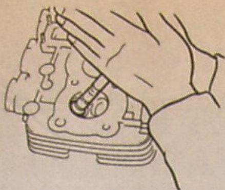
12.24a After lapping, the valve face should exhibit a uniform, unbroken pattern . . .
