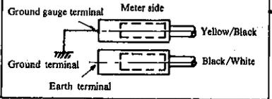
Meter pointer fails to move → Meter side defective → Check (5)
