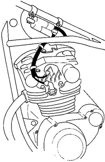
How to set contact breaker lead wire
