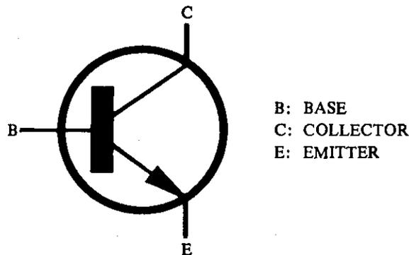
Each transistor has three terminals identified as the Base (B), Collector (C), and Emitter (E), and operation is as follows:
