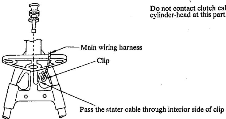
Do not contact clutch cable and cylinder-head at this part.
