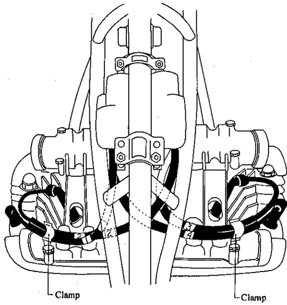
How to set contact breaker lead wire.
