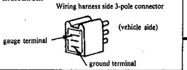
Meter pointer swings to extreme position → Connector contact defective
