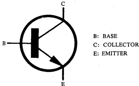
Each transistor has three terminals identified as the Base (B), Collector (C), and Emitter (E), and operation is as follows:
