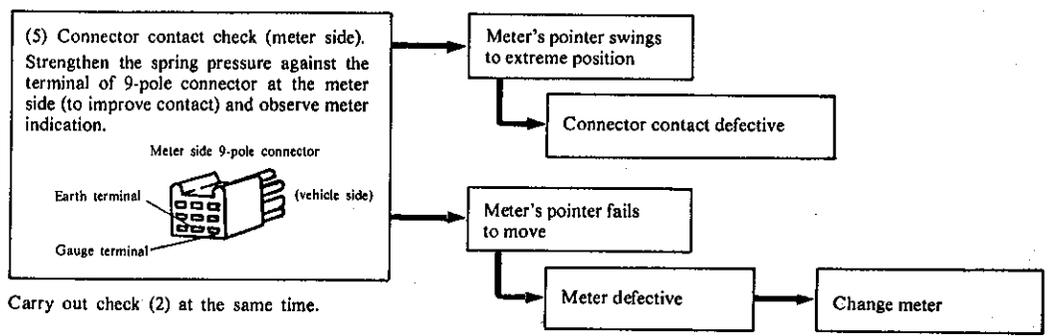
Meter's pointer swings to extreme position and indicates plus.
