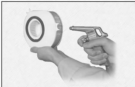
3. Lightly tap the air filter element to remove most of the dust and dirt, and then blow the remaining dirt out with compressed air as shown. If the air filter element is damaged, replace it.
