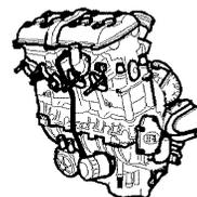
Install the intake camshaft with the timing notch of the drive gear parallel to the head table, facing outside (see picture).
