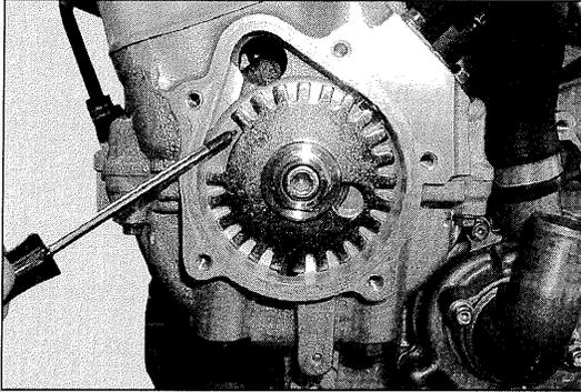
In this position the "T" notch on the phonic wheel is aligned with the notch on the crankcase.
