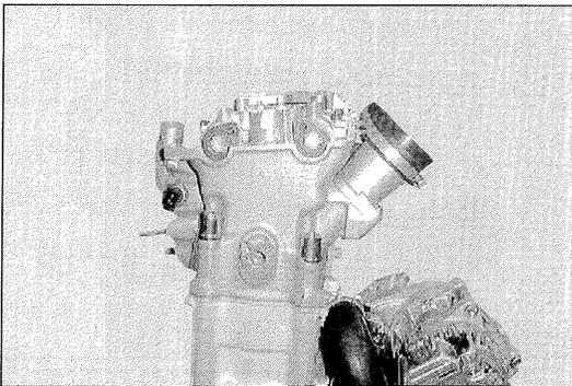
The N°1 cylinder cams converge to the top symmetrically as shown in picture. The notches on the camshafts control gears are horizontal and face outwards.
