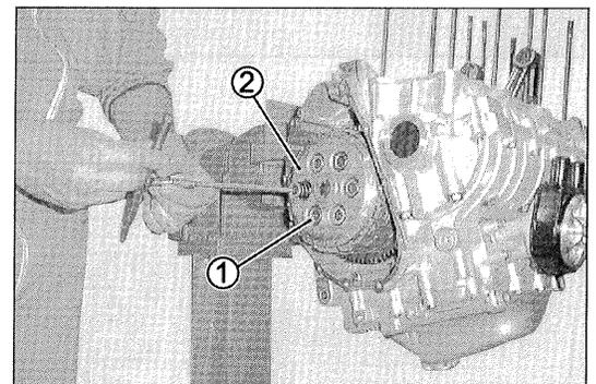
Remove the clutch spring plate.
