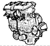
First remove the external camshafts U-bolts (4 - 5) by acting on the 4 socket head screws of each one.
