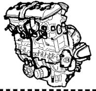
Install the gear group in gear in the crankcase to avoid any damage to the neutral switch light.
