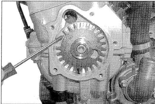
Rotate the camshaft until the n°1 piston reaches the TDC, using a 19 socket wrench on the phonic wheel nut.
