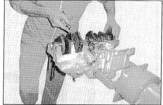
Install the bearings on the lower crankcase with the stoppers facing each other and inside the crankcase.
