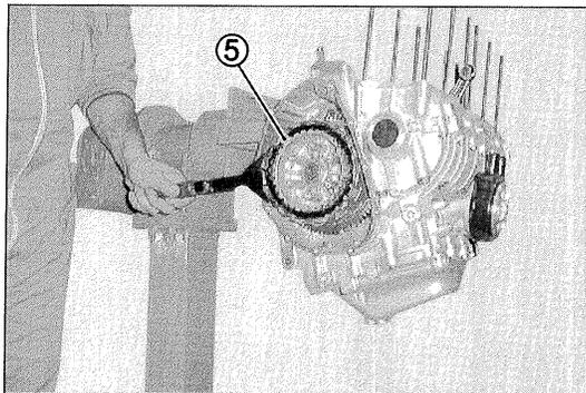
Remove the nut using the n° 79015 tool to stop the clutch hub (5).
