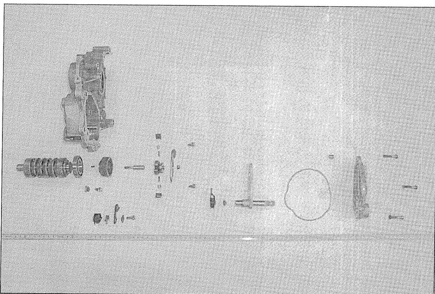
Verify the gear locker pawl free movement. Reassemble the various parts by acting in the opposite way.
