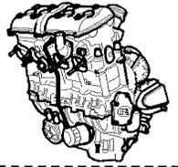
The clutch disengagement is obtained with a transmission group made of a thrust piston on the engine left side, with hydraulic drive. This piston pushes a rod controlling the clutch spring plate
