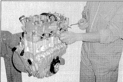
Withdraw the central screw of the timing system chain tensioner. Remove the chain tensioner by acting on the 2 fixing screws.
