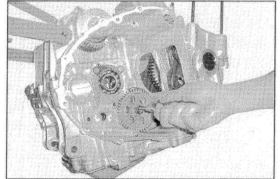
Perform an accurate visual check of the parts to find signs of scoring or deformation
