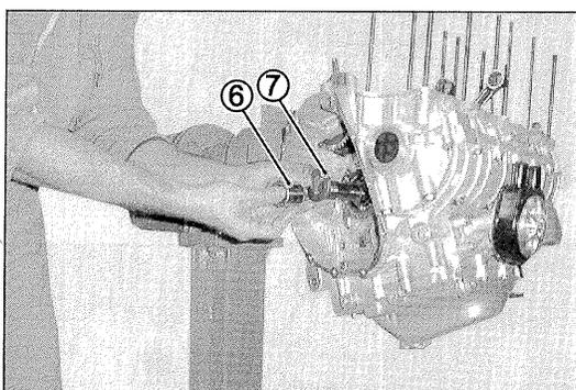
Remove the clutch group, the spacer (6) and the shim adjustment washer (7)
