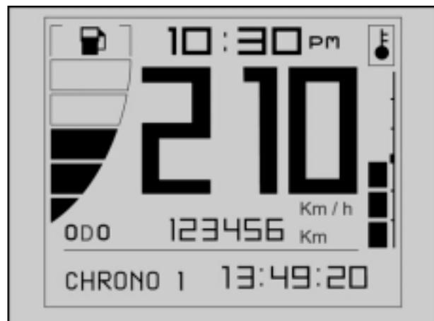
Press again the MODE selector to the centre position after 10 seconds have elapsed from timer start, time measurement is interrupted, stored and a new one is started. Press the MODE selector for a certain time to the centre position to interrupt lap time set.
