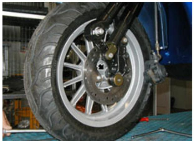
If necessary the front shock absorbers can now be removed.
