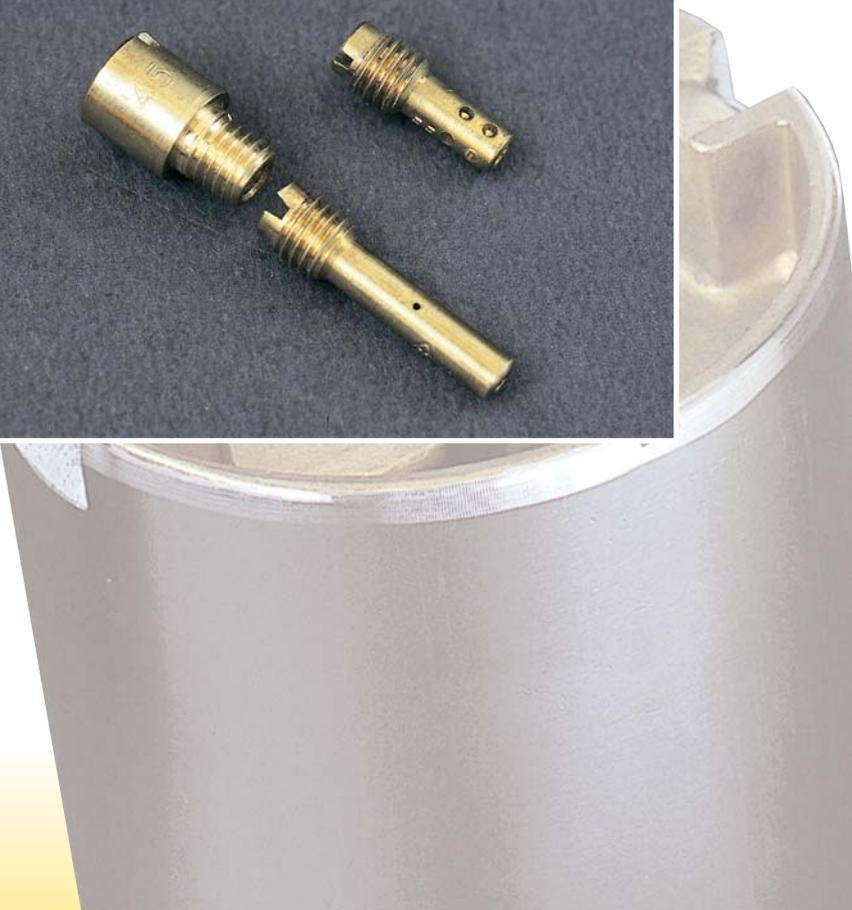
On the left, the idle jet, whether or not connected to a diffuser, is often screwed inside the emulsion tube and not outside as is common in other versions of carburetors.
