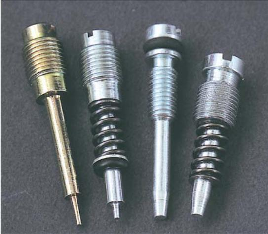
On the right, the air adjustment screws (the two on the left) have a smaller point than the mixture screws (on the right) since they are required to control a different fluid and therefore allow a finer adjustment. By controlling the air, this system has its own influence on the progression circuit, while the mixture screw acts only on the idle delivery.
