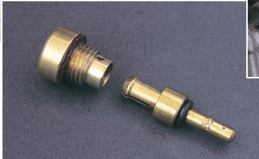
*Above, the nozzle spraying fuel into the venturi is controlled by a calibrated hole machined into the body of the nozzle itself. This component is kept in the seat by a plug (cap), therefore in Dell'Orto's carburetors it is easy to reach from the outside.*
