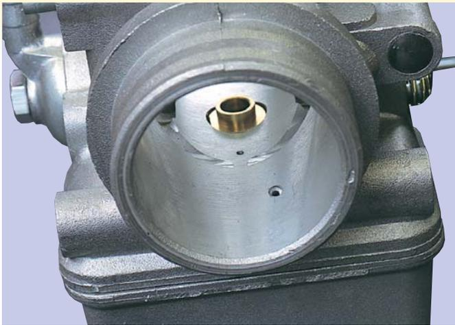
Above are two details of the supply ports of the idle and progression circuits, which can be seen slightly downstream of the main spray nozzle.
