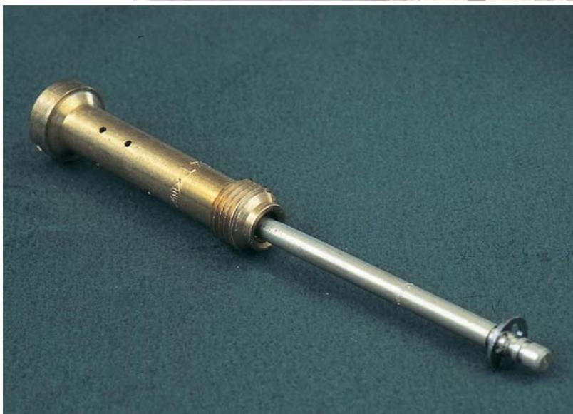
*Above, the group of main and starting jets inside the float chamber. We can note the baffle that keeps fuel in the chamber of the main jet even when the motorcycle is subjected to acceleration that would tend to move the liquid mass in the float chamber. Below, the conical needle and atomizer placed in their relative working positions.*
