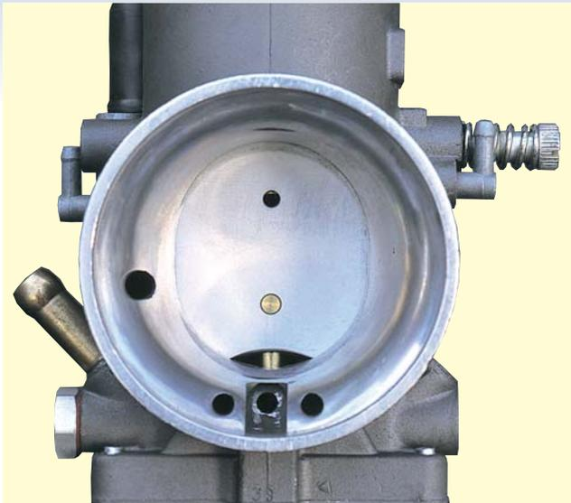
The throttle valve of "needle" carburetors has a chamfered edge (measured in tenths of mm: for example, .30) which influences the carburation at small throttle openings. A valve with low chamfer (as above) enriches the mixture up to 1/4 throttle, while if the carburation is too rich, we can use a valve with a higher chamfer (as below).
