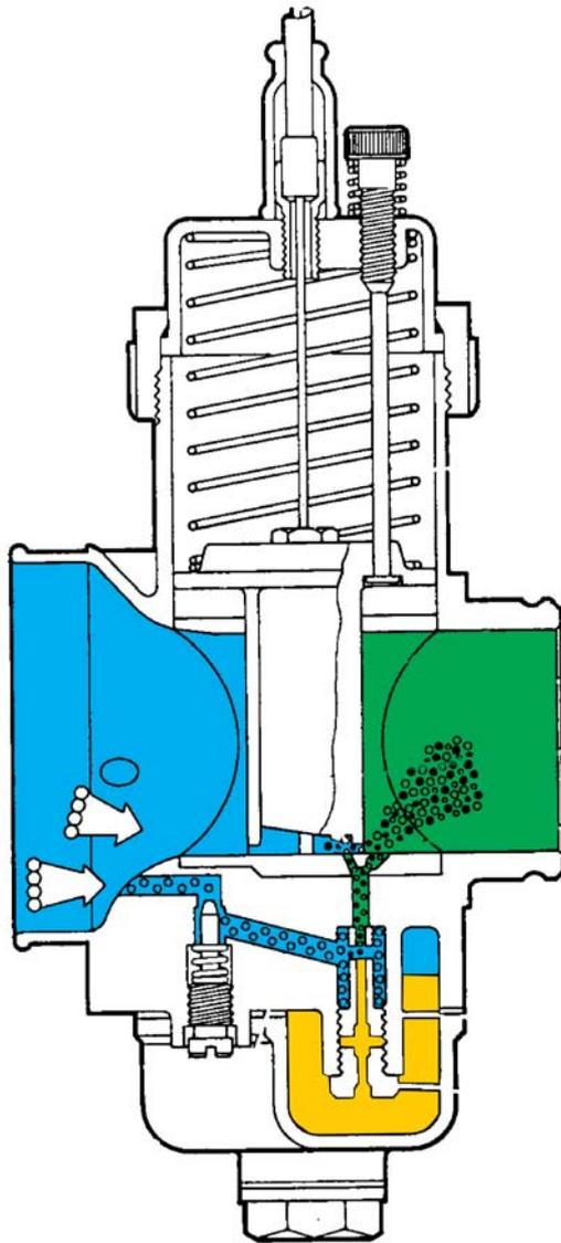
port. This progression port is placed upstream of the rear edge of the valve, just before the idle port (with respect to the direction of the airflow in the diffuser).
