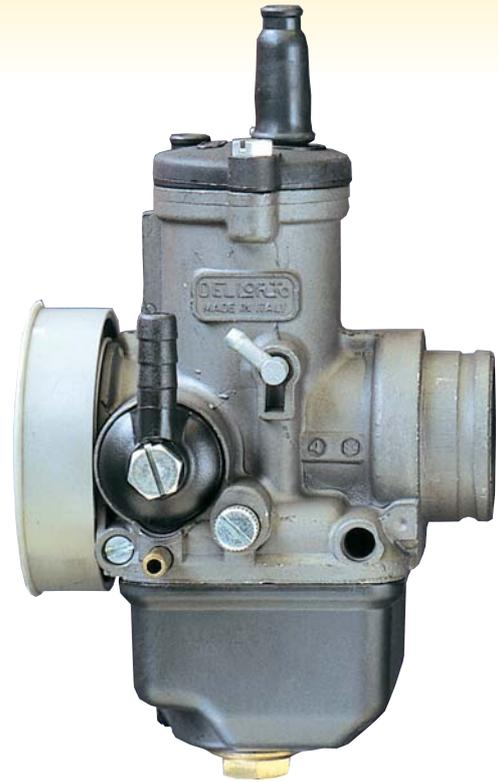
tor is equipped. To enrich we have to close the air screw (by closing the airflow) or open the mixture screw. To lean the mixture, one has to open the air screw or close the mixture screw.
