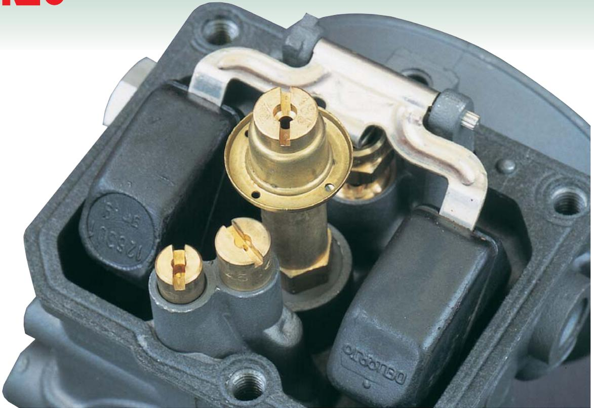
That is why the system with a conical needle has been adopted, with a configuration well known to everyone and clearly visible in the illustrations. The needle runs inside the metering section of the atomizer, and when the valve is lifted only slightly, the passage available for the fuel is small.
