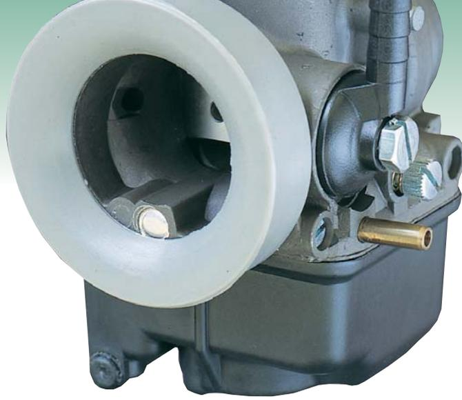
*To eliminate the influence of pressure pulses present in the filter box, sometimes the main emulsion air inlet is drawn from the outside by means of a connection in which we see the feed tube on the right of the carburetor. In this case the hole in the air intake is plugged.*
