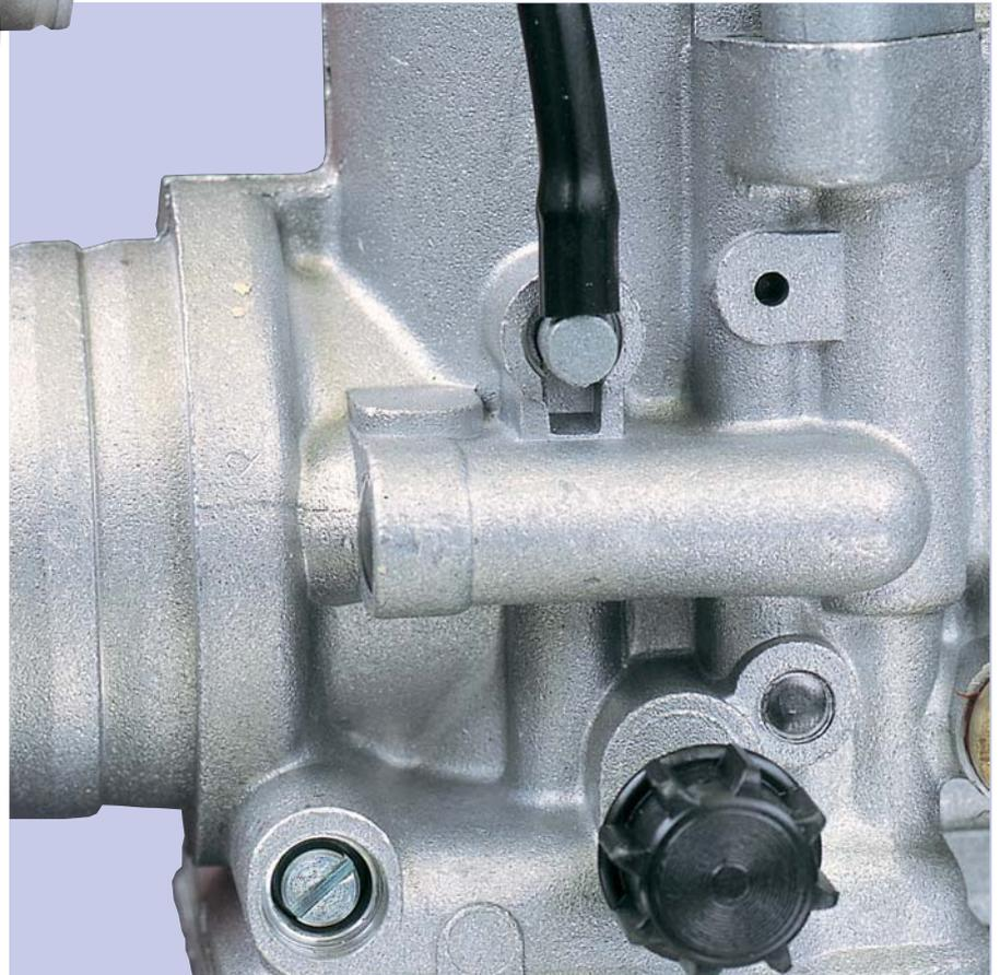
On the left side we see a VHSC with the air adjustment screw near the aspiration mouth.
