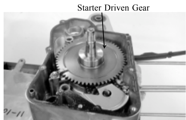
Starter Driven Gear
