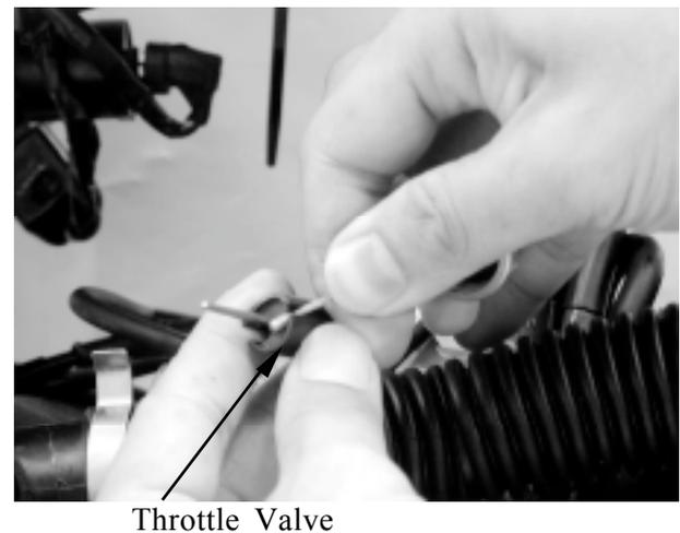
Remove the throttle valve spring, carburetor cap and rubber seal.
