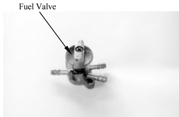
Remove the screw on the fuel valve control switch.
