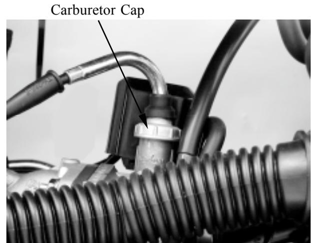
Disconnect the throttle cable from the throttle valve.
