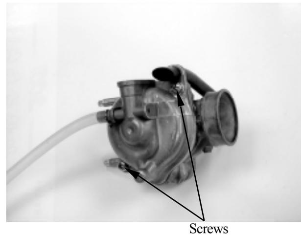
Remove the screw and O-ring.
