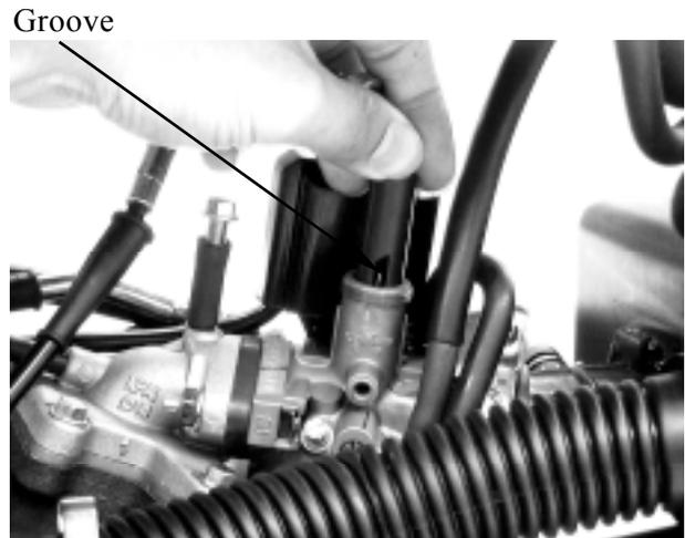
Tighten the carburetor cap.
