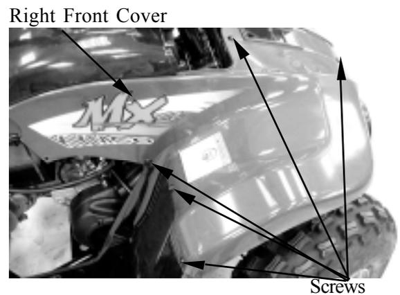
⚠ During removal, be careful not to damage the joint claws.
