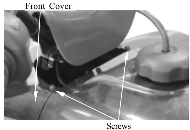
Remove the left and right front fender under bolt.
