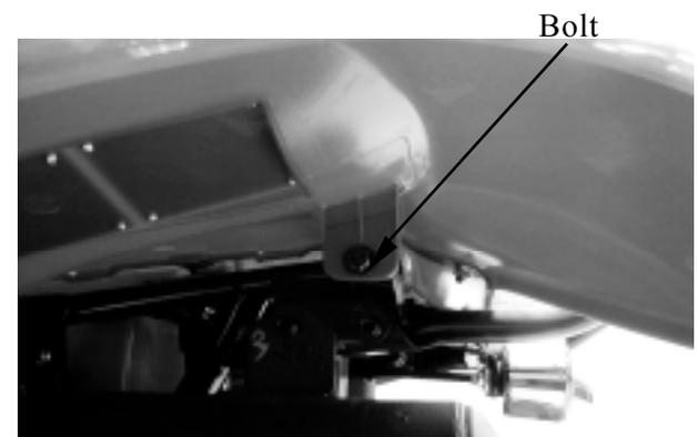
Remove right rear fender under bolt.
