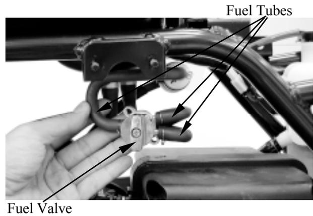
Remove the fuel valve and fuel cup.
