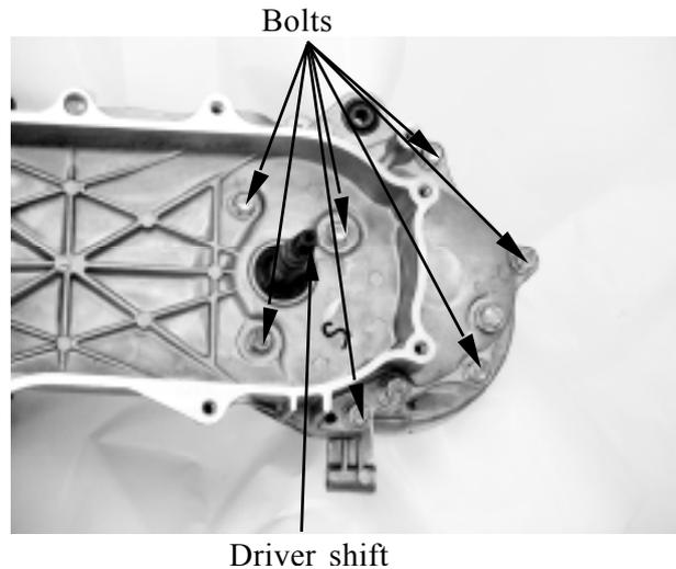
Remove the final gear and countershaft.
