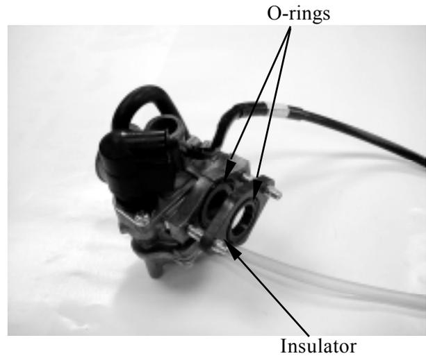
Install the carburetor and insulator onto the intake manifold and tighten the two lock nuts.
