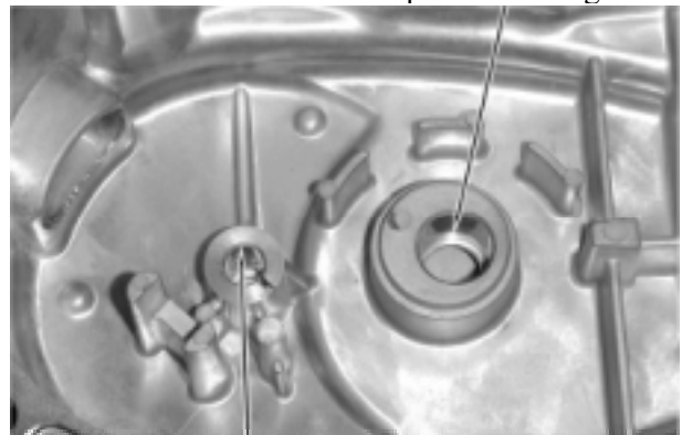
Starter Driven Gear Shaft Forcing Starting Ratchet
