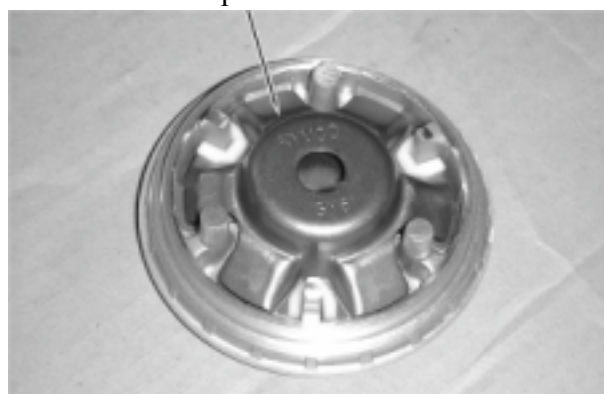
Movable Drive Face Assembly Ramp Plate
