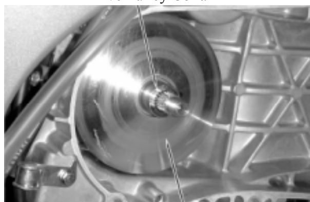
Movable Drive Face Assembly Ramp Plate
