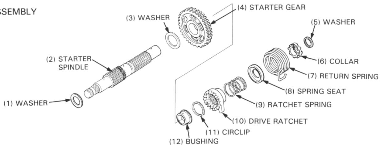
Install the thrust washer, kick starter gear and bushing.
