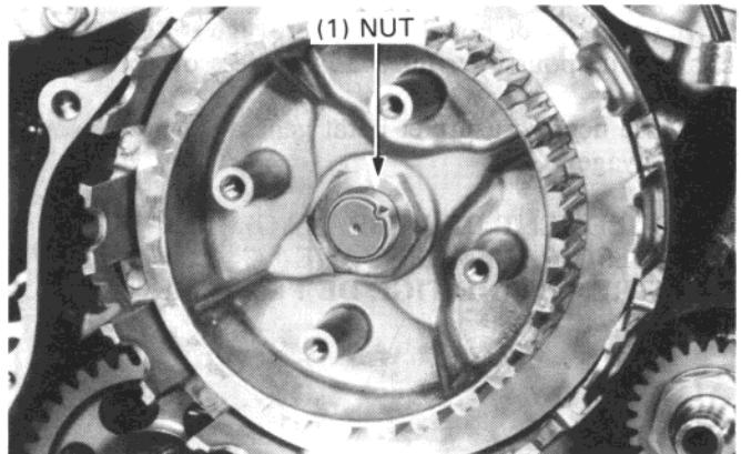
Coat the 7 discs and 6 plates with clean engine oil and install them as shown.
