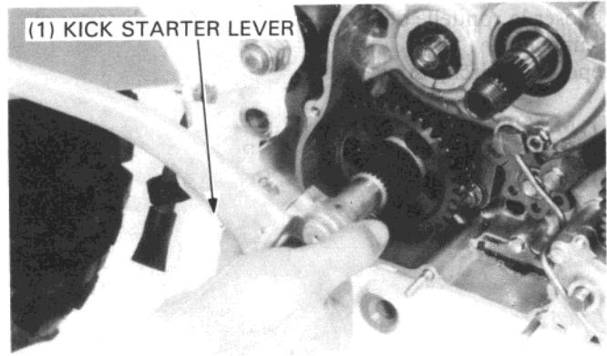
Install the thrust washer.
