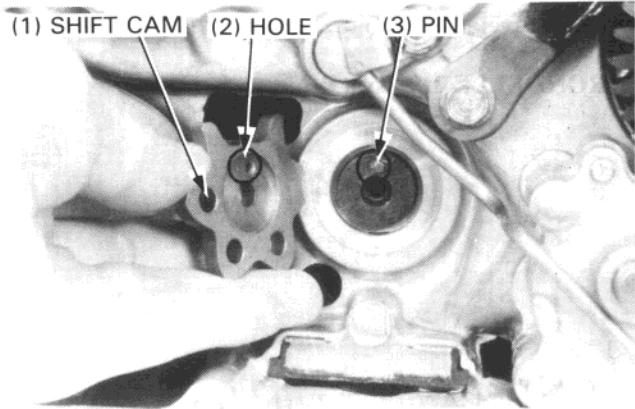
Apply locking agent to the threads of the cam plate bolt and tighten the bolt.
