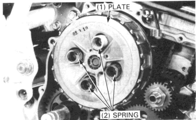
Install the clutch bolts in crisscross pattern in 2-3 steps.
