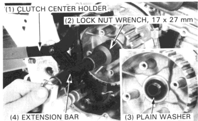
Remove the clutch center and thrust washer.
