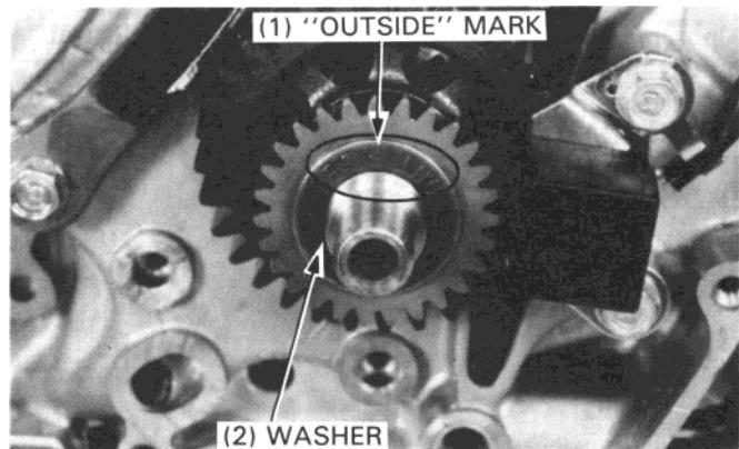
Temporarily install the clutch outer and gear holder.
