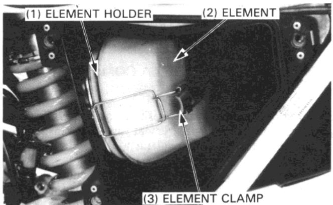
Wash the element in non-flammable or high flash point solvent, and let it dry.
