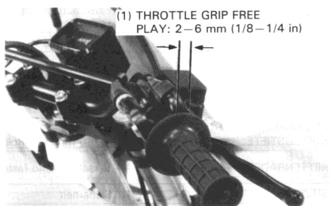
Throttle grip free play can be adjusted at either end of the throttle cable. Replace any damaged parts before beginning this adjustment.
