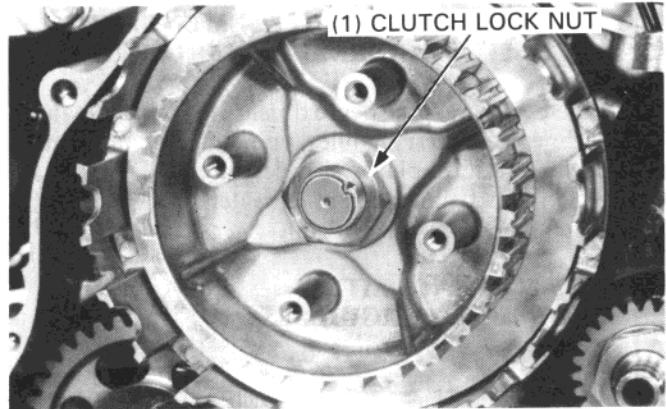
Attach the clutch center holder to the clutch center.
