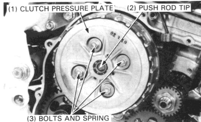
Remove the push rod tip, release bearing and lifter rod.
