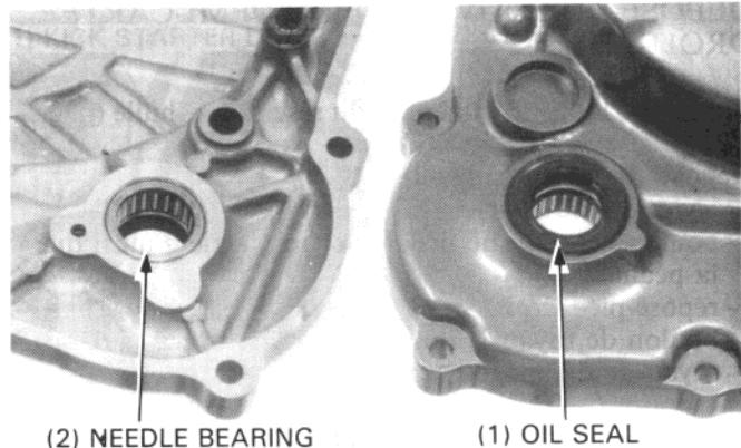
Drive in a new needle bearing with the special tools.
