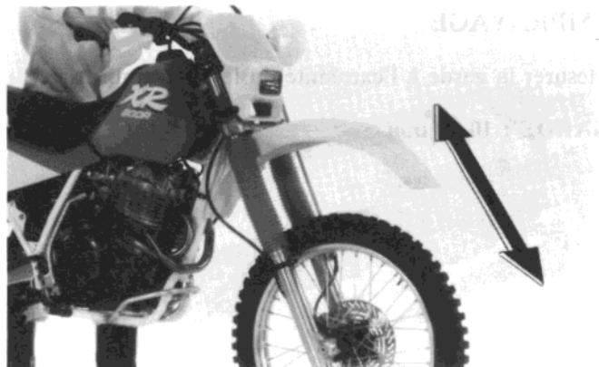
Check the fork air pressure when the fork is cold.
