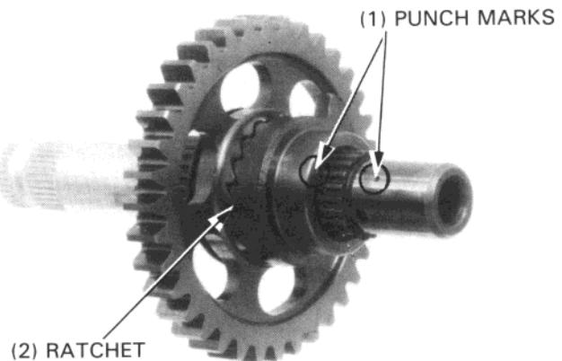
Install the ratchet spring and spring seat.
