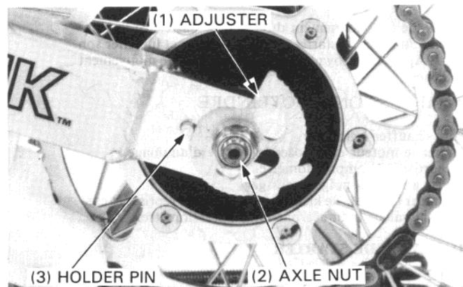
When the drive chain becomes extremely dirty, it should be removed and cleaned prior to lubrication.
