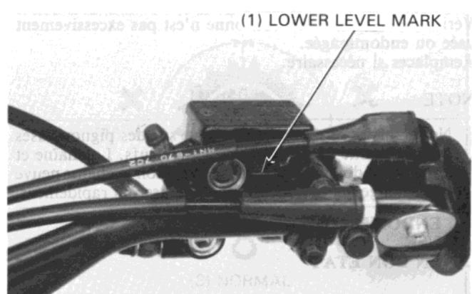
If the level was low, check the entire system for leaks.
