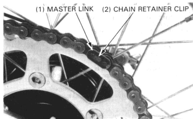
Clean the drive chain with a non-flammable or high flash point solvent that will not damage the O-rings and wipe dry.
