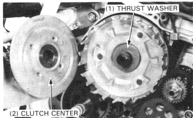
Remove the clutch outer guide from the mainshaft.
