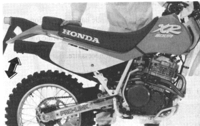
Pump grease into the swingarm, pivot bearings through the grease fitting on the swingarm. Grease the linkage bushings through the grease fittings on the linkage pivots.
