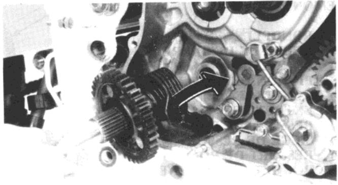
Temporarily install the kick starter lever onto the shaft.
