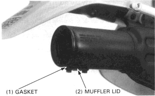
Start the engine and increase rpm to blow carbon out of the exhaust pipe while momentarily creating exhaust system back pressure by blocking the end of the muffler with a shop towel. Repeat until carbon stops coming out.
