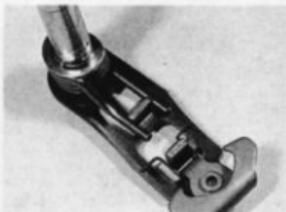
37.2 Ensure gearchange shaft return spring is correctly fitted
