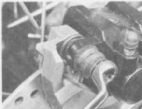
Release caliper body retaining bolt ...
