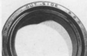
32.3 Ensure right-hand main bearing oil seal is fitted correctly (see text)
