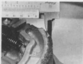
14.2a Brake shoe lining thickness measurement
