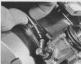
14.3a Disconnect oil delivery and feed pipes ...
