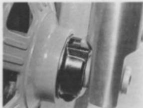
3.2a Ensure protruding lug on fork leg is positioned between ribs on gearbox - TZR model
