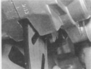
On TZR model brake caliper must be viewed from rear to check pad wear
