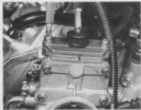
4.10 On flat-slide carburetor the top is retained by two screws
