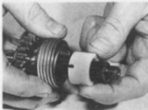
40.2d Slide nylon guide into place ensuring that notch engages with inner end of kickstart spring
