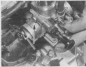
4.12b Ensure tab set in carburetor locates with cutout in inlet stub (arrowed)
