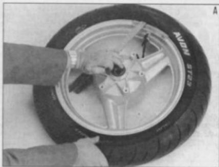
Deflate tyre. After releasing beads, push tyre bead into well of rim at point opposite valve. Insert lever adjacent to valve and work bead over edge of rim.
