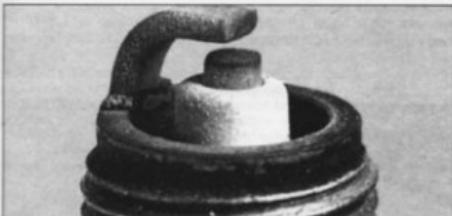
**Normal condition** - A brown, tan or grey firing end indicates that the engine is in good condition and that the plug type is correct
