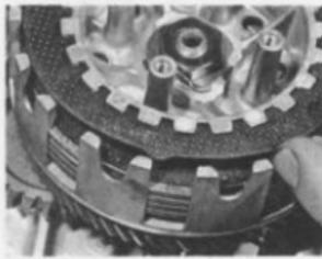
41.4 Note cutaway area on plain plates. These must be arranged as described in text
