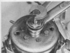
14.4 Extractor must be used to remove rotor
