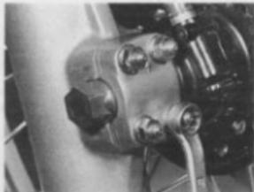
3.4b DT model - check spindle clamp is correctly fitted (arrow facing up) and tighten nuts as described in text
