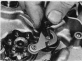
37.1 Apply thread-locking compound to shouldered bolt and refit detent arm and return spring
