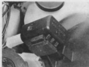
11.1a The turn signal relay is situated between oil and expansion tanks on TZR model ...
