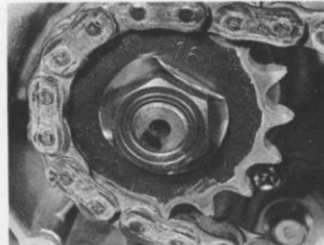
45.2 Refit gearbox sprocket and final drive chain - DT model shown
