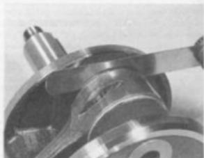
25.3 Measuring crankshaft big-end endfloat
