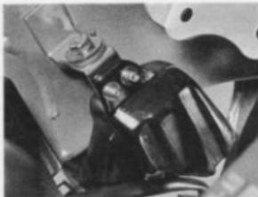
4.8b ... and remove chamber - TZR125 shown
