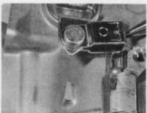
On TZR model, pointer is on end of lifting arm
