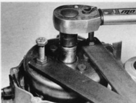
36.3b ... and lock crankshaft as shown whilst nut is tightened to specified torque setting
