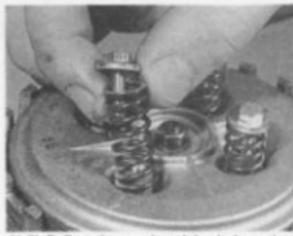
41.5b Refit springs and retaining bolts and tighten them to the specified torque setting
