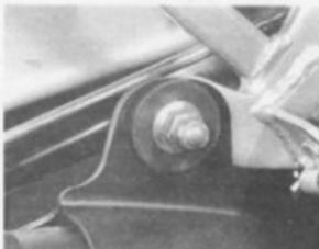
4.7b ... and remove rear mounting bolt
