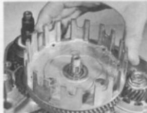
41.2a Refit clutch outer drum ...
