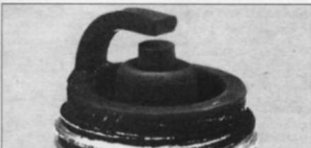
**Carbon fouling** - Dry, black sooty deposits leading to misfire and weak spark. Caused by an over-rich fuel/air mixture, faulty choke operation or blocked air filter
