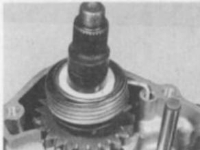
40.3b ... then engage the kickstart return spring into its locating hole
