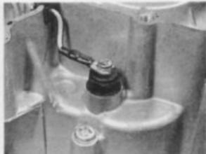
14.5a Neutral switch lead must be disconnected ...
