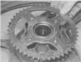
7.2d ... and lift off sprocket
