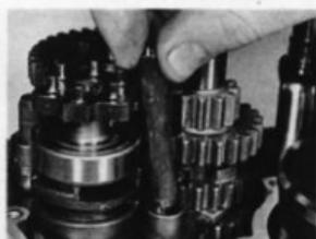
33.4c Refit selector forks into their respective slots in the drum and install selector fork shafts
