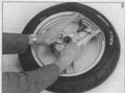
Use two levers to work bead over edge of rim. Note use of rim protectors.
