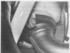
4.7d Release two front mounting nuts ...
