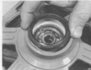
6.9c Grease seal to aid installation
