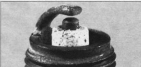
**Overheating** - A blistered white insulator and glazed electrodes. Caused by ignition system fault, incorrect fuel, or cooling system fault
