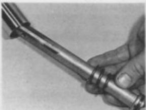
3.8a Fit rebound spring to damper rod and insert into stanchion upper end
