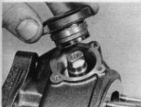
43.2b Refit sleeve and end cap assembly ...
