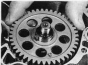
38.2c Fit balancer shaft drive gear making sure punch mark faces outwards ...
