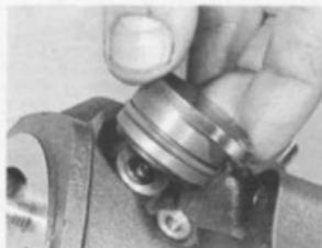
7.3b ... and remove right-hand valve cap
