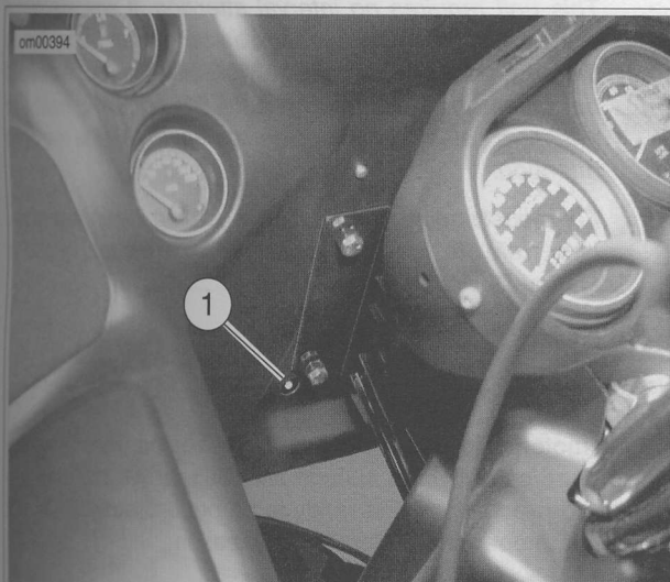
Figure 64. Headlamp Adjustment: FLTR
