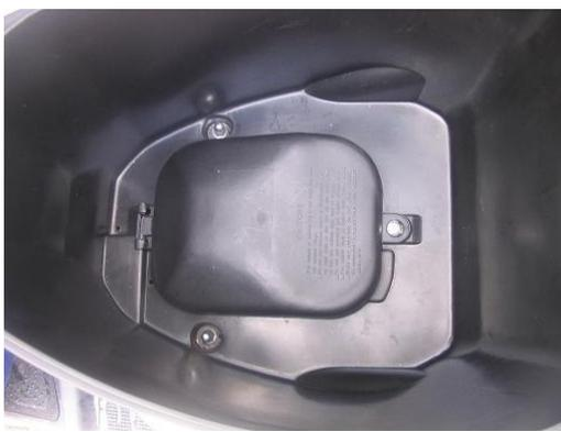
Firstly petrol. Open the seat and you should see a cover in the bottom of the storage compartment.
