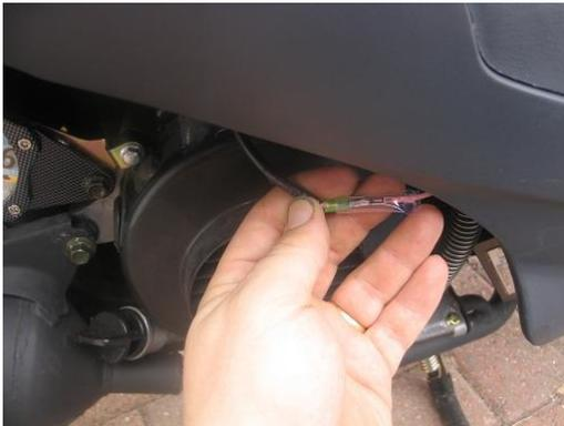
When you have disconnected this wire you will need to cover the ends with the electrical tape. **DO NOT DISCONNECT ANY OTHER WIRE.** The pink wire sends information about the speed of the back wheel to the CDI unit. If the CDI unit doesn't receive this info (because we disconnected it!) it thinks you are not moving and will allow the
