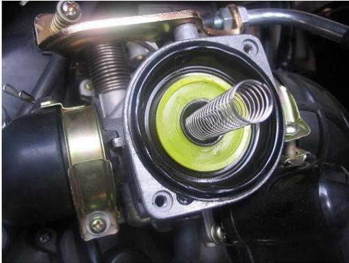
Remove the black circular cover (2 screws) VERY CAREFULLY. There is a spring under this cap and it will pop out if you are not careful. When you have removed the cover you should see this..
