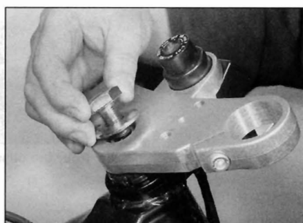
8.7 Unscrew the steering stem bolt and remove the washer
