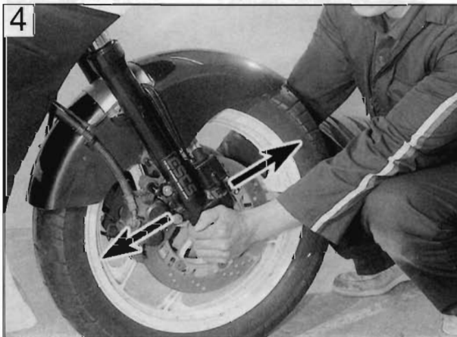
Checking the steering head bearings for freeplay
