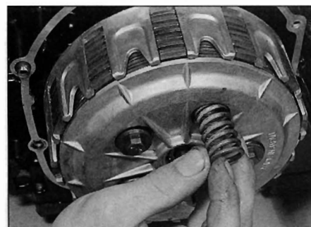
18.21b ... then install the springs and bolts ...
