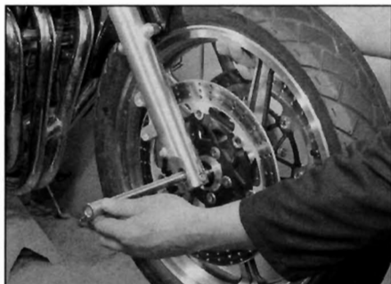
14.5 Support the wheel and withdraw the axle
