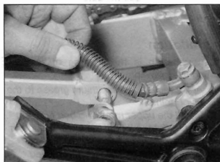
12.3 Remove the brake torque arm bolt and lift the arm off
