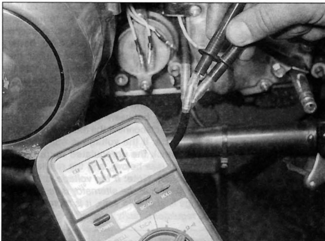
33.14 Testing stator coil resistance
