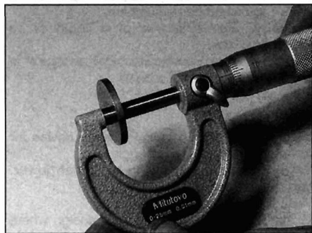
Tappet shims are measured with a micrometer
