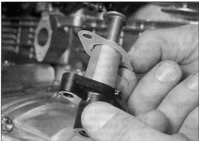
9.21a Fit a new gasket on the tensioner ...
