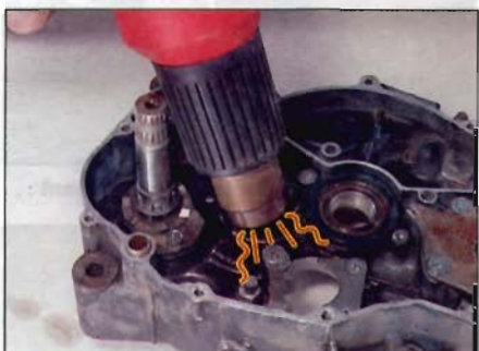
2.15 Using heat to free a seized fastener
