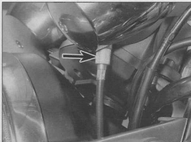
15.5 Unscrew the knurled ring securing the cable to the speedometer (arrowed) . . .
