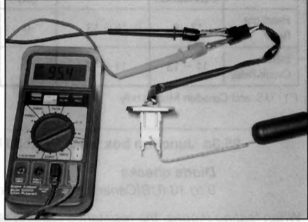
26.2b Fuel level sender testing - EMPTY position
