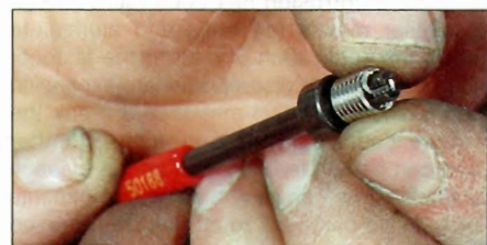
2.28 ... fit insert on the installing tool ...
