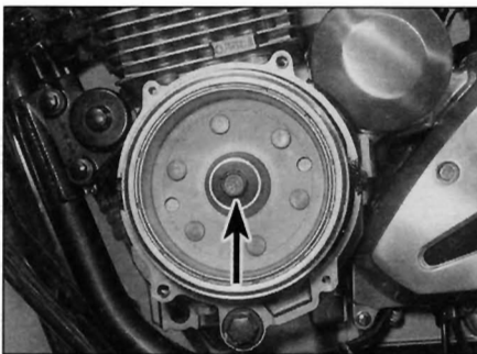
34.4 Alternator rotor bolt (arrowed)
