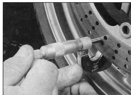
4.3b Using a micrometer to measure disc thickness
