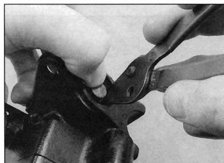
5.12a . . . then depress the piston and remove the circlip using a pair of internal circlip pliers
