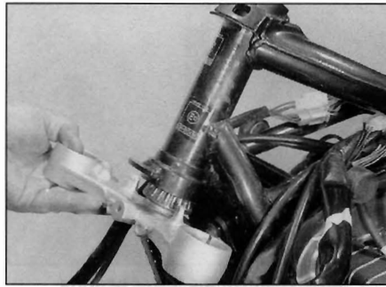
8.12a Lift the steering stem up into the head
