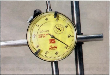
3.17 Dial gauge reading of 1.48 mm
