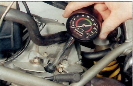
3.20 Using a rubber-cone type cylinder compression gauge
