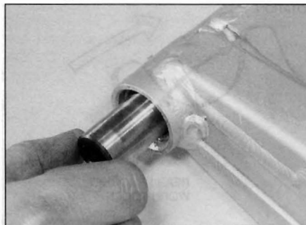
13.4b ... and withdraw the inner sleeve
