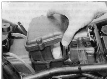
3.1 On 750 models, remove the air filter cover to access the battery
