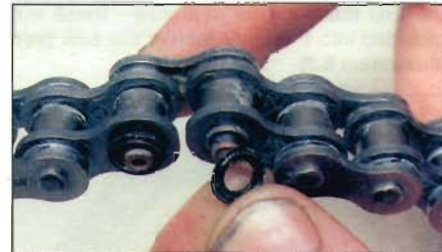
8.5 ... install the O-rings over the pin ends ...
