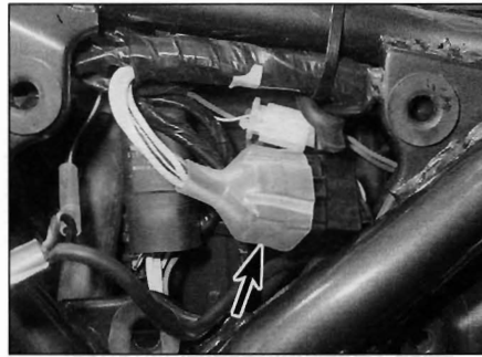
35.1a Regulator/rectifier wiring connector (arrowed) - later 550 models
