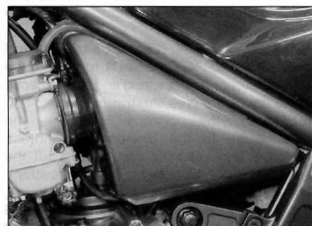
6.2 Remove the air filter housing end covers
