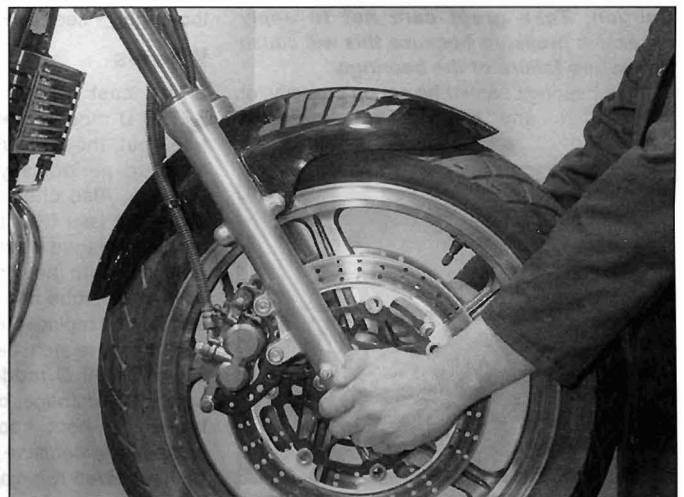
14.4 Checking for play in the steering head bearings
