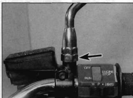
2.1 Unscrew the mirror using a spanner on the nut (arrowed)
