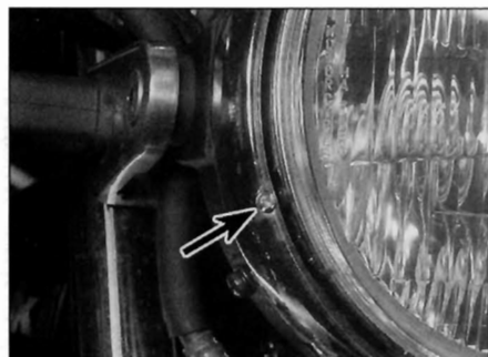
37.2 Headlight beam horizontal adjuster screw (arrowed)
