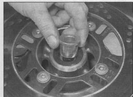
15.5b . . . and the right-hand spacer from the wheel
