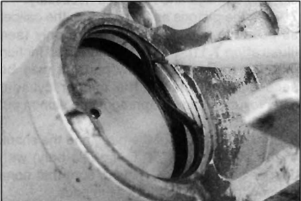
3.5 Remove the dust seal with a plastic or wooden tool (a pencil works well) to avoid damage to the bore and seal groove
