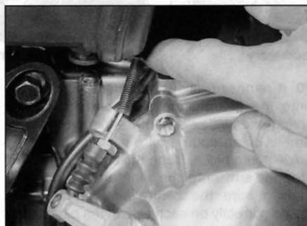
19.1f Withdraw the adjuster from its bracket ...
