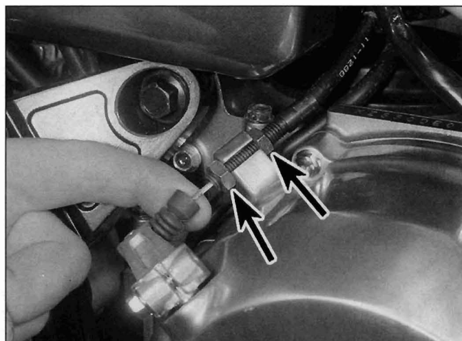
10.4 Slacken the locknuts (arrowed) and move the adjuster as required
