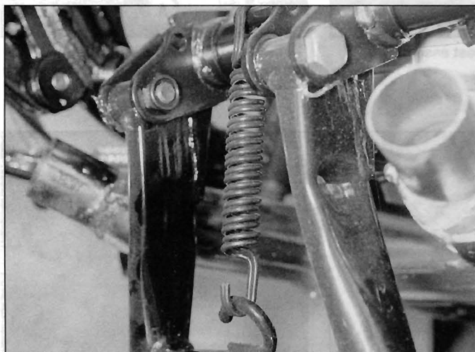
4.1 Unhook the stand spring, then unscrew the nuts and withdraw the bolts
