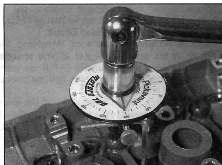
Angle-tightening cylinder head bolts
