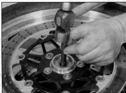
16.4a Using a drift to knock out the bearings
