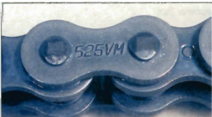
8.10 Typical chain size and type marking
