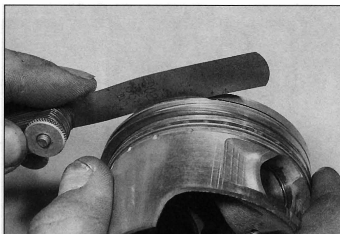
16.11 Measure the piston ring-to-groove clearance with a feeler gauge
