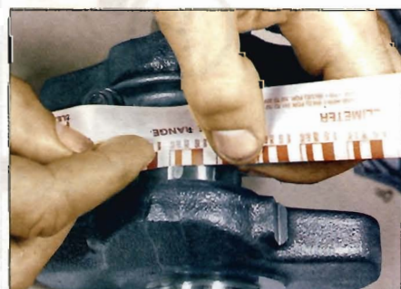
3.16 Measuring the width of the crushed Plastigauge
