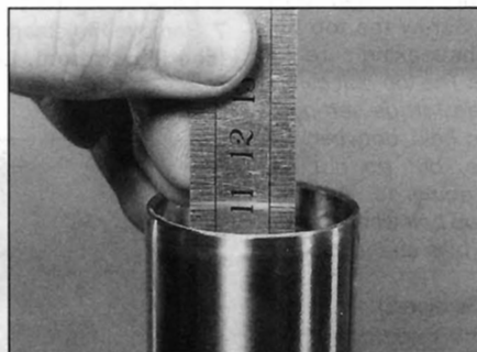
7.25b Measure the oil level with the fork held vertical
