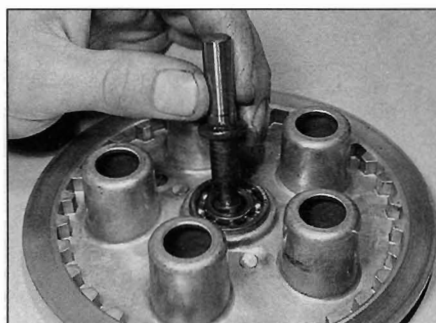
18.20 Fit the release rod through the back of the pressure plate
