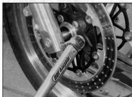
14.14 . . . and the axle clamp bolt to the specified torque setting
