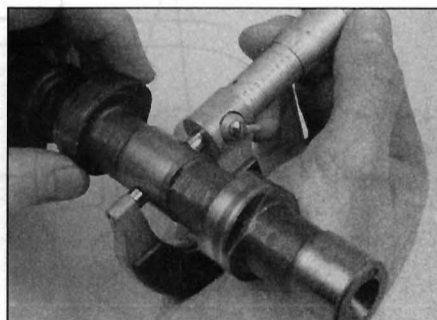
11.16b Measure the cam bearing journal with a micrometer
