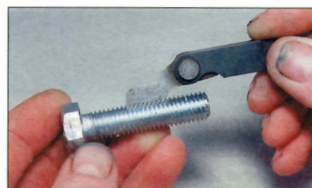
2.12 Using a thread gauge to measure pitch
