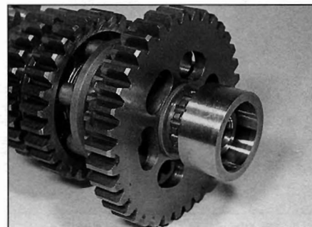
30.32e ... then slide the outer race over the bearing
