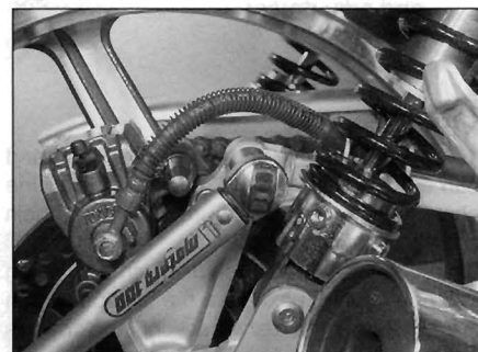
2.8b ... and the torque arm nuts to the specified torque setting
