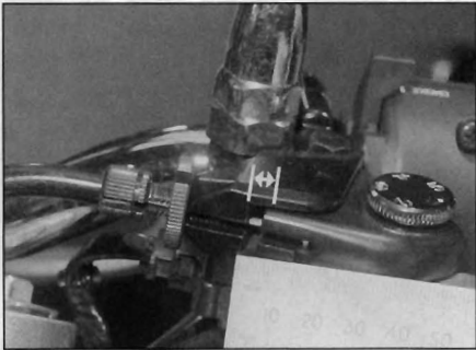
10.1 Measuring clutch lever freeplay
