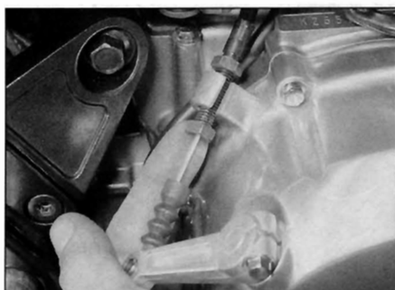
19.1b ... then slacken the upper nut and thread the nut off the adjuster
