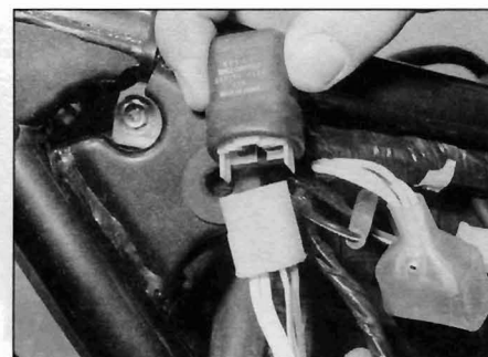
27.13c Disconnect the relay wiring connector and remove the relay
