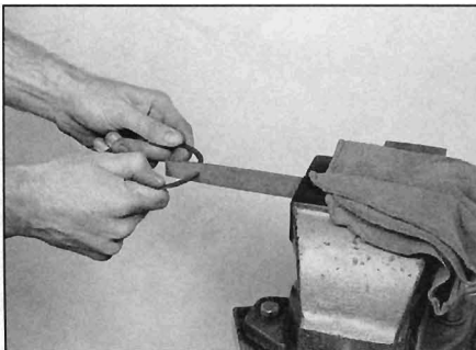
17.5 Ring end gap can be enlarged by clamping a file in a vice and filing the ring ends
