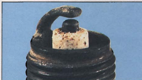
Overheating – A blistered white insulator and glazed electrodes. Caused by ignition system fault, incorrect fuel, or cooling system fault
