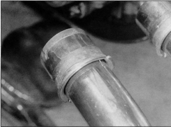
13.2c Note how the half-ring retainers fit
