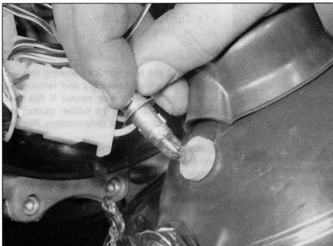
7.8a Pull the bulbholder out of the headlight . . .
