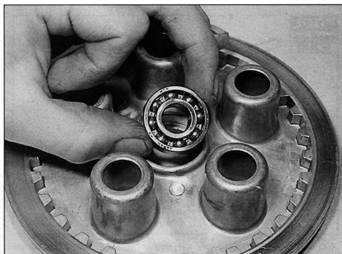
18.13 The release bearing on 550 models fit into the pressure plate
