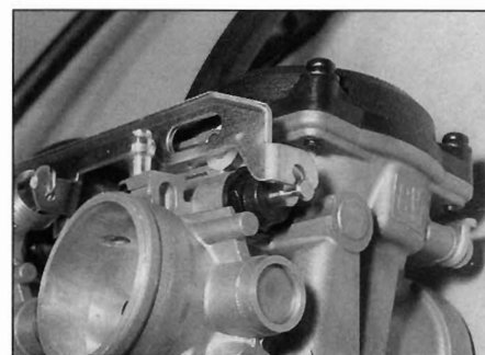
9.1c ... making sure it locates correctly onto each plunger
