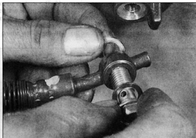
10.4 Remove the banjo bolt and separate the hose from the caliper; there is a sealing washer on each side of the fitting
