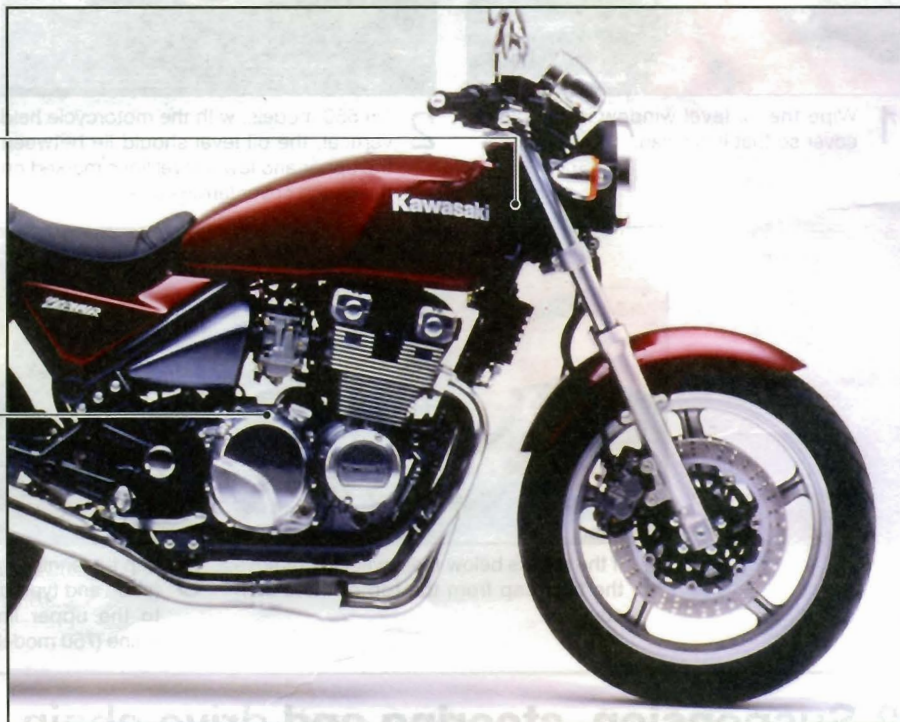
The engine number is stamped into the top of the crankcase behind the cylinder block
