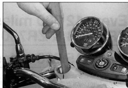
32.6b . . . then measure the level of oil in the fork
