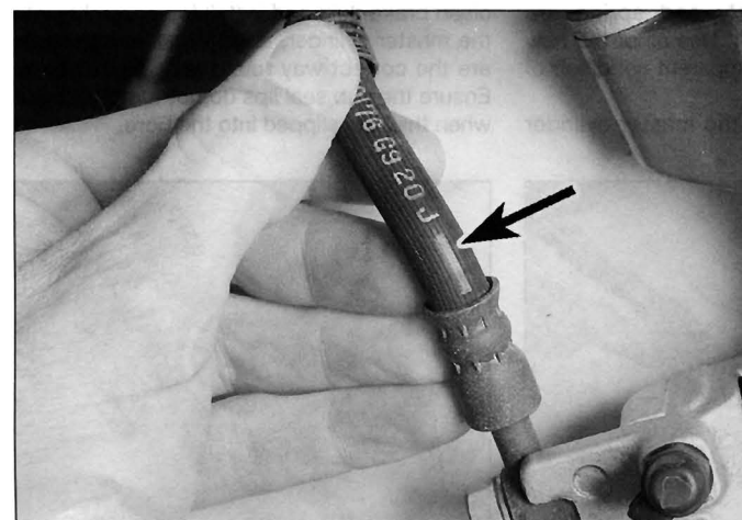
10.2 Flex the brake hoses and check for cracks, bulges and leaking fluid
