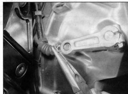
19.1g ... and remove the cable end nipple from the lever
