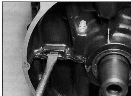
24.7 Use a screwdriver in one of the leverage points to separate the crankcase halves
