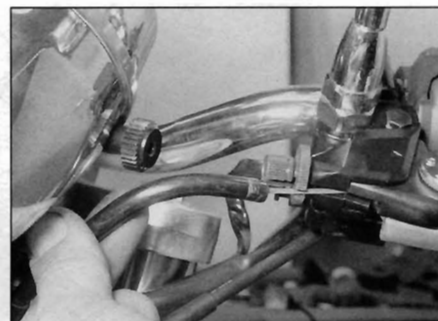
19.1d With the slots aligned, remove the outer cable from the adjuster ...
