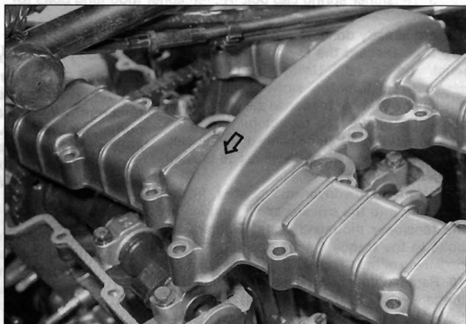
8.11 . . . then install the valve cover with the arrow facing forward
