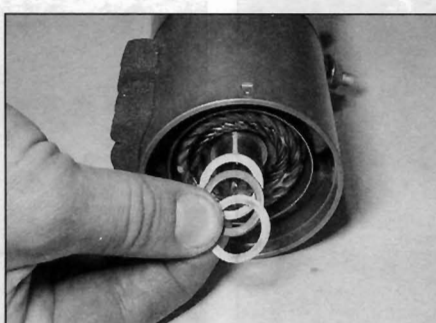
31.19b On 750 models, fit the washers onto the shaft ...
