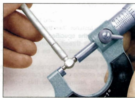
3.8 . . . then measure the gauge with a micrometer
