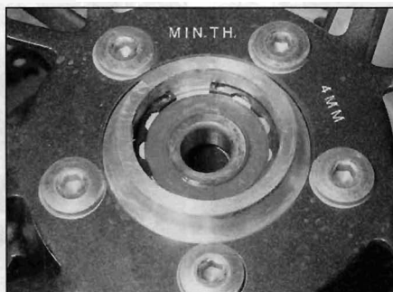
4.3a The minimum disc thickness is marked on the disc
