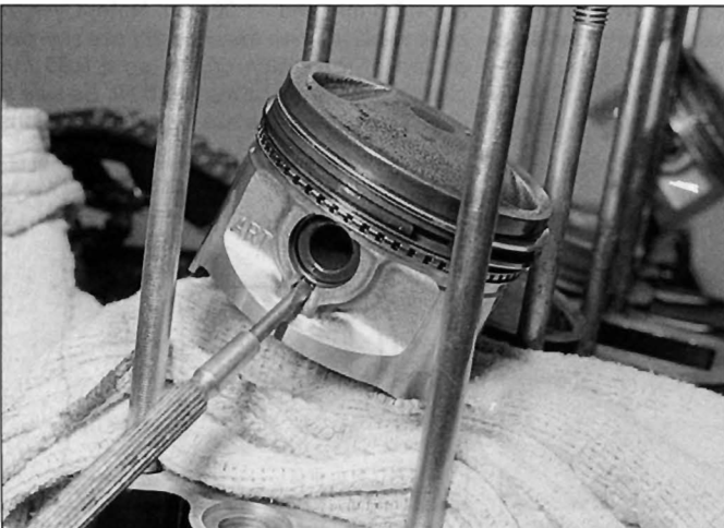
16.3a Remove the circlip using a pair of pliers or screwdriver inserted in the notch...
