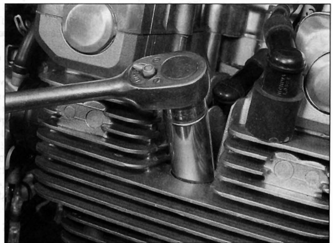
3.4b . . . then unscrew the spark plug
