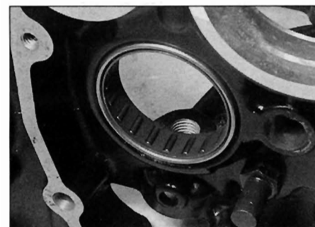
31.14 Check the needle bearing in the crankcase
