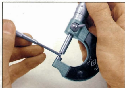
3.10 . . . then measure the gauge with a micrometer
