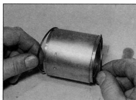
31.18a Fit new O-rings onto the main housing ...
