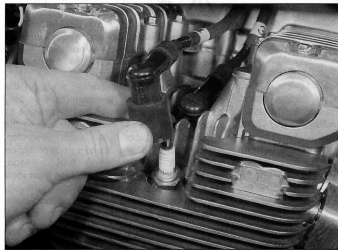
3.4a Pull off the spark plug cap . . .
