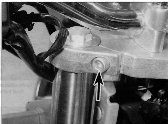
6.4 Top yoke fork clamp bolt (arrowed). Note the alignment of the fork with the top yoke as an aid to installation
