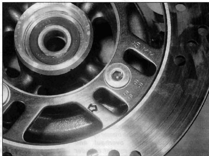
8.4 The arrow must point in the direction of normal rotation
