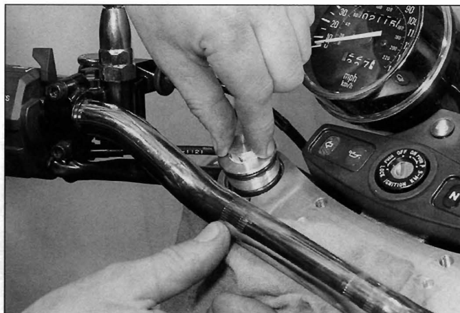
32.2b With the handlebars displaced, unscrew the fork top bolt
