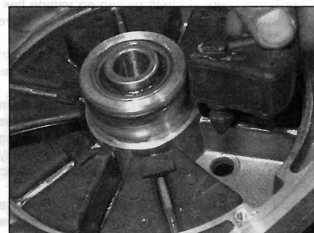
Cush drive rubbers dampen out transmission shocks
