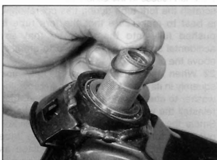
8.8b Displace the O-ring and discard it
