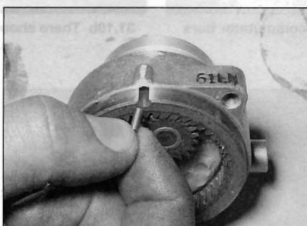
31.19d Make sure the locating pin is in place ...
