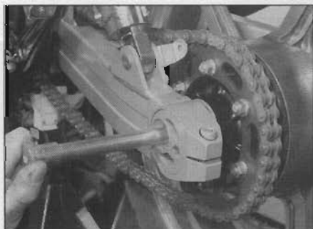
15.4 Support the wheel and withdraw the axle
