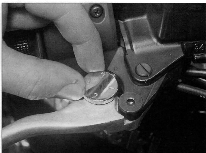
13.4 Adjusting the front brake lever span
