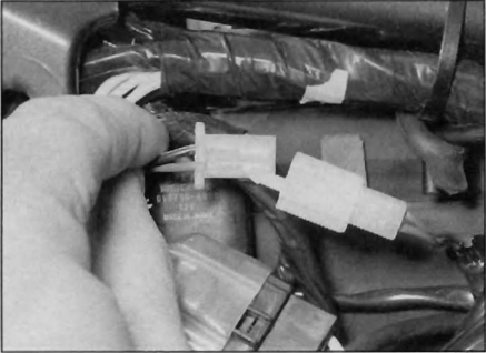
14.8b Disconnect the wiring at the connector behind the right-hand side panel
