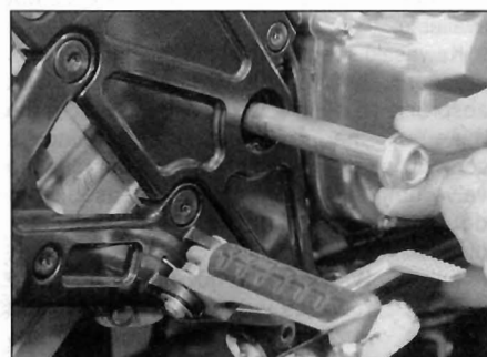
12.7c ... and withdraw the pivot bolt
