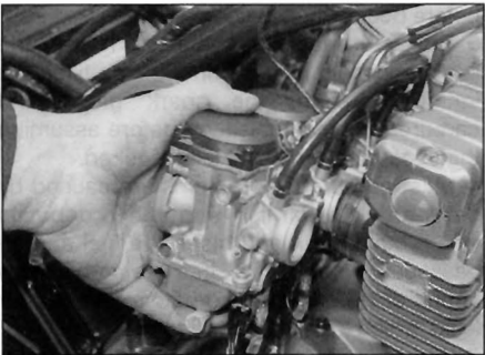
6.6b . . . and ease them off the adapters and out of the frame
