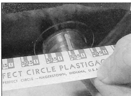
27.19 Measure the width of the crushed Plastigauge (be sure to use the correct scale - metric and imperial are included)
