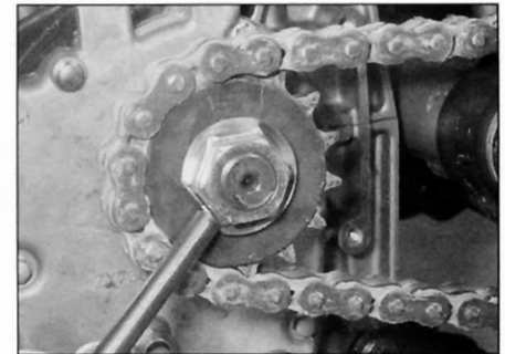
15.13 Bend up a lockwasher tab to lock the nut
