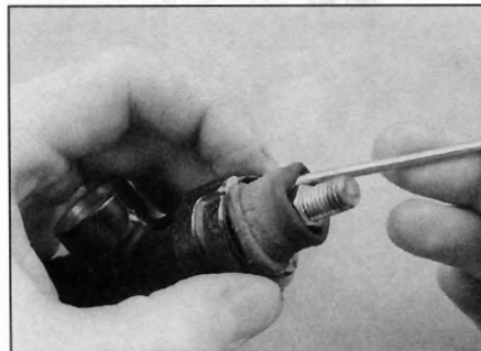
9.10b Remove the dust boot from the pushrod
