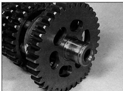
30.32a Slide the 1st gear pinion ...
