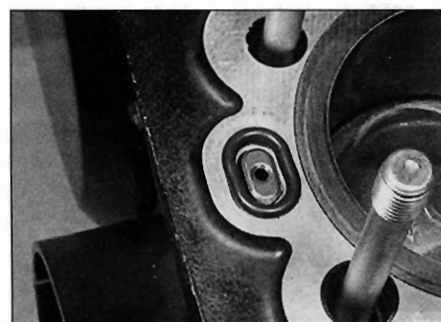
12.13b . . . and fit a new O-ring around it
