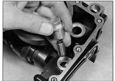
31.6 Unscrew the cam plunger bolt and remove it with the spring and plunger
