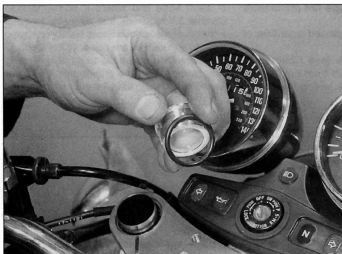
32.8a Fit a new O-ring onto the top bolt . . .
