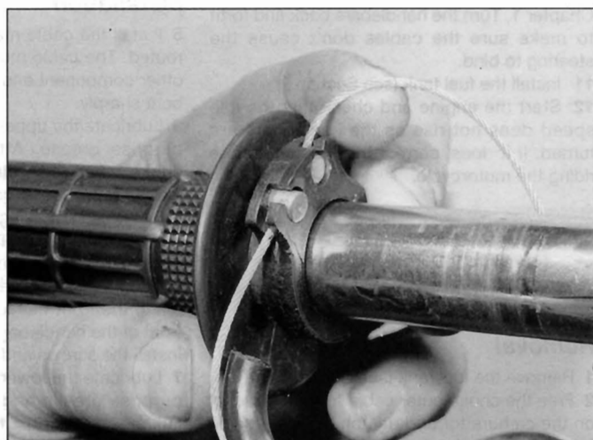
10.3c . . . then detach the cable ends from the pulley
