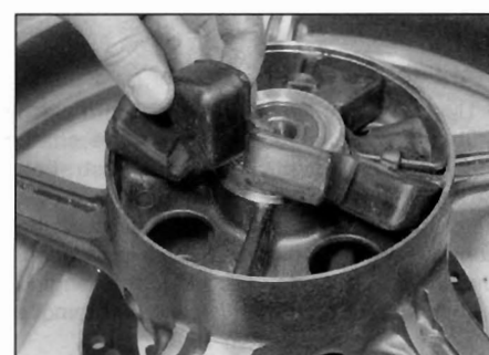
16.3 ... and check the damper segments for wear and deterioration
