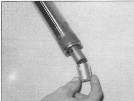
7.20b ... and fit the seat onto its bottom end
