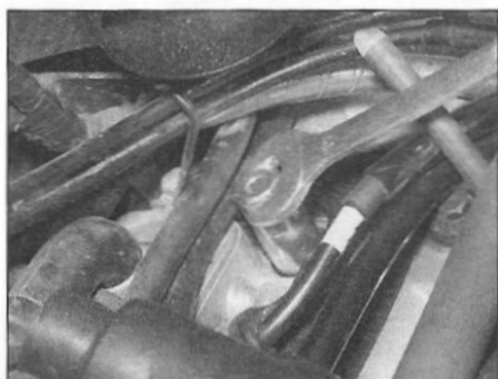
3.4b ... then unscrew the spark plug
