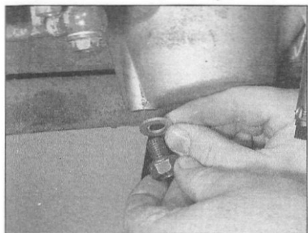
6.5a Do not forget the sealing washer and use a new one if necessary
