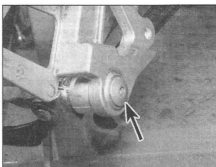
3.8b Unscrew the bolt to free the footrest and lever
