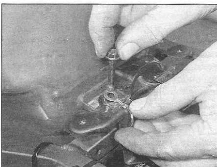
3.5 On F models secure the earth wire with the left-hand tank bolt
