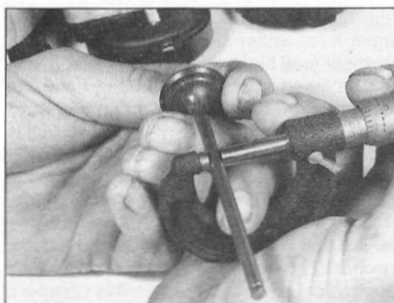
12.17a Measure the valve stem diameter with a micrometer
