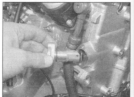
8.10b ... then install the tensioner ...
