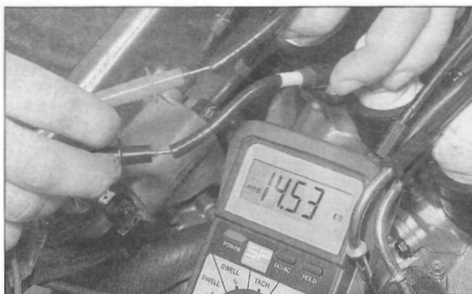
3.6 Checking the coil secondary circuit resistance
