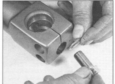
7.21 Use a new sealing washer on the damper cartridge Allen bolt
