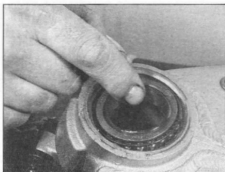
8.9 Remove the upper bearing
