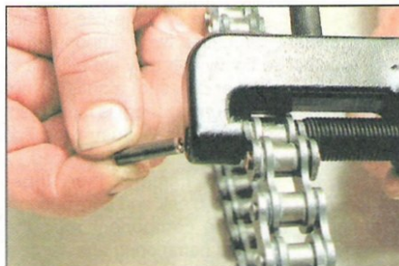
8.2 ... withdraw the pin, remove the tool ...
