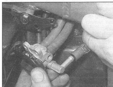
2.4b . . . then release the clamp and pull the hose off its union
