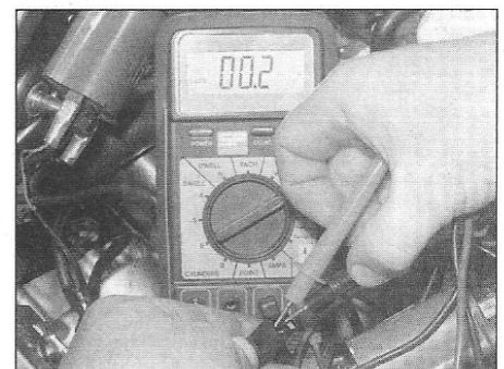
31.12 Checking stator coil resistance
