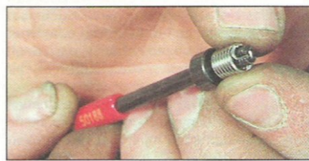
2.28 ... fit insert on the installing tool ...
