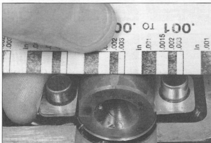
9.15a Compare the width of the crushed Plastigauge to the scale printed on the Plastigauge container
