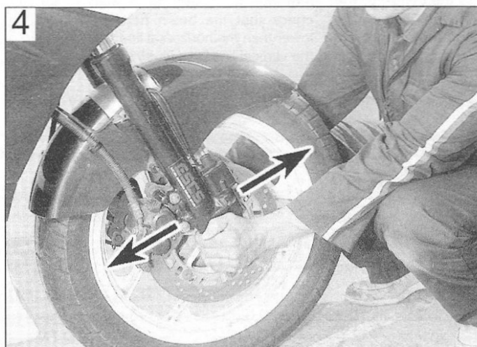
Checking the steering head bearings for freeplay
