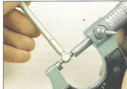
3.8 ... then measure the gauge with a micrometer
