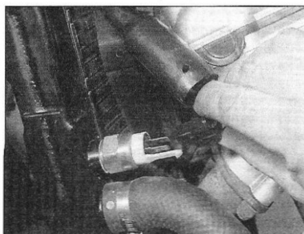
4.1 Disconnect the wiring connector from the fan switch
