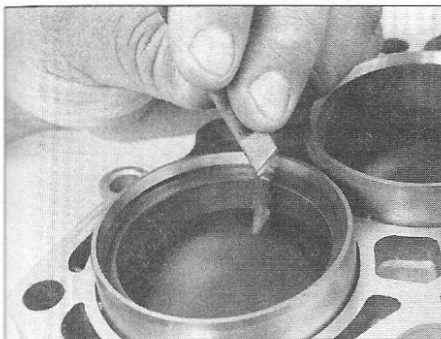
15.3 Measuring piston ring installed end gap
