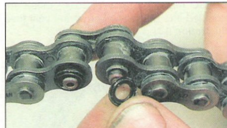
8.5 ... install the O-rings over the pin ends ...
