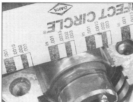
26.12 Measure the width of the crushed Plastigauge
