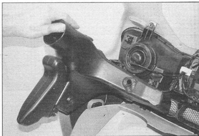
9.2b . . . and lift out the ducts
