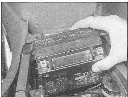
3.3b ... and remove the battery
