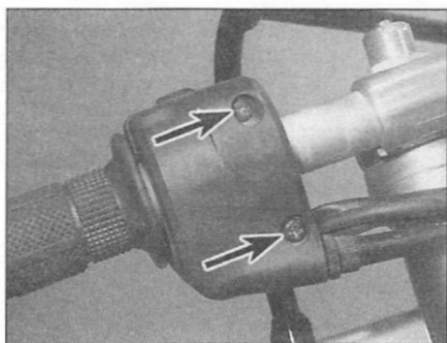
10.3a Throttle housing screws (arrowed) – F models
