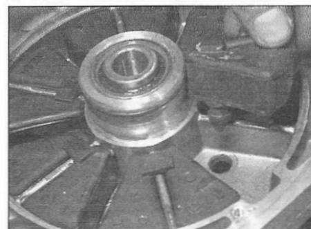
Cush drive rubbers dampen out transmission shocks
