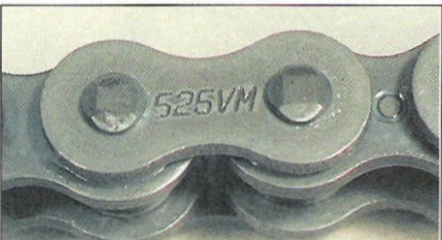
8.10 Typical chain size and type marking
