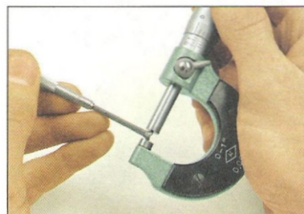
3.10 ... then measure the gauge with a micrometer
