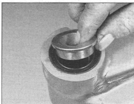
14.4a Remove the collar and cap . . .
