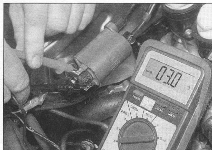
3.4 Checking the coil primary circuit resistance
