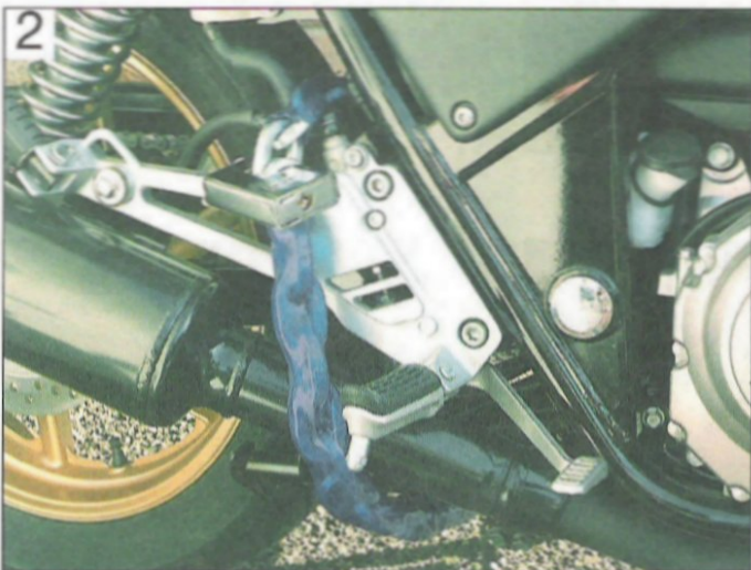
Pass the chain through the bike's frame, rather than just through a wheel...
