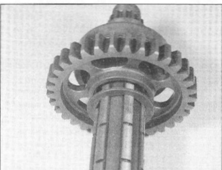
31.19b ... the toothed washer and 2nd gear ...
