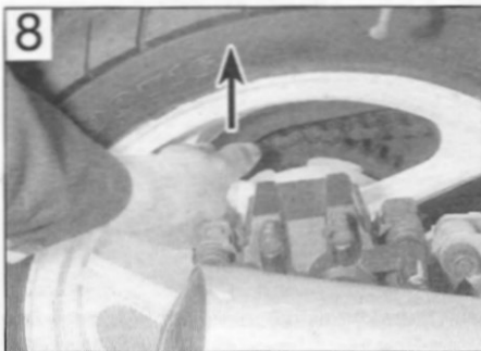
Checking for rear suspension linkage play
