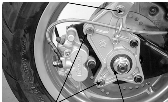
Brake Caliper Bolts
