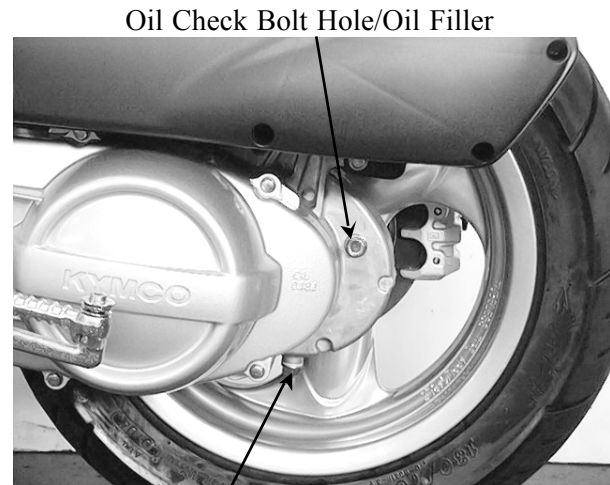
Drain Bolt
