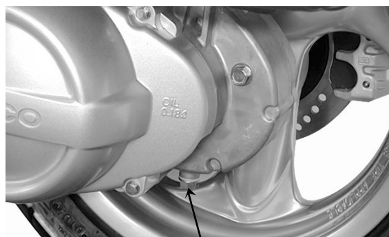
Oil Drain Bolt/Sealing Washer
