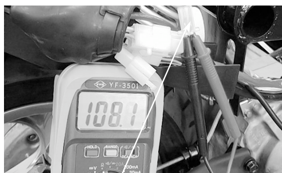
Pulser Coil Wire Coupler
