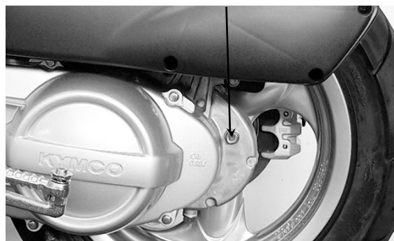
Oil Check Bolt Hole/Oil Filler
