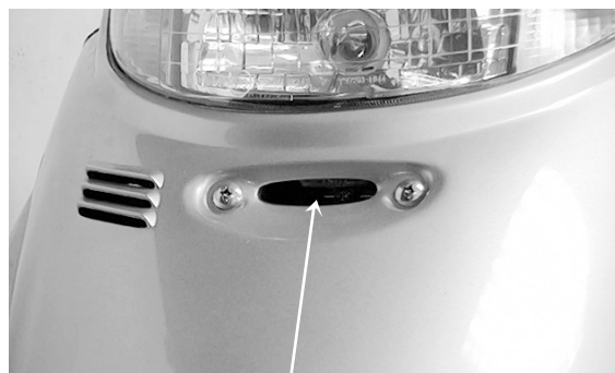
Headlight Aim Adjusting Bolt
