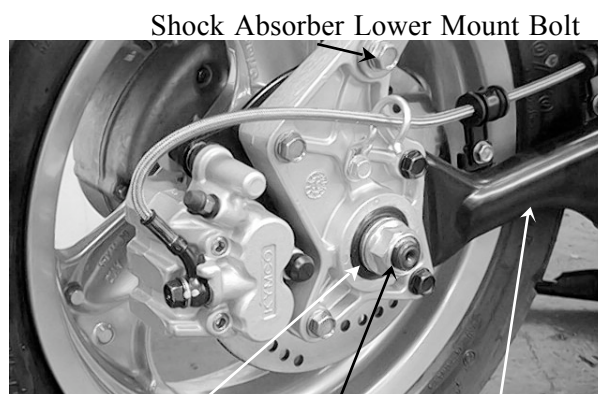
Shock Absorber Lower Mount Bolt Collar Axle Nut Rear Fork
