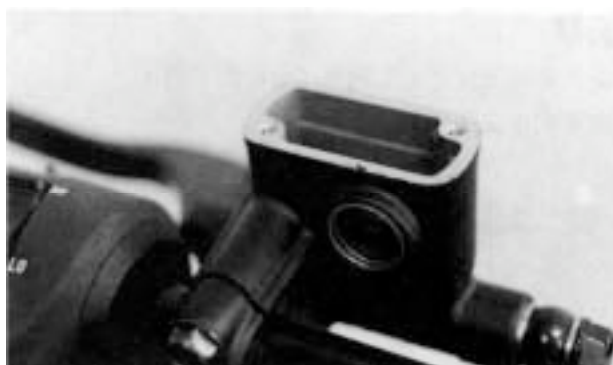
Stop Switch Wire Connector
