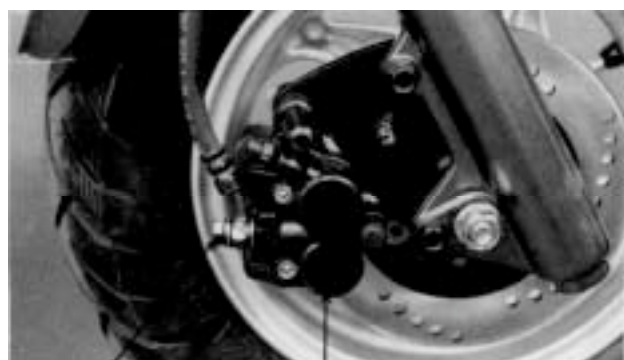
Fluid Tube Bolt
