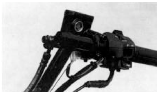
Stop Switch Wire Connector
