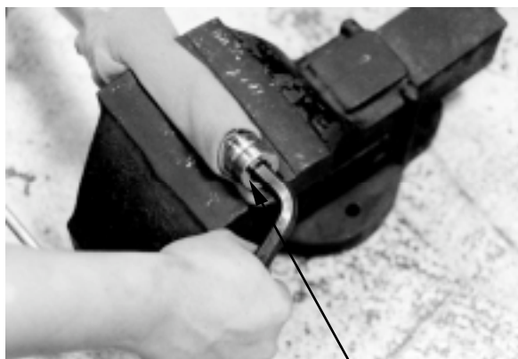
Shock Absorber Tube Circlip
