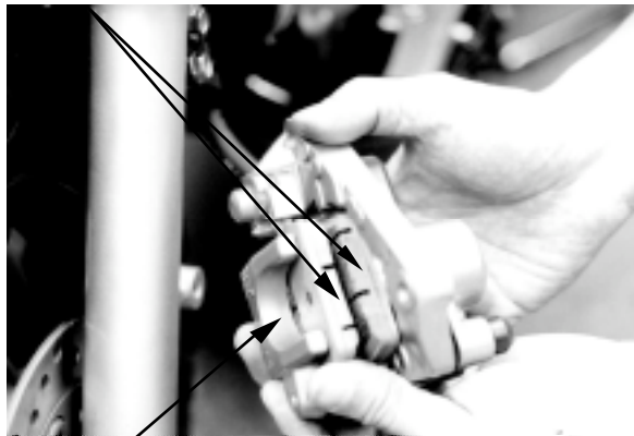
Front Brake Caliper
