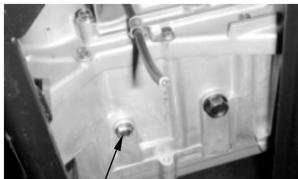
Oil Drain Bolt/ Sealing Washer
