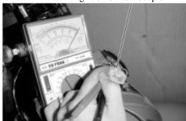
Ignition Switch Coupler
