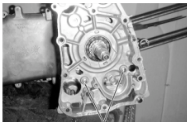
Crankcase Bolts Gasket
