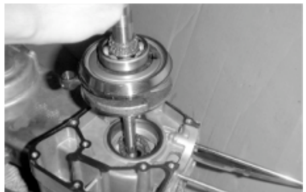
Crankshaft Bearings
