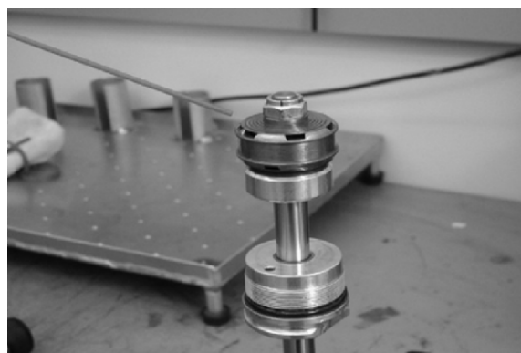
Valve Nut Torque 12 ft. lbs. (17 Nm)
