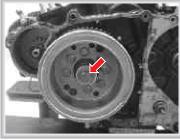
Rotor Mounting Bolt
