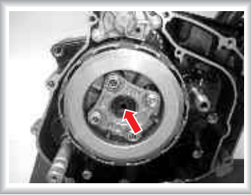
Clutch Nut (LH Threads)
