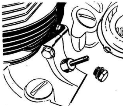
Timing plunger is position (500)
