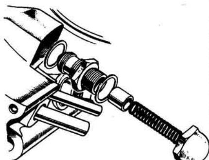
Pressure relief valve (Trident)
