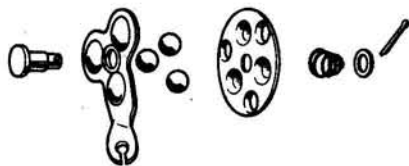
Clutch operating mechanism
