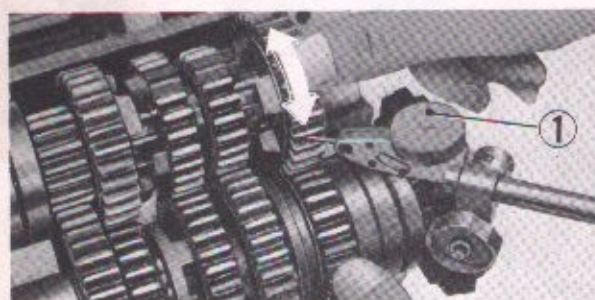
Fig. 4-109. Measuring the gear backlash
