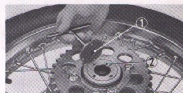
① Bearing retainer tightening wrench ② Bearing retainer Fig. 5-129. Removing the bearing retainer
