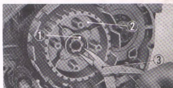
① 25 mm circlip ② Clutch center ③ Pliers
