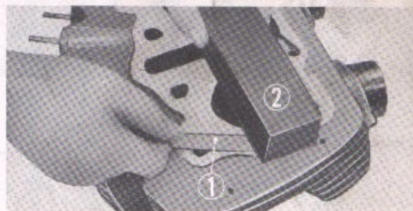
① Thickness gauge ② Stretch
