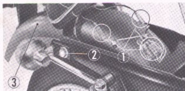
Fig. 5-64. Removing the rear fork
