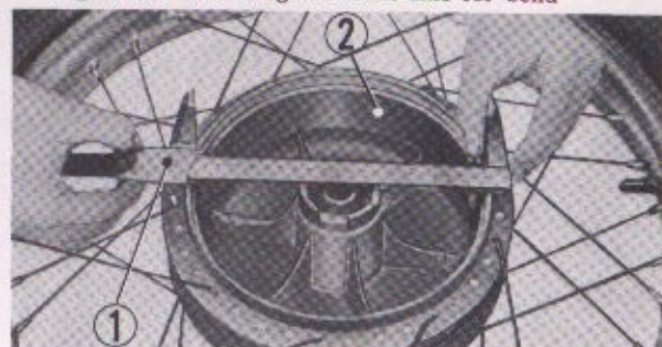
① Vernier caliper ② Front wheel hub Fig. 5-86. Measuring front brake drum inside diameter
