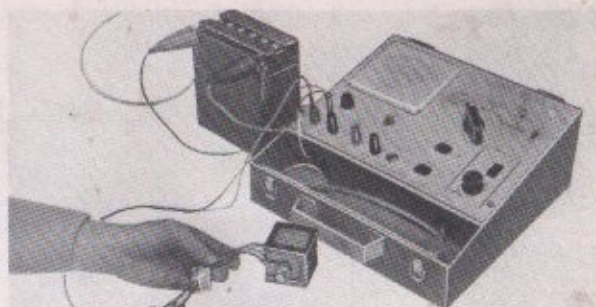
Fig. 6-40. Rectifier resistance measurement
