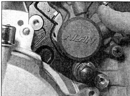
7.13 Mount the caliper onto the disc
