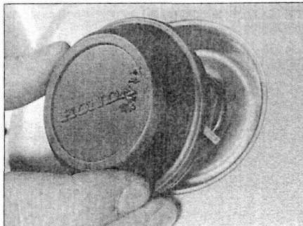
15.10b . . . then fit the wheel nut cap . . .
