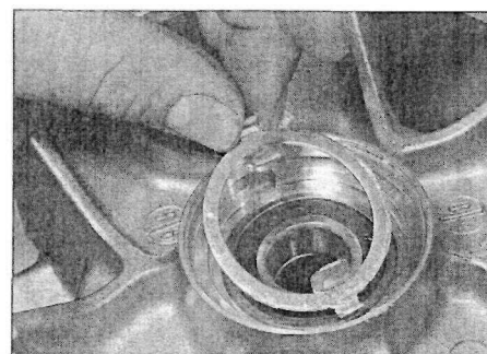
16.4 Remove the speedometer driveplate
