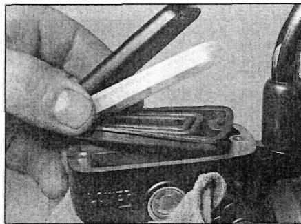
5.26 Install the rubber diaphragm, the diaphragm plate and the reservoir cover
