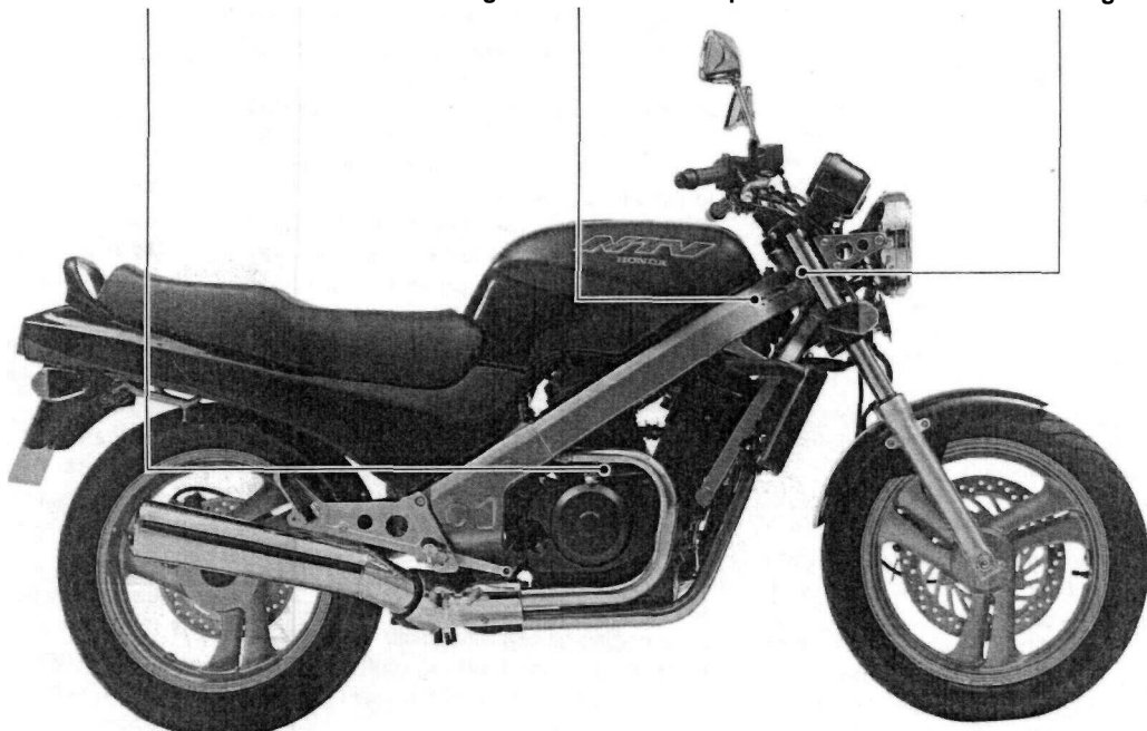
The engine number is on the right-hand side crankcase above the clutch cover
