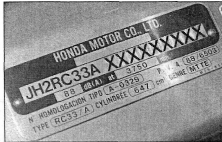
The model identification plate is mounted on the right-hand side frame spar
