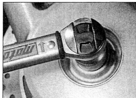
15.9 Tighten the axle nut to the specified torque setting
