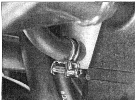
3.2 The reservoir inlet/outlet hose is secured by a screw type clamp
