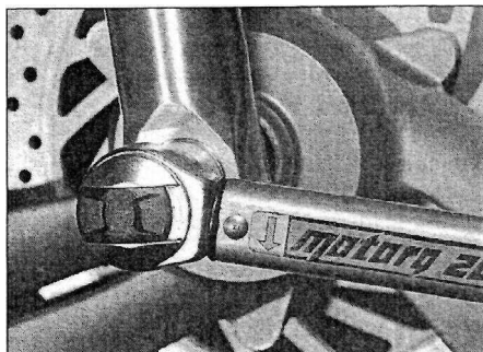
14.14b . . . and tighten it to the specified torque setting
