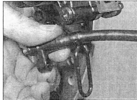
14.17a Fit the speedometer cable into its guide on the brake caliper . . .
