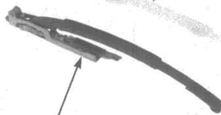
CAM CHAIN TENSIONER
