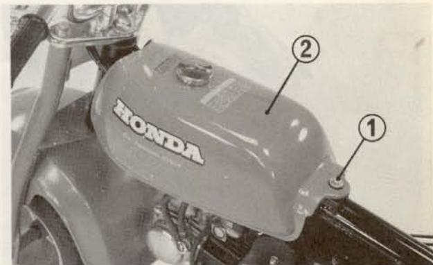
Fig. 11 (1) Bolt (2) Fuel tank
