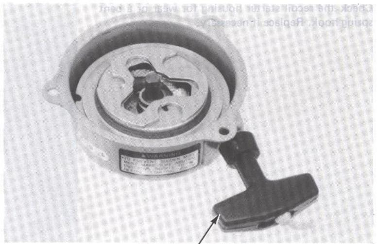
Remove the starter rope from the drive pulley.
