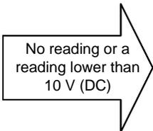
RR at fault. Replace it with a new one and return to START
