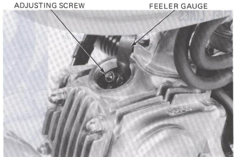
Adjust by loosening the lock nut and turning the adjusting screw until there is a slight drag on the feeler gauge.
