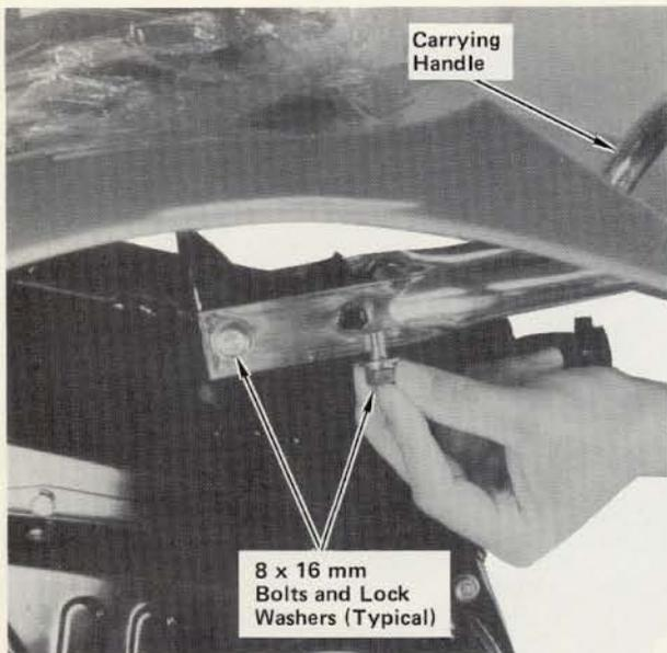
**STEP 16**—Install carrying handle on frame, with curved end up, using four 8 x 16 mm bolts and lock washers. Tighten bolts to specified torque.
