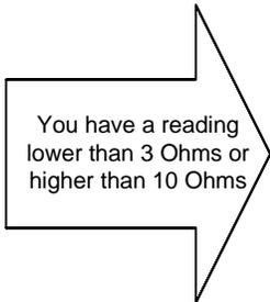
The fieldwinding in the generator or the brushes to the rotor are at fault. If there are any brushes inside the generator, disconnect them and measure the resistance between the two copper slip-rings on the rotor. These are the rings on which the brushes run.
