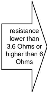
Rotor at fault. Replace it with a new one, and return to START
