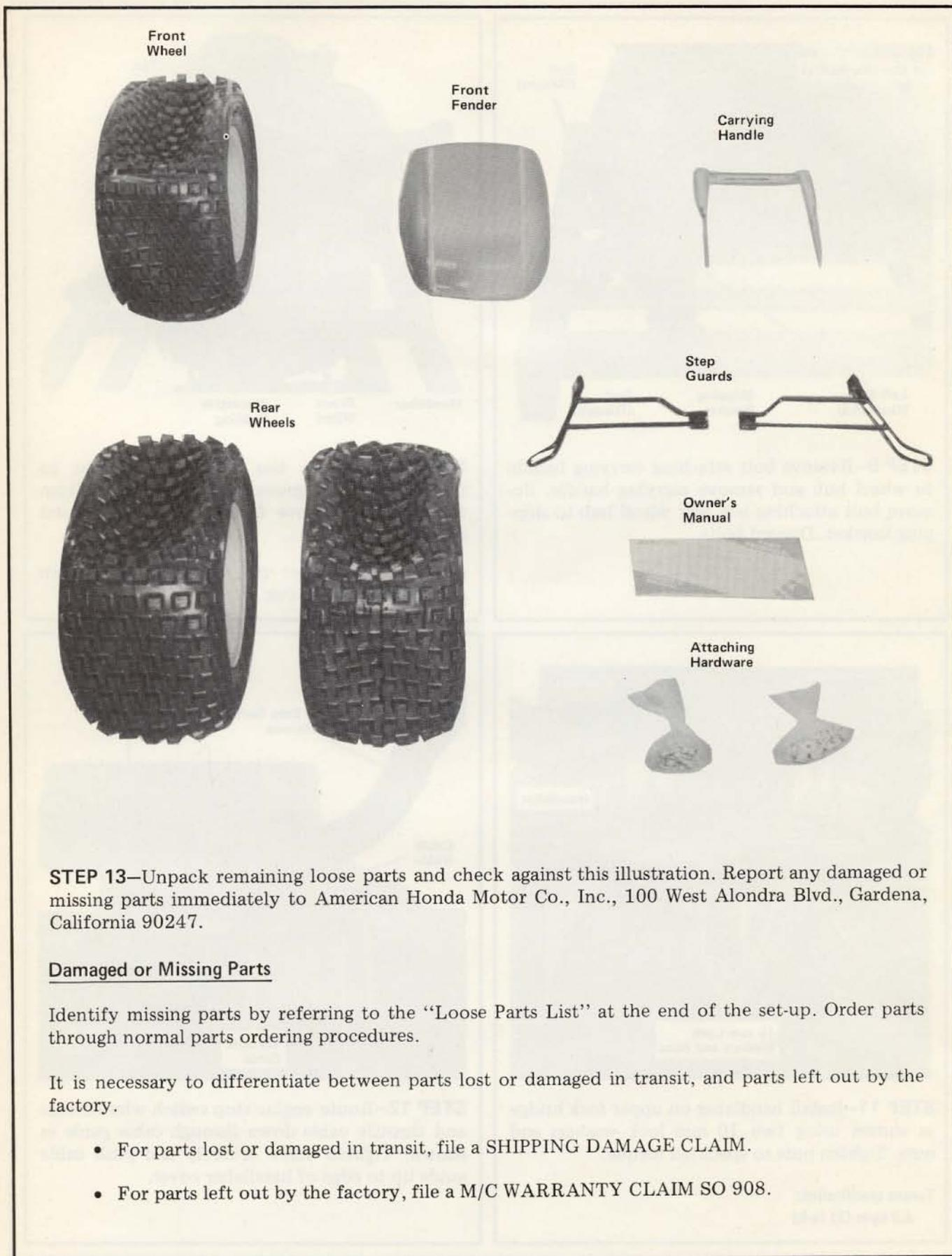
**STEP 13**—Unpack remaining loose parts and check against this illustration. Report any damaged or missing parts immediately to American Honda Motor Co., Inc., 100 West Alondra Blvd., Gardena, California 90247.
