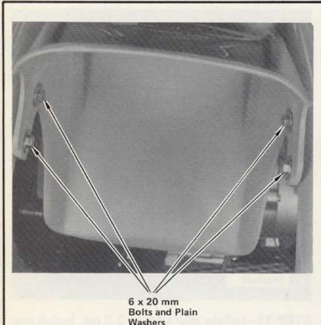
**STEP 20**—Install front fender using four 6 x 20 mm bolts and plain washers. Tighten bolts securely.
