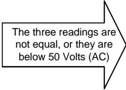
Stator at fault. Replace stator and return to START
