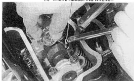
(1) VALVE ADJUSTING WRENCH
