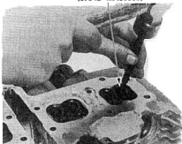
(1) VALVE GUIDE REMOVER (07942-MA60000)
