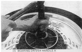
(1) BEARING DRIVER HANDLE A BEARING DRIVER OUTER (42 x 47 mm) DRIVER PILOT (17 mm)
