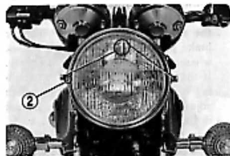
(1) Headlight mounting bolts
