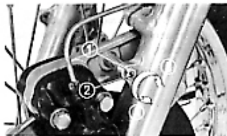
(1) Stopper bolt lock nut (2) Stopper bolt
