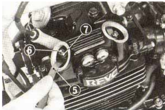
(5) Feeler gauge (6) Adjusting screw
