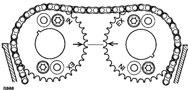
**Camshaft to Cylinder Head Alignment Marks**
