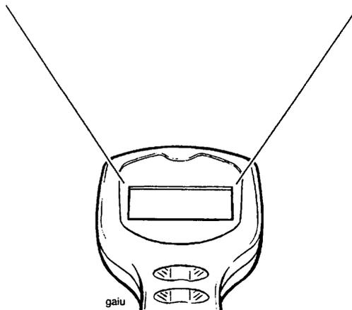
If the test is satisfactory the display will read ‘**TEST COMPLETE**’. Press the Validation key ‘\*’ to display ‘**FUNCTION TEST**’ (operation 24).
