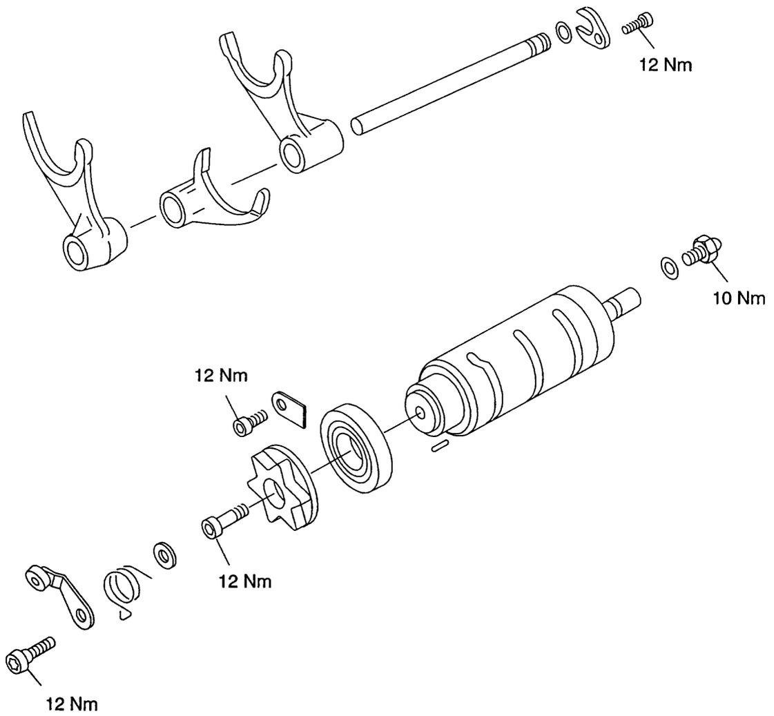
Exploded View, Gear Change Mechanism
