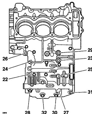
**Upper Crankcase Bolt Tightening Sequence**
