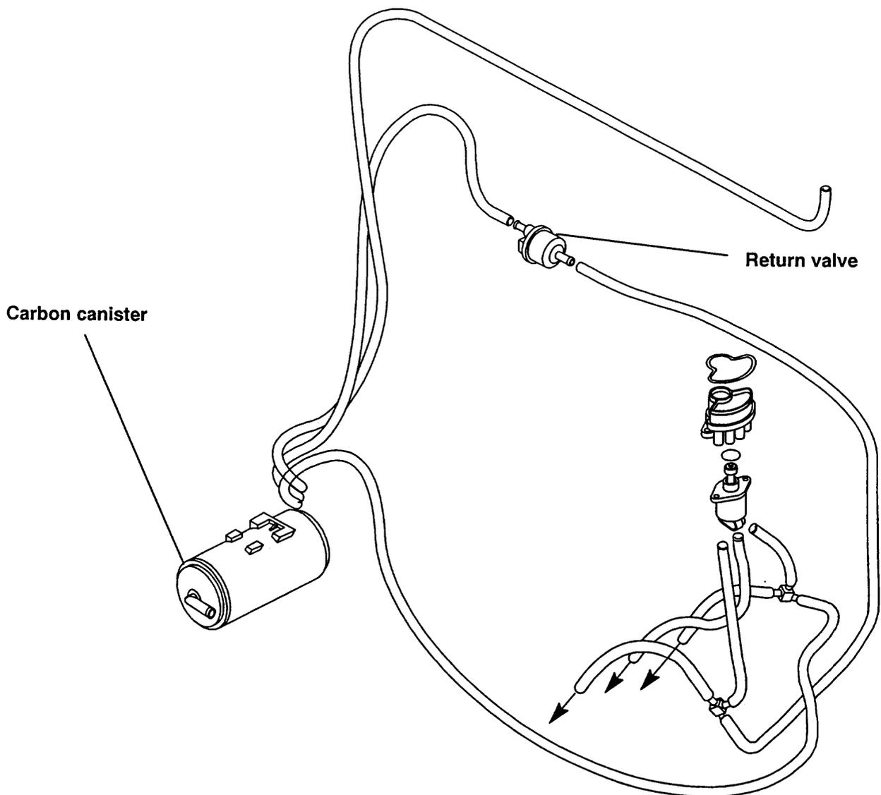
**Evaporative Control System - Engine Off.**
