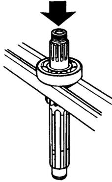
4. Fit a new circlip (11) to the input shaft ensuring that the clip is correctly located in the circlip groove.
