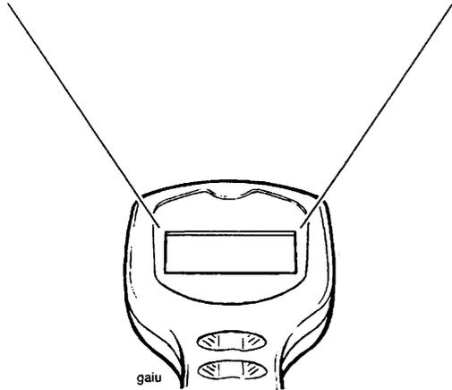
The screen will display the message 'Triumph Motorcycles Diagnostic Tool' and will also give the diagnostic software version and the software release year.
