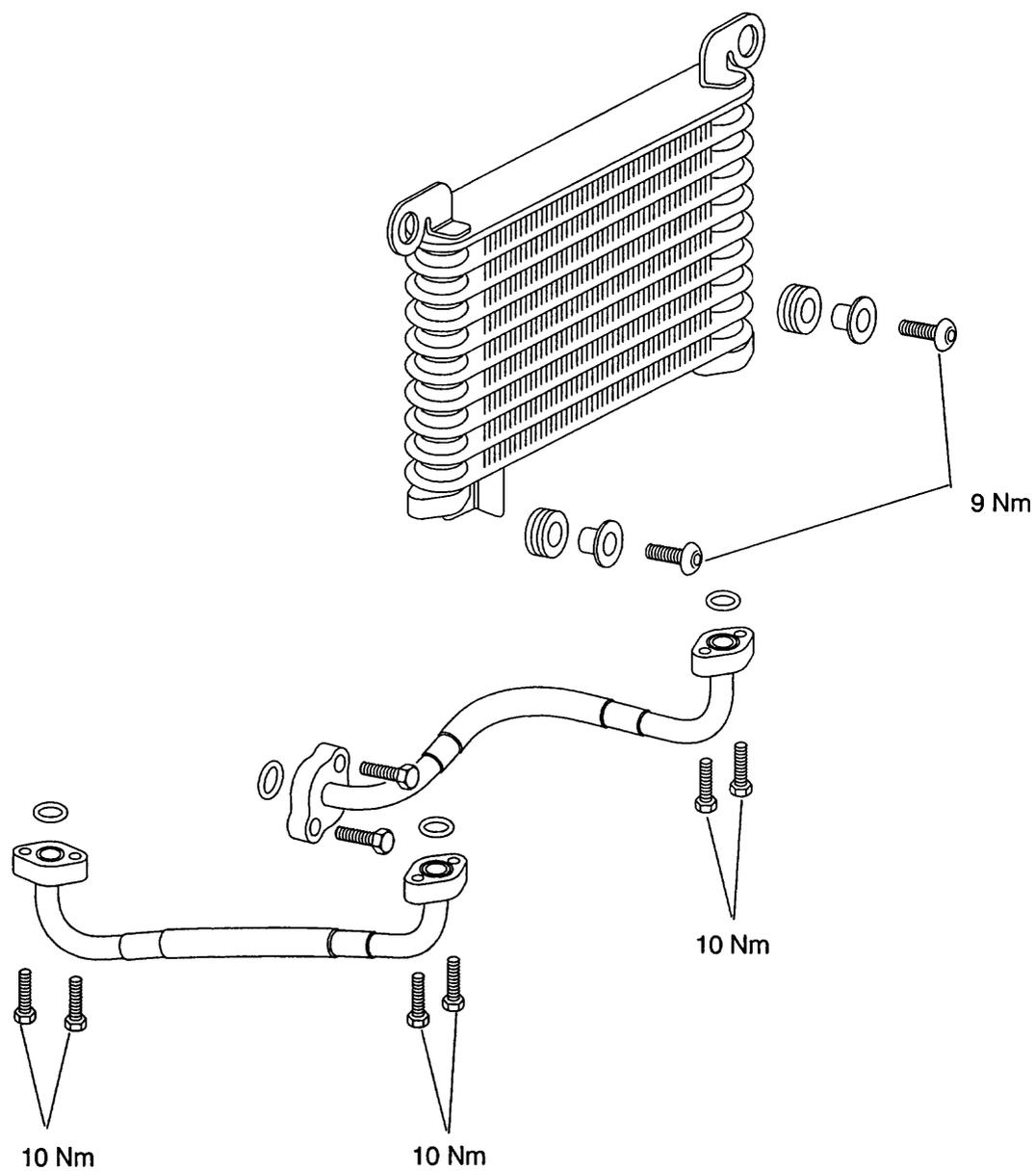
Exploded View - Speed Triple Oil Cooler
