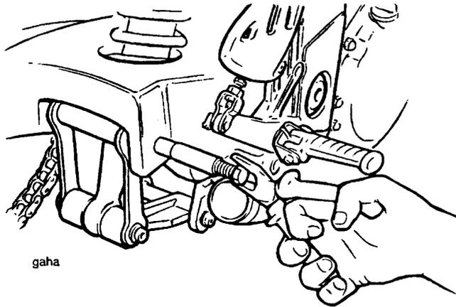
**Removing drop link spindle**
