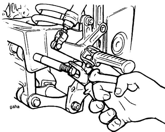
**Removing drop link spindle**
