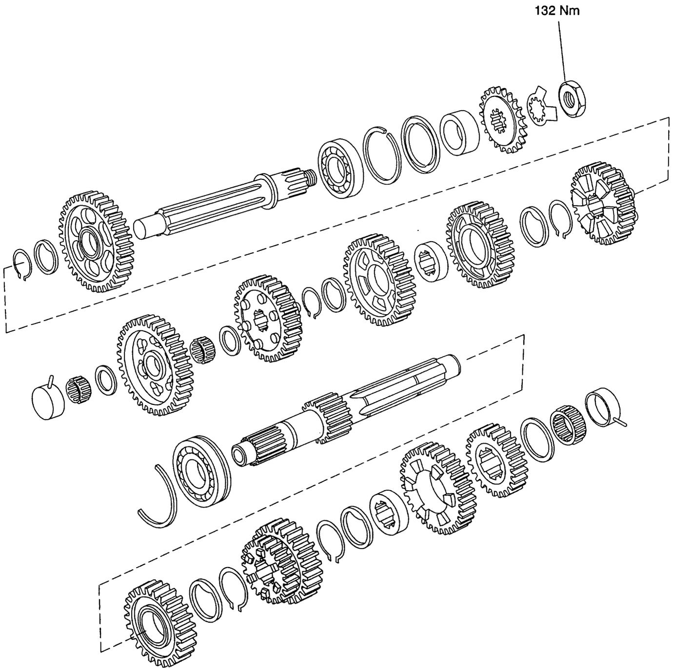
Exploded View, Sprag Clutch and Starter Gears
