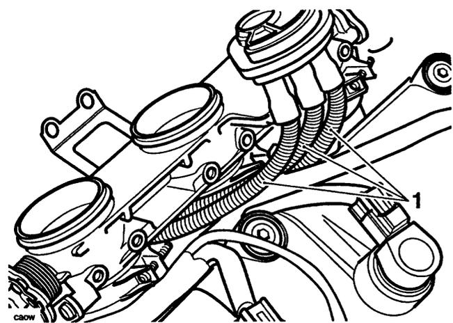
1. Air bleed hoses (disconnect at cylinder head)
