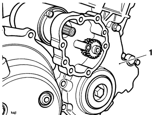
**1. Right hand crank cover (starter cover removed)**
