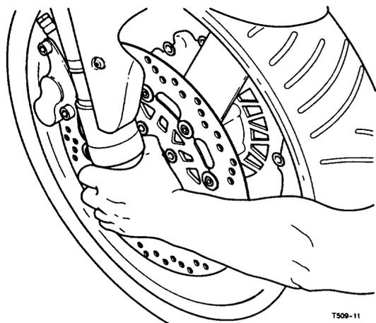
**Checking headstock bearing adjustment**
