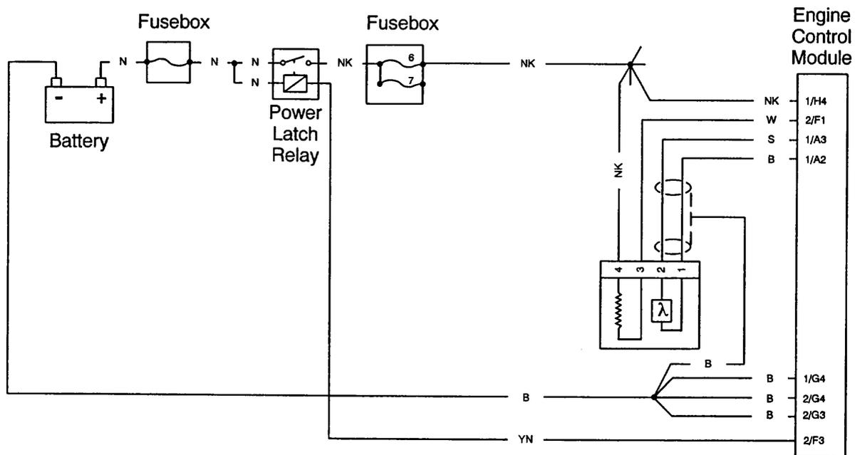
**SECONDARY AIR INJECTION SOLENOID**
