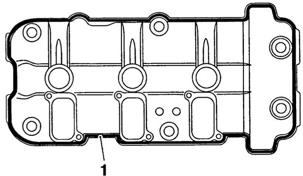
1. Cam cover seal groove
