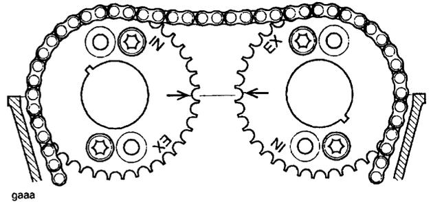
**Camshaft to Cylinder Head Alignment Marks**
