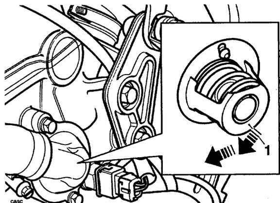
1. Thermostat (face shown inserted into the head)
