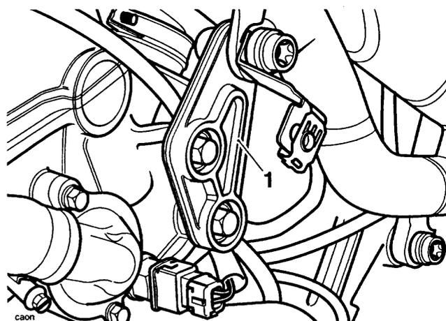
**1. Frame to Cylinder Head Mounting Bracket**
