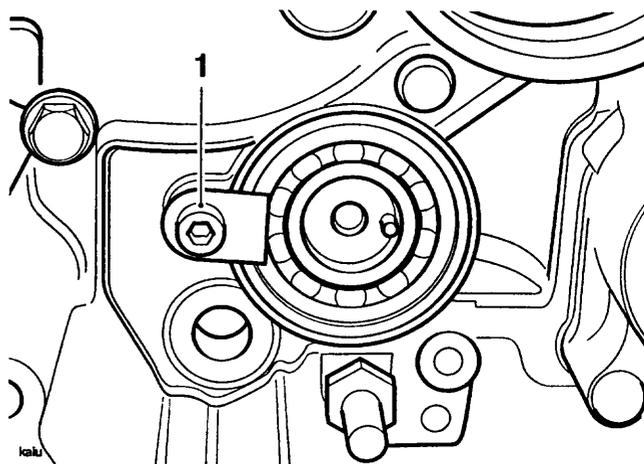
**1. Bearing Retaining Bolt**
