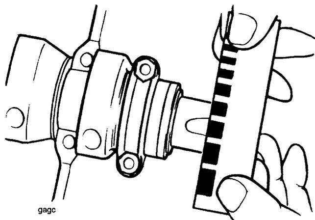
Checking crankpin clearance using *Plastigage*
