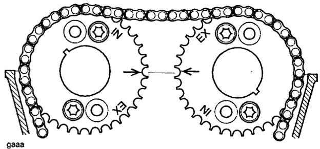
**Camshaft to Cylinder Head Alignment Marks**
