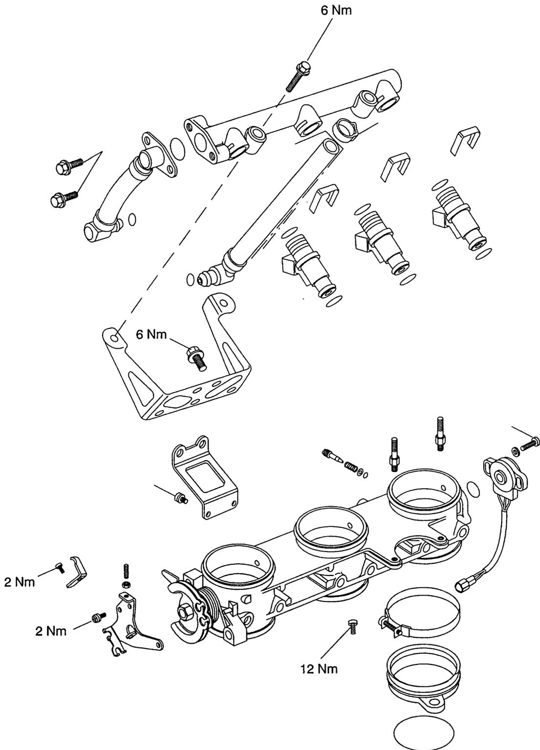
**Exploded View - Secondary Air Injection Valves and Controls**
