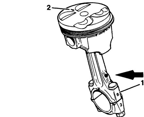
**1. Connecting Rod with Oil Hole Arrowed**
