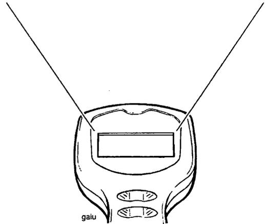
Start the engine. 'CURRENT DATA' includes the information shown in the table below which can be accessed by scrolling, using the 'Up' and 'Down' keys. At the end of each line of text, the actual reading at that instant is provided to assist diagnosis e.g. **ENGINE TEMP 95C**.
