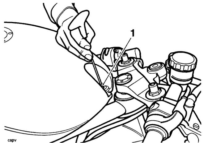
1. Fuel tank to frame bolt (front)
