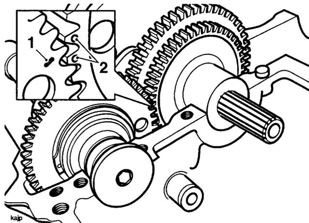
1. Balancer backlash and drive gear markings
