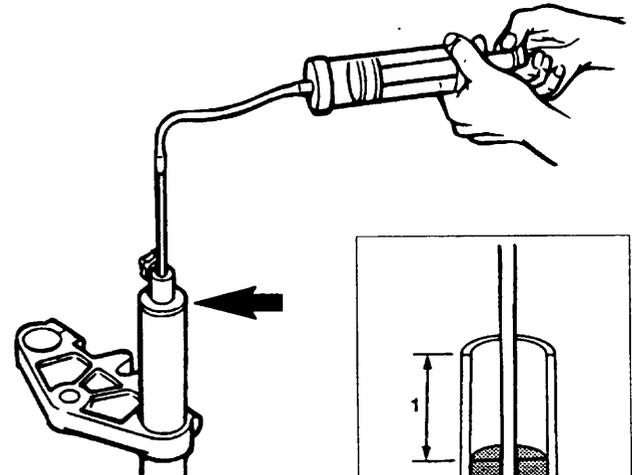
Plate arrowed must be level with fork slider
