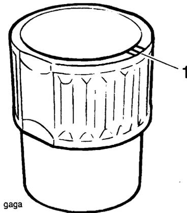
**CAUTION:** Some cylinder liners are made of aluminium alloy and therefore can be easily damaged. Handle these cylinder liners with care, ensuring the cylinder bore is not scratched.
