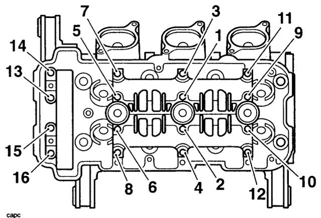
**Cam-cap and ladder bolt tightening sequence**
