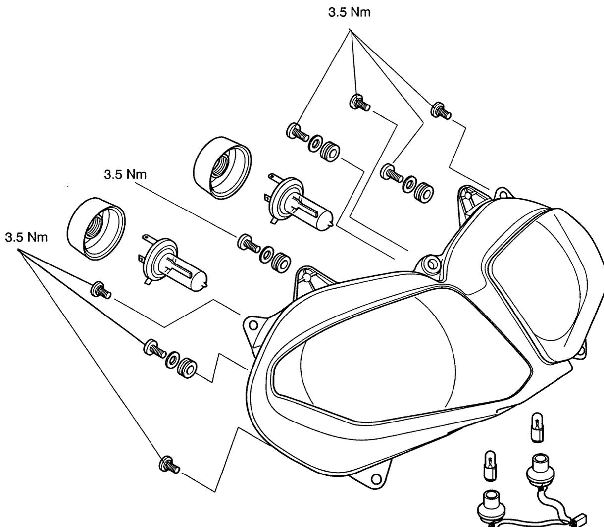
**Exploded View - Speed Triple Headlight**
