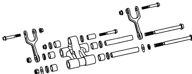
**Exploded view - drop/drag link components**
