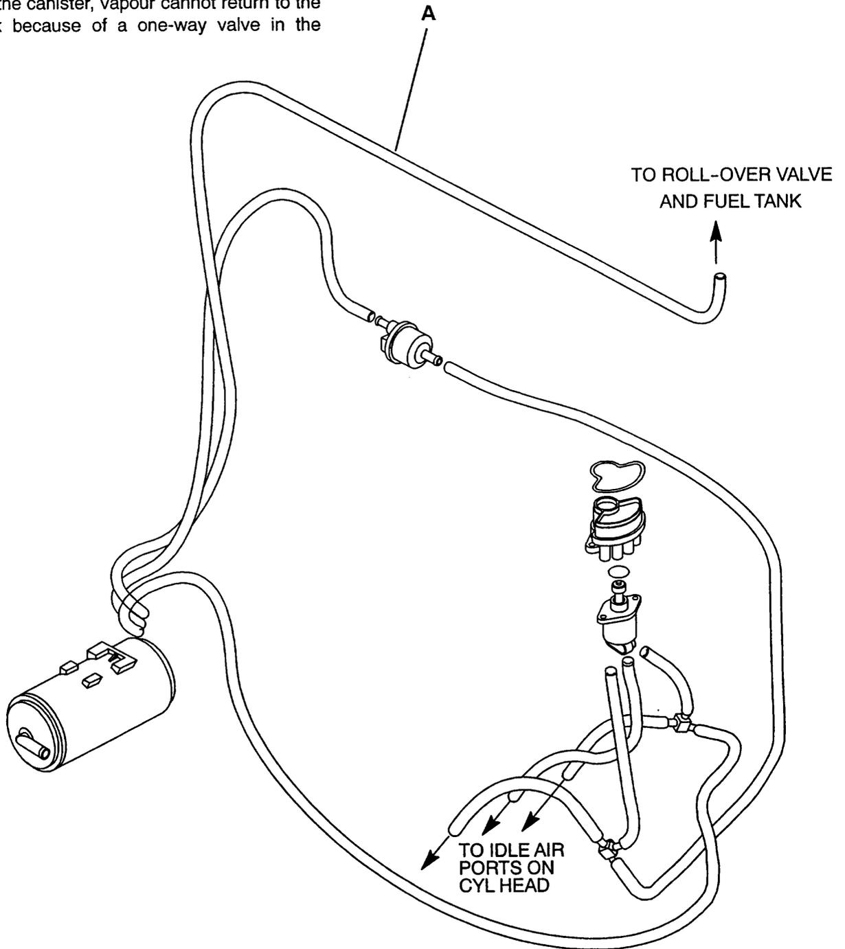
**Evaporative Control System - Engine Running**
