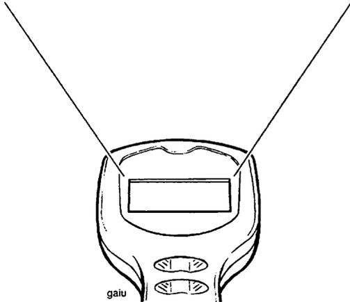
The second line – ‘DTC COUNT’, shows the number of DTC’s stored in the ECM memory.
