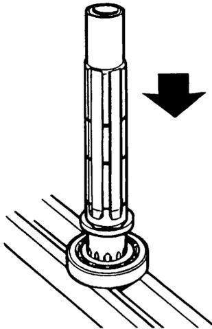
2. Fit the retaining ring (23) to the shaft. Lubricate and fit a new oil seal (22).
