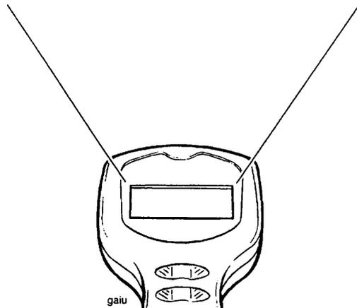
To clear the DTC's, press the Validation key '\*'. 'STORED DTCs' will be displayed (see operation 13).
