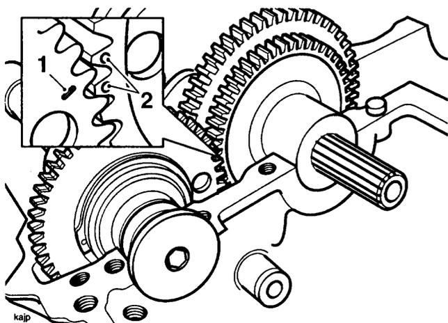
1. Balancer backlash and drive gear markings
