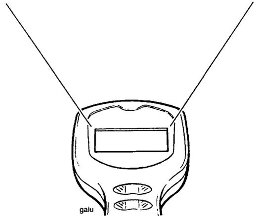
If the test at operation 22 is unsatisfactory, a DTC will be displayed on line 3 of this display (except fuel pump tests).
