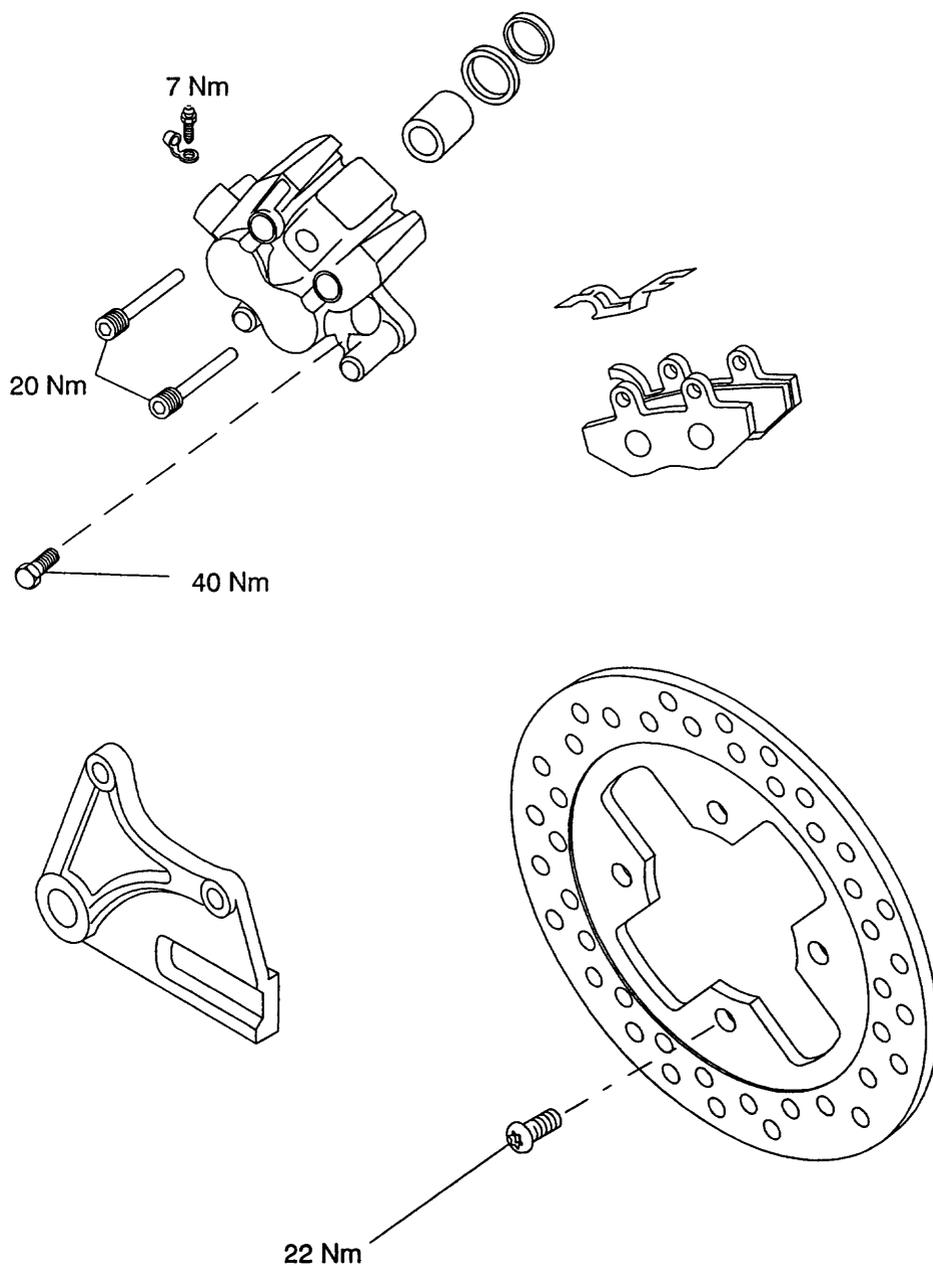
**Exploded View - Rear Brake Caliper (single sided swinging arm versions)**
