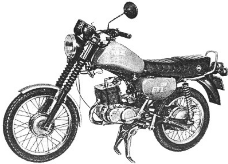
Fig. 2. ETZ 125/150 with drum brake in standard design
